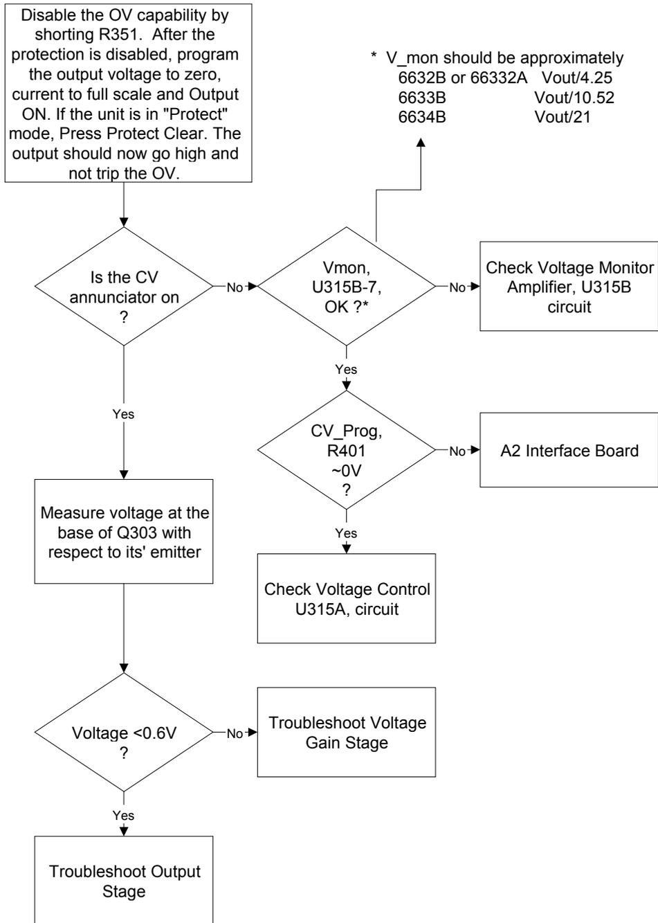
Figure 3-1 Sheet 12. High Output Voltage
