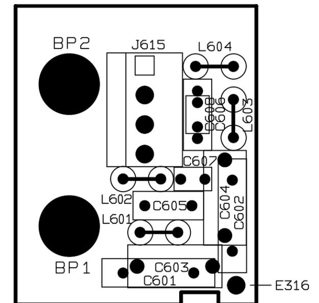
Figure 6-2. A4 and A6 Board Component Locations
