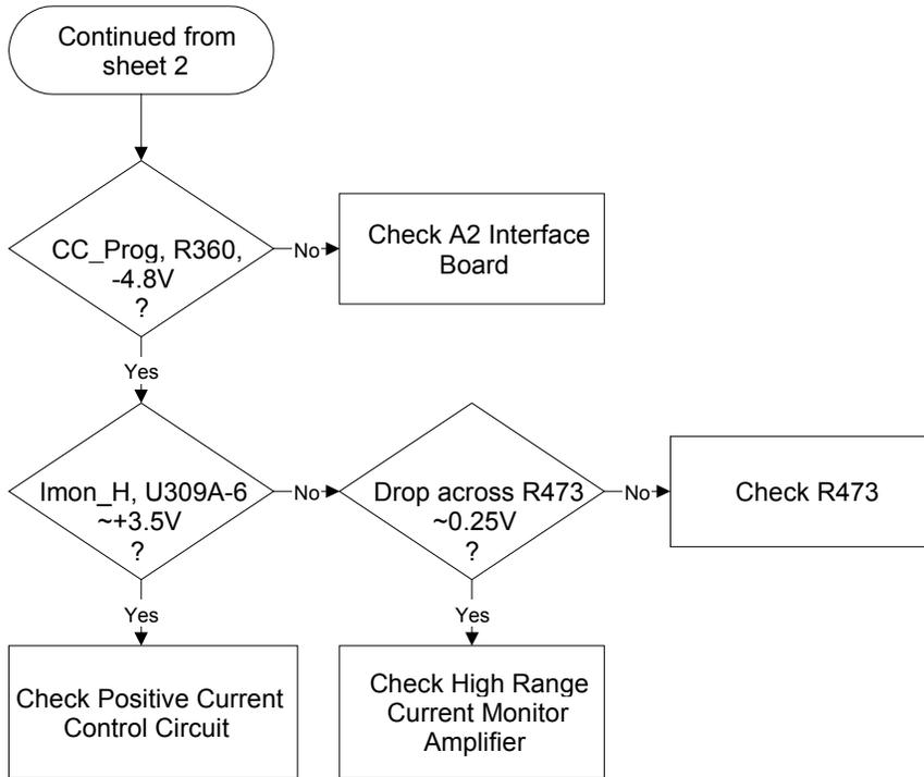
Figure 3-1 Sheet 10. No Current Limit
