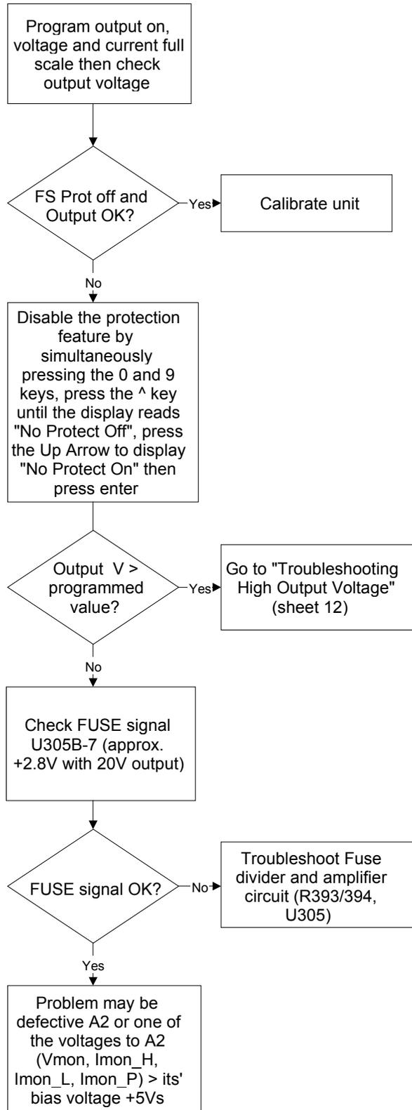
Figure 3-1 Sheet 6. FS Indicated but Fuse OK
