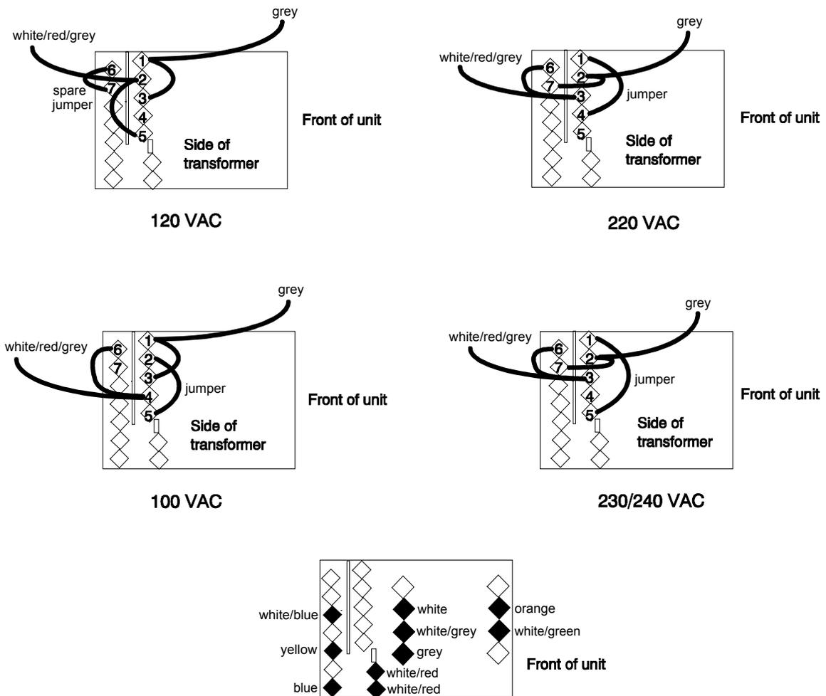
**Figure 3-3. Transformer Wiring**
