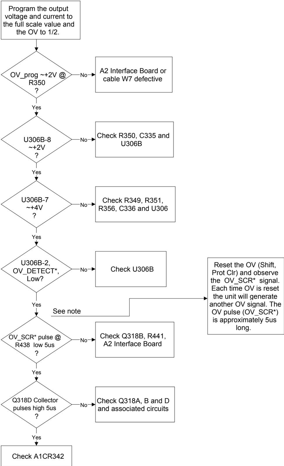
Figure 3-1 Sheet 11. Unit Does Not OV
