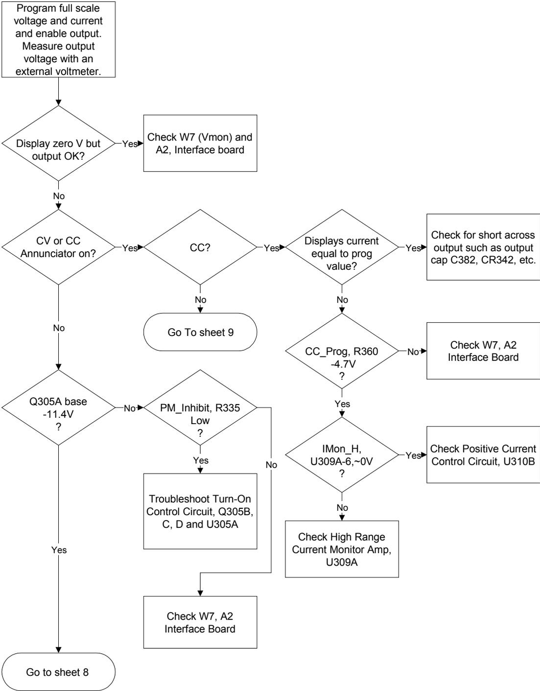
Figure 3-1 Sheet 7. No Output Voltage
