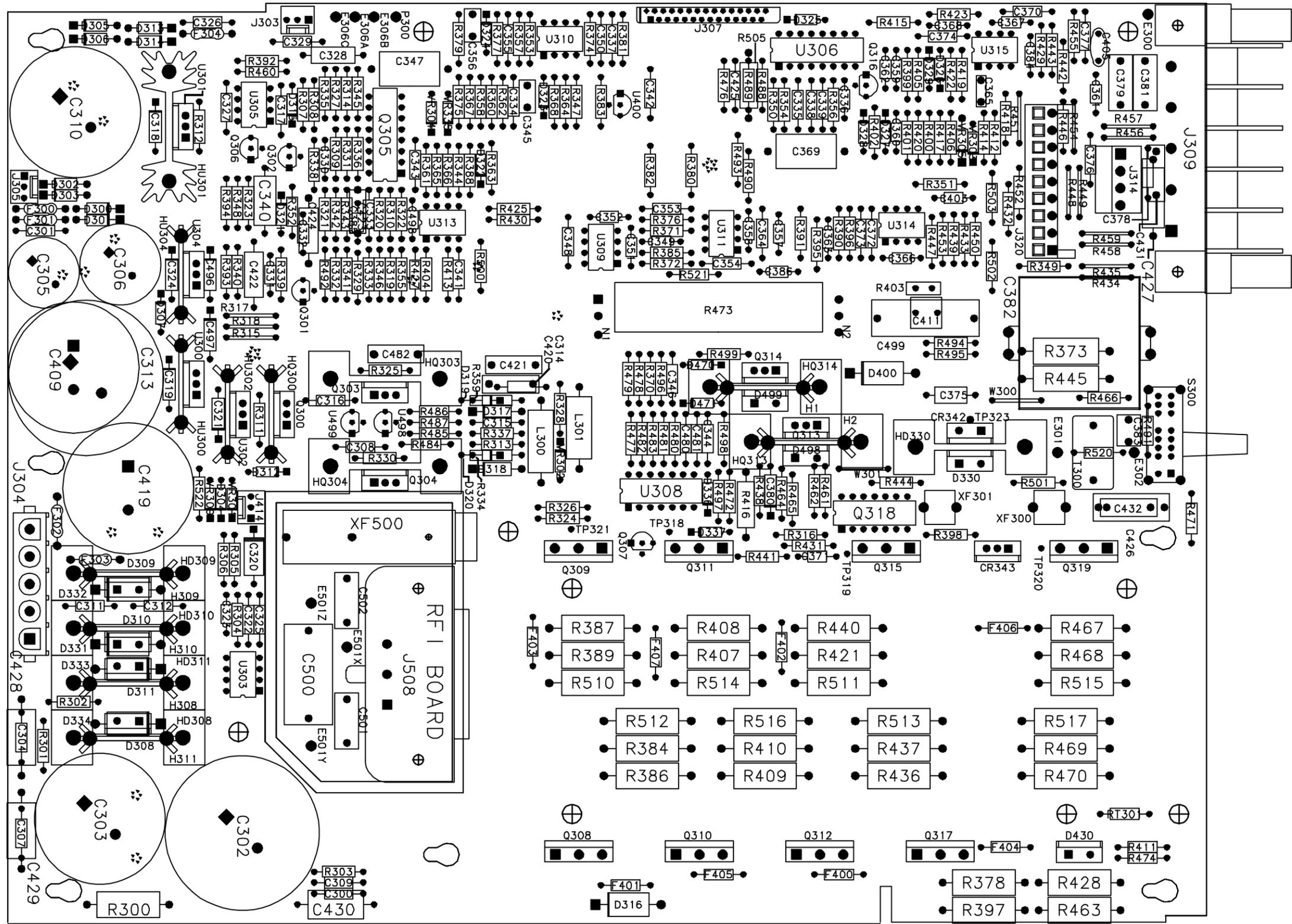
Figure 6-1. A1 Board Component Locations
