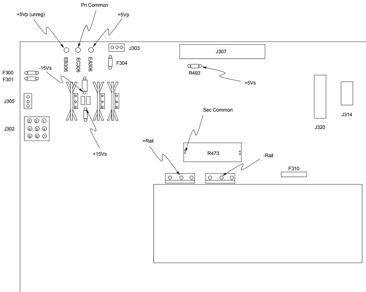
Figure 6-1. A1 Board Component and Test Point Locations
