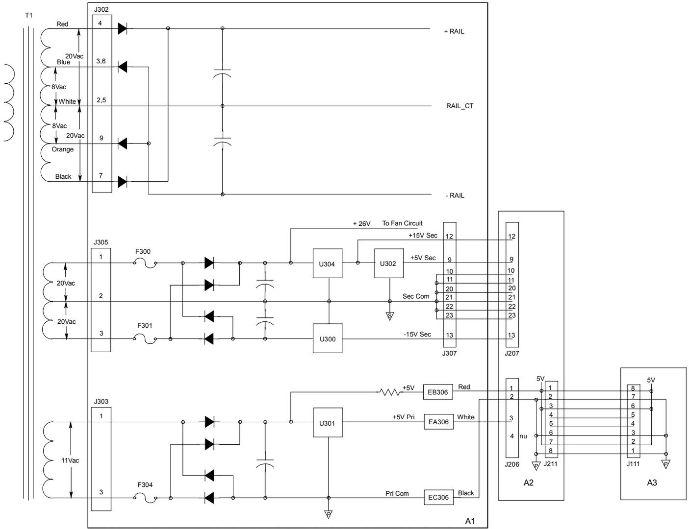
**Figure 6-4. Rail and Bias Circuits**
