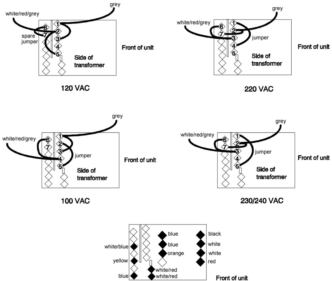
Figure 3-3. Transformer Wiring
