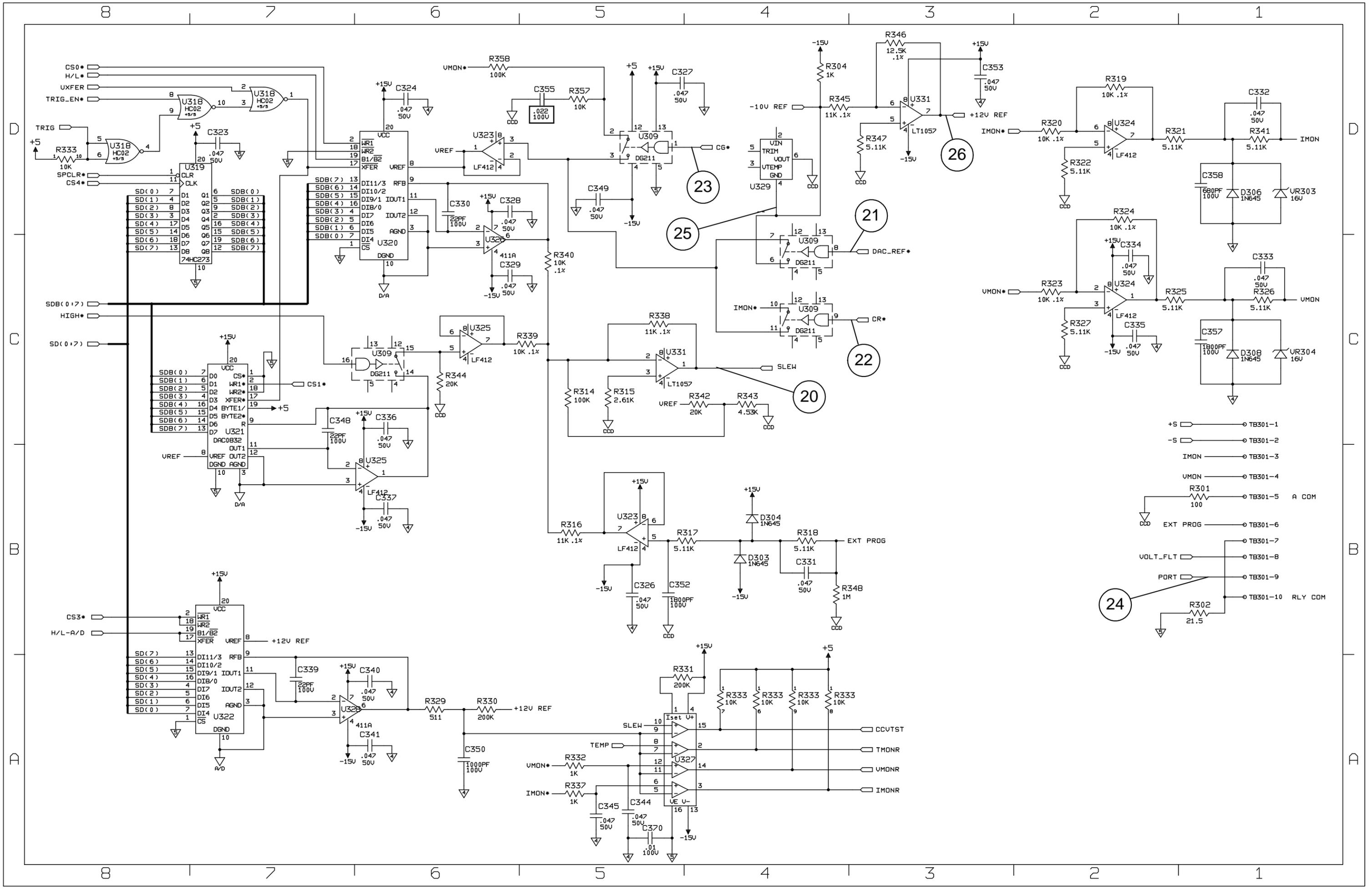
Figure 6-1. 6060B/6063B Electronic Load Schematic (Sheet 4 of 6)
