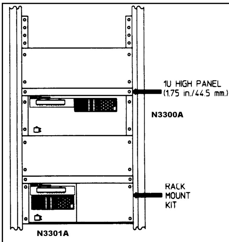
Figure 3-4. Rack Installation
