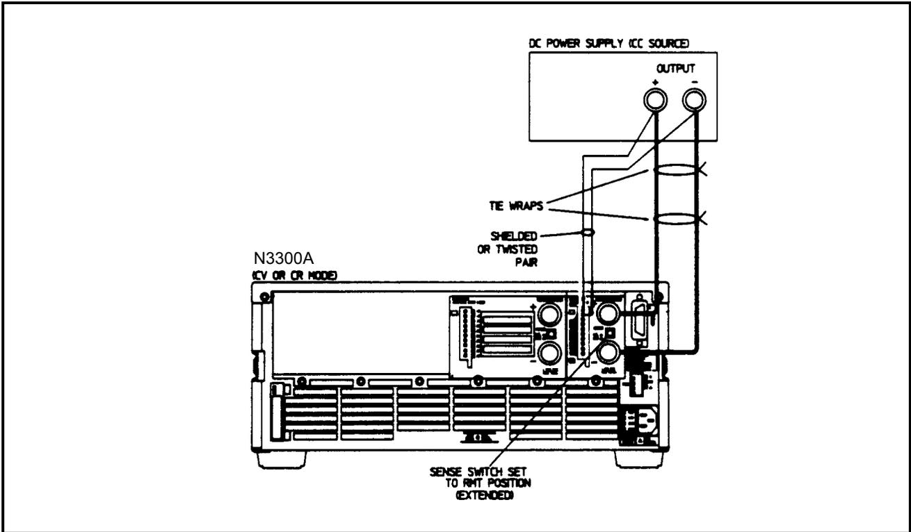
Figure 3-11. Remote Sensing
