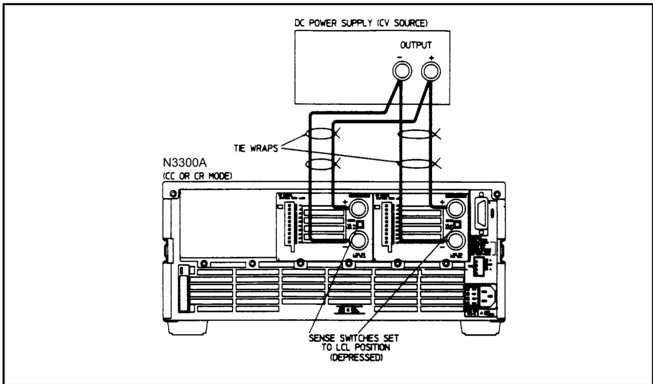
Figure 3-12. Parallel Operation
