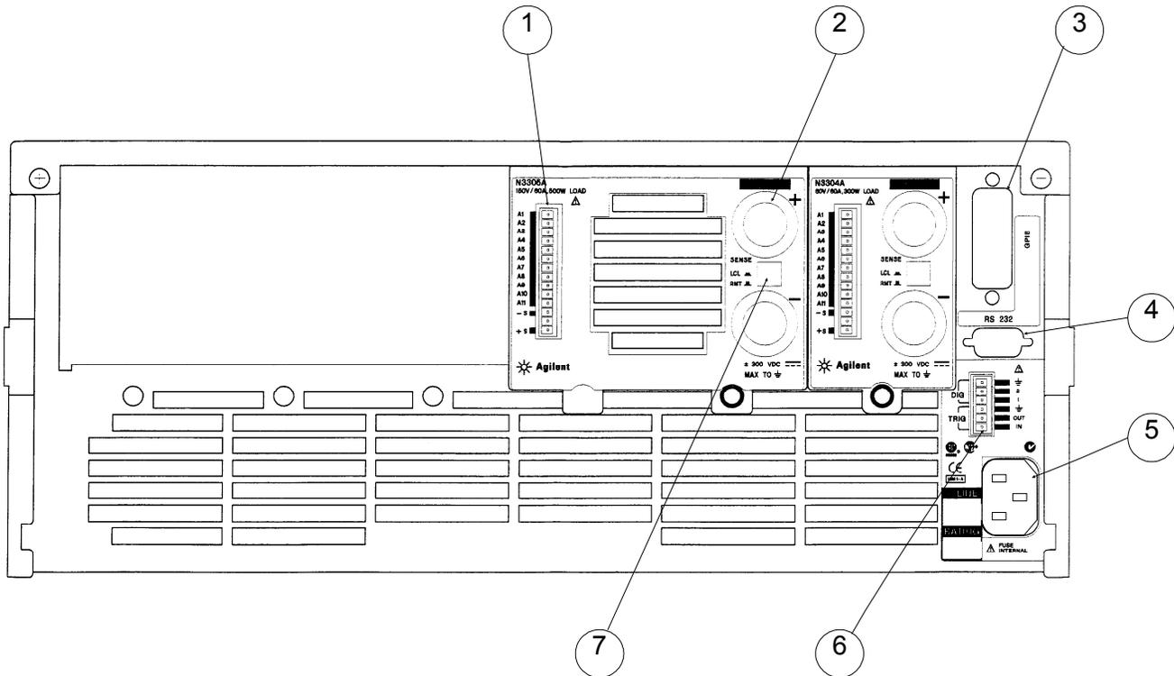
⑤ 3-pin IEC 320 ac input connector. (power cord requires ground conductor)
