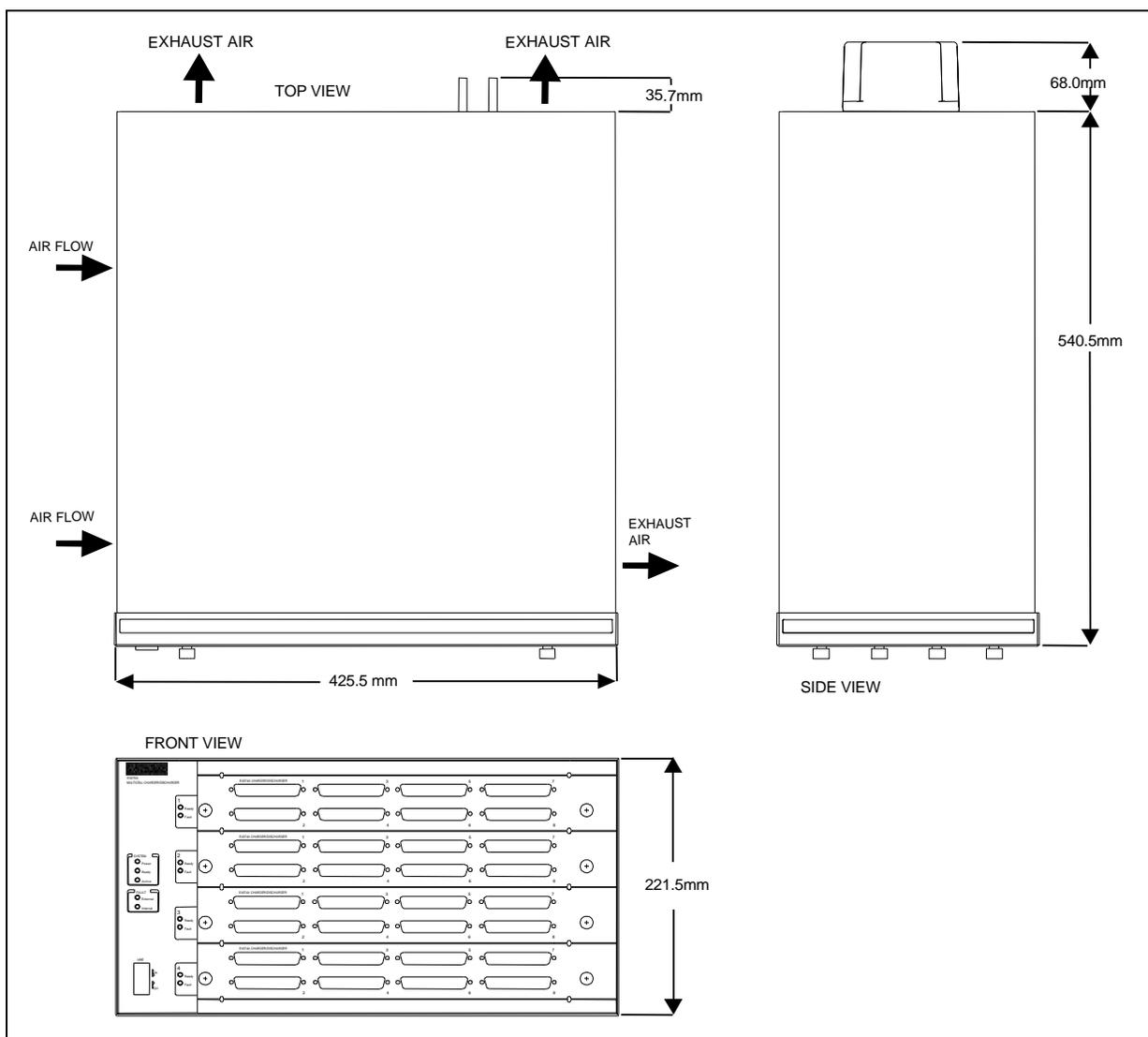
Figure C-1. Agilent M CCD Simplified Outline Diagram
