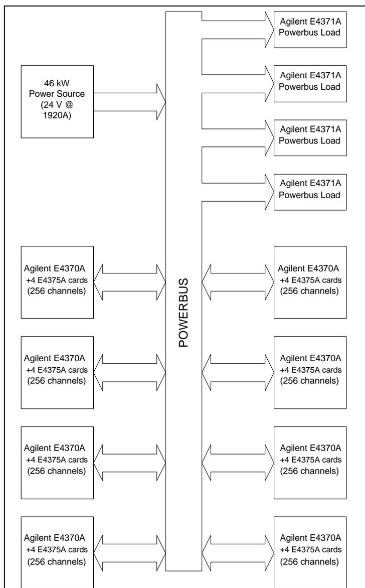
**Figure 1-6. System Diagram Using Agilent E4375A Cards**
