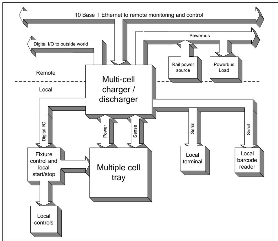
Figure 1-1. Block Diagram of Agilent MCCD System
