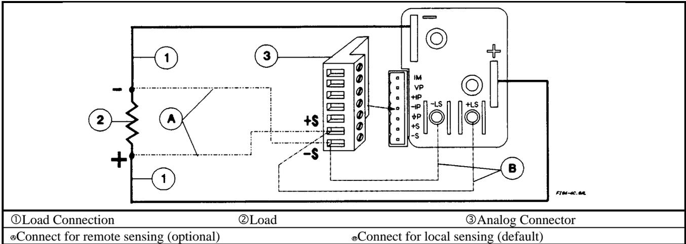
**Figure 4-5. Single Load Connection (Remote Sensing Optional)**
