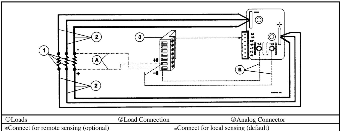
**Figure 4-6. Multiple Load Connection (Remote Sensing Optional)**
