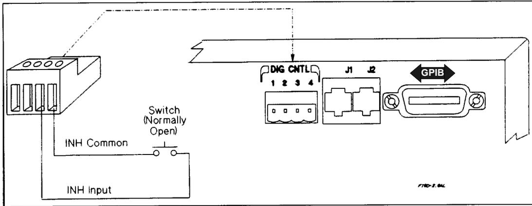
**Figure F-2. Example of Inhibit Input**
