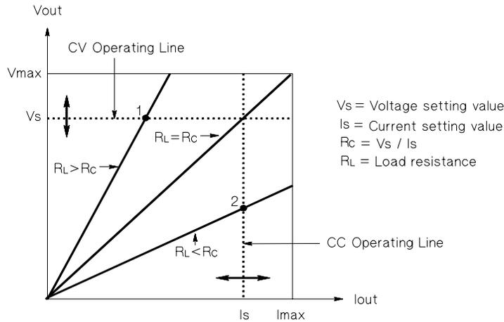
Figure 7-5. Output Characteristics
