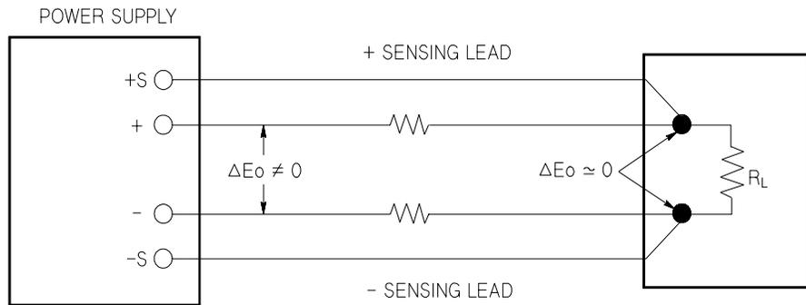
**Figure 7-7. Regulated Power Supply with Remote Sensing**
