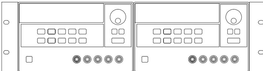
**To rack mount two instruments of the same depth side-by-side, order link kit 5061-9694 and flange kit 5063-9214.**
