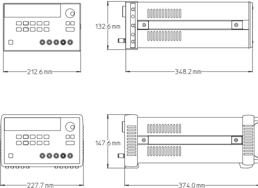
**Figure 8-1. Dimensions of Agilent E3632A Power Supply**
