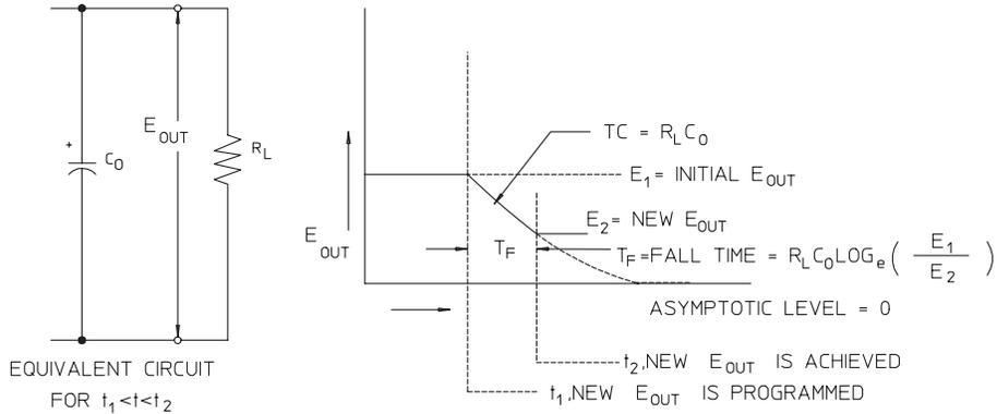
**Figure 7-9. Speed of Response - Programming Down**
