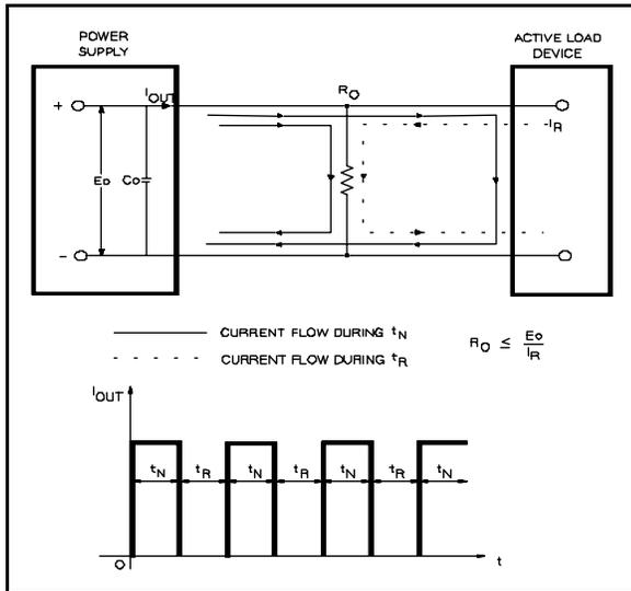
Figure 3. Reverse Current Loading Solution
