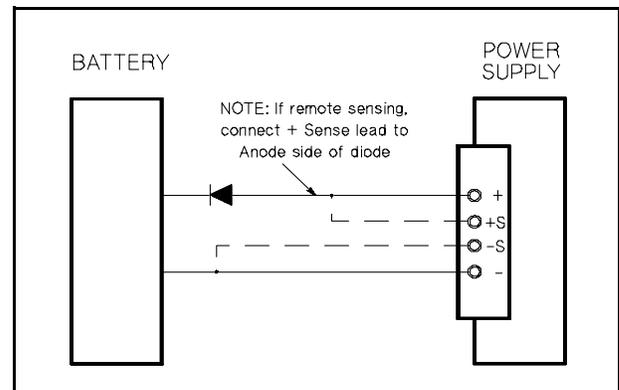
Figure 17. Recommended Protection Circuit for Battery Charging
