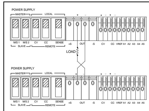
**Figure 11. Normal Series Operation of Two Supplies**
