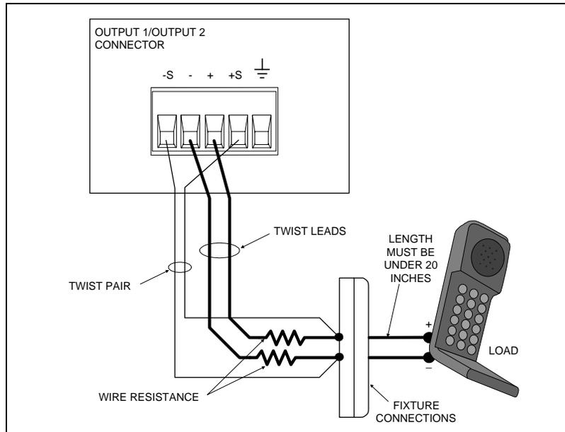
Figure 3-4. Remote Sense Connections with Test Fixture
