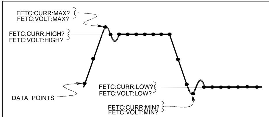
Figure 7-3. Measurement Commands Used to Return Pulse Data
