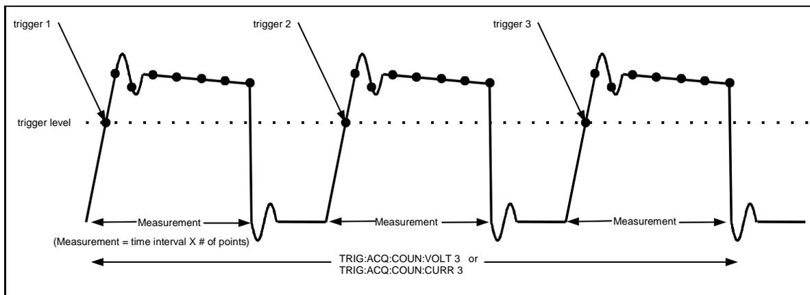
**Figure 7-6. Multiple Measurements**
