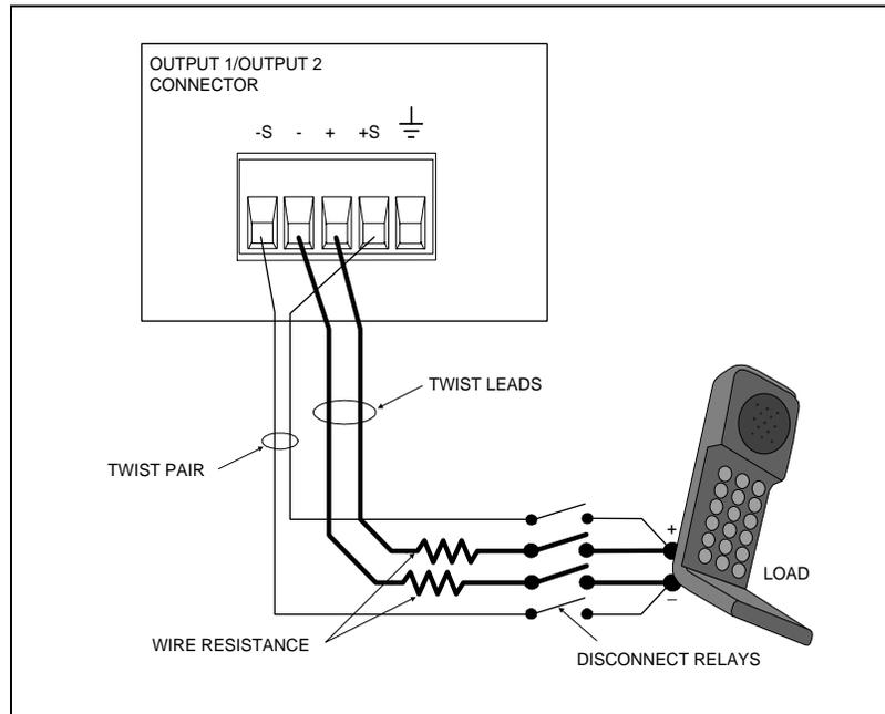
**Figure 3-3. Remote Sense Connections with External Relays**
