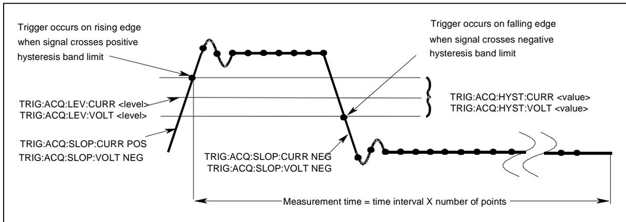
**Figure 7-5. Commands Used to Control Measurement Triggers**
