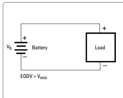
Figure 5. Single Battery Test Configuration
