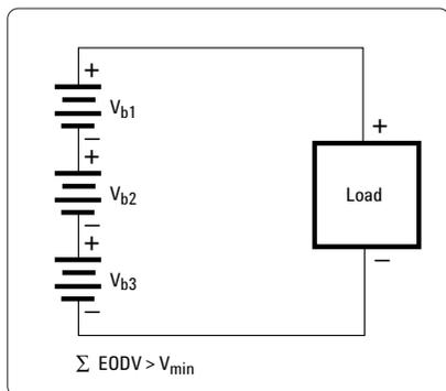
Figure 6. Batteries in Series
