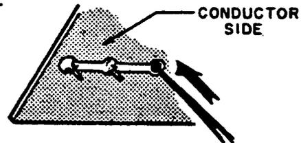
3. Bend clean tinned lead on new part and carefully insert through eyelets or holes in board.
