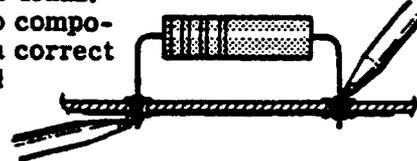
In the event that either the circuit board has been damaged or the conventional method is impractical, use method shown below. This is especially applicable for circuit boards without eyelets.
