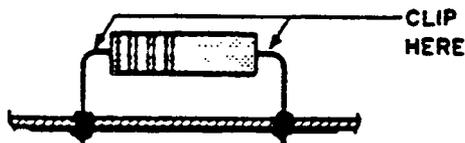
2. Bend protruding leads upward. Bend lead of new component
