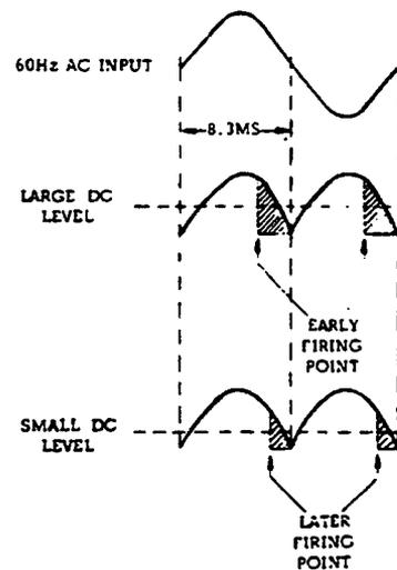
Figure 4-3. SCR Phase Control of DC Input Level
