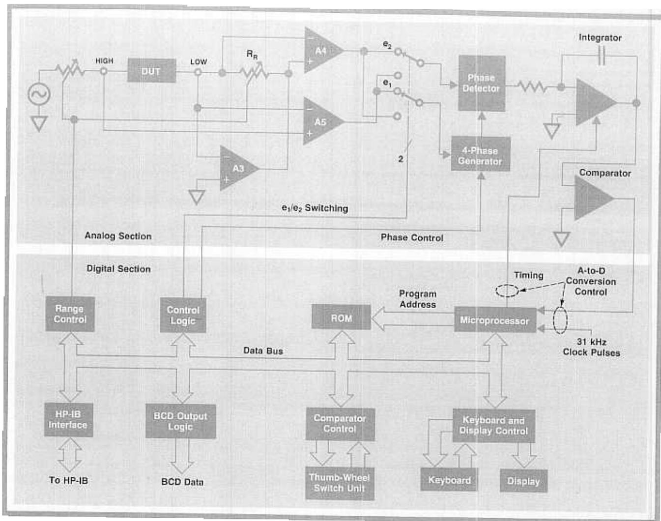
**Fig. 4.** Simplified block diagram of the Model 4262A LCR Meter. Under control of the microprocessor, the circuits find the ratios of the real and imaginary parts of the voltage across the DUT with respect to the current (or vice versa), from which the device parameters can be derived.
