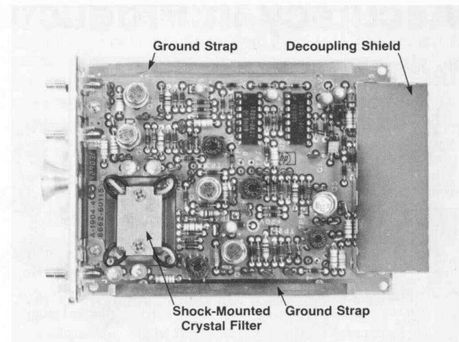
Fig. 4. Spring ground strap provides additional grounding for sensitive or critical boards. A beryllium-copper shield decouples the RF and dc circuits.
