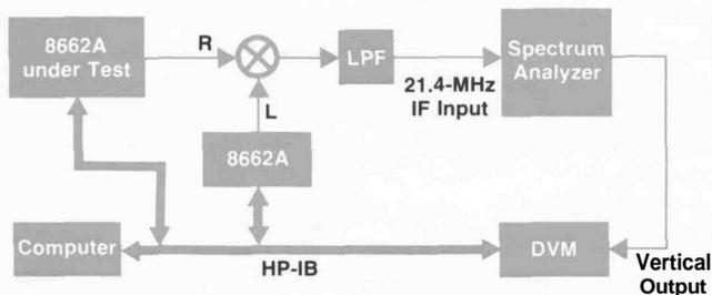
**Fig. 14.** System to measure the spurious output of the 8662A uses a 21.4-MHz spectrum analyzer IF section and a second 8662A as a swept local oscillator. The second 8662A improves the analyzer's phase noise.
