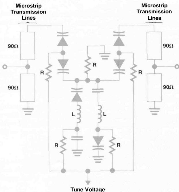
Fig. 7. Voltage-tunable bandpass filter consists of two resonators coupled by a shunt capacitance. The tuning voltage changes the capacitance of the diodes.
