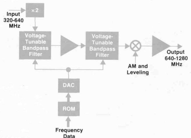
Fig. 4. Frequency doubler system provides the top octave of the 8662A frequency range.
