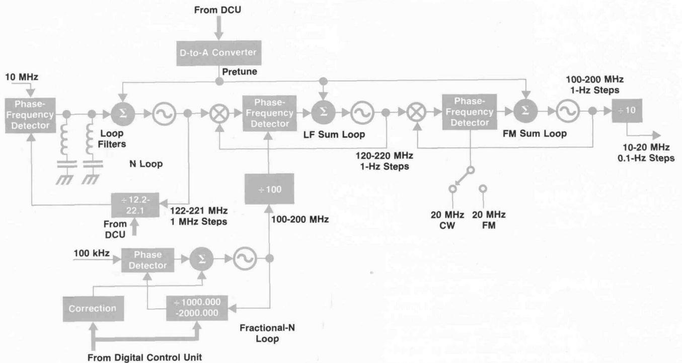
Fig. 9. 8662A low-frequency section has four phase-locked loops and produces a signal from 10 to 20 MHz in 0.1-Hz steps.
