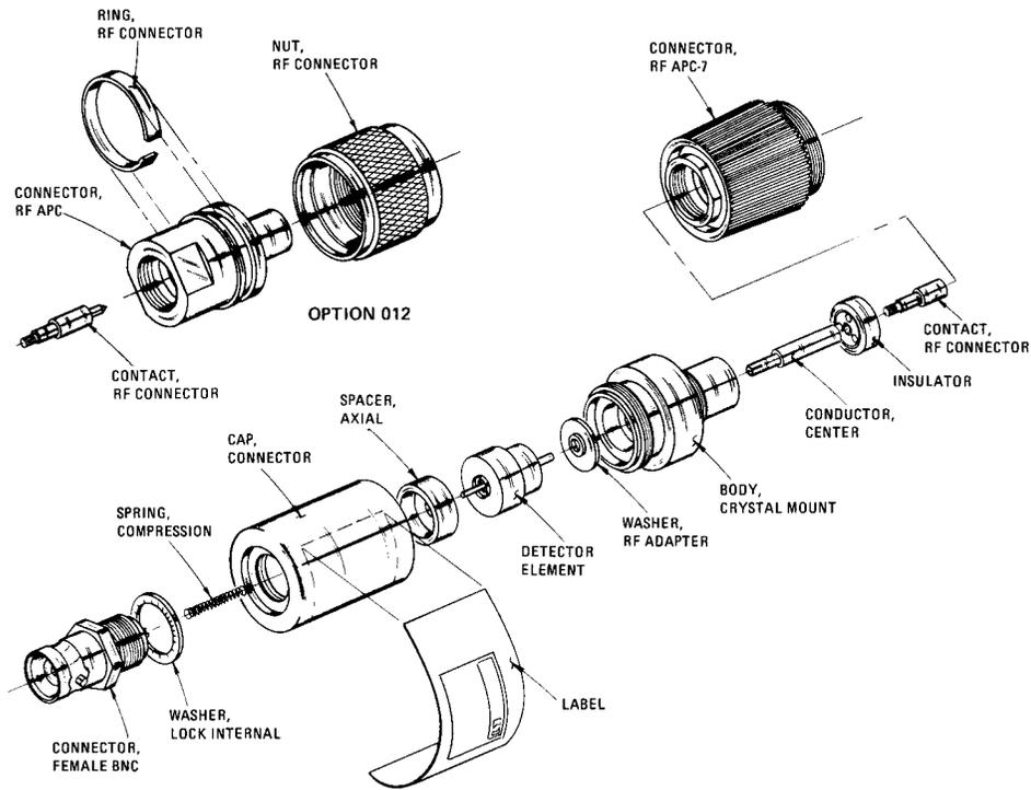
Figure 4 8470B and 8470B Option 012 Detector Assemblies
