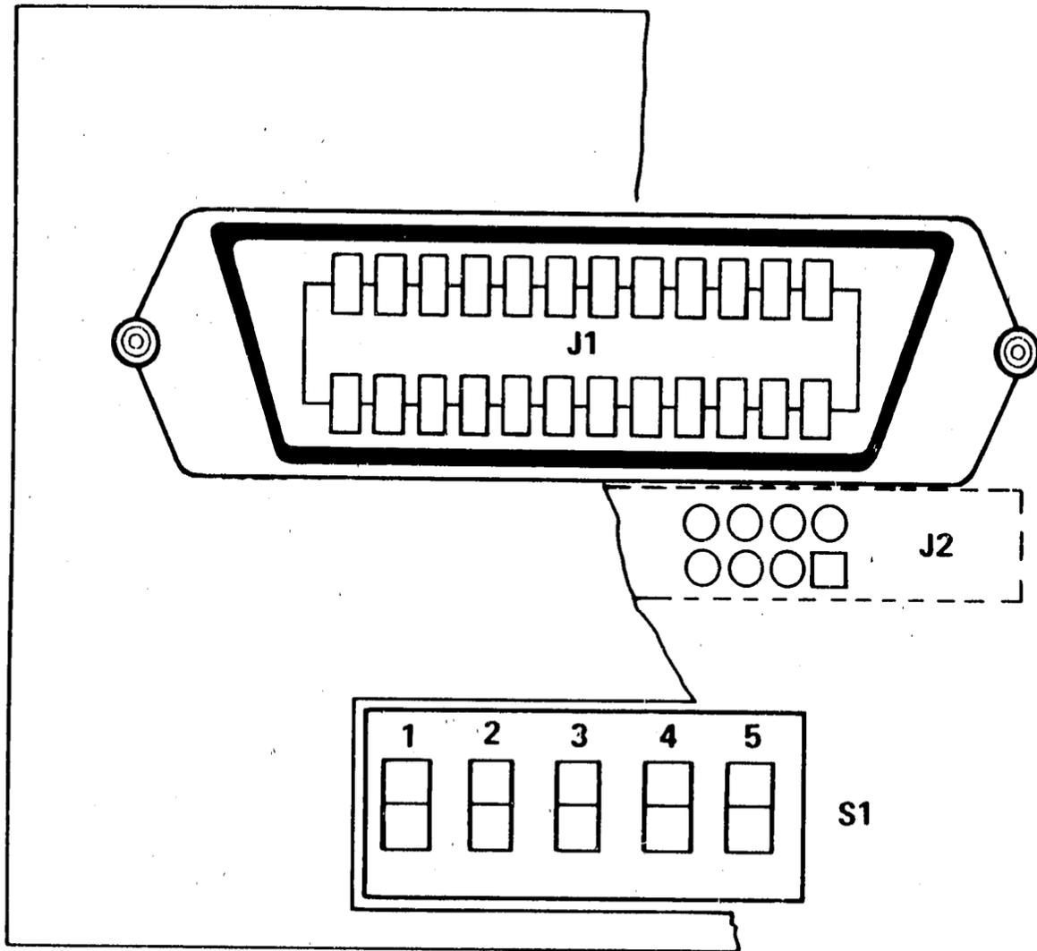
Figure 8-20. HP-IB (A3 Assembly) Connector Component Locations
