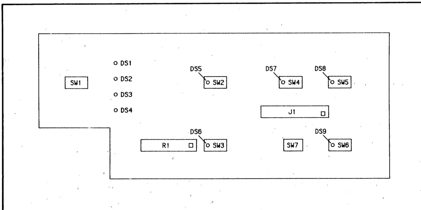
Figure 8-25. Keyboard and Annunciators (A1 Assembly) Component Locations
