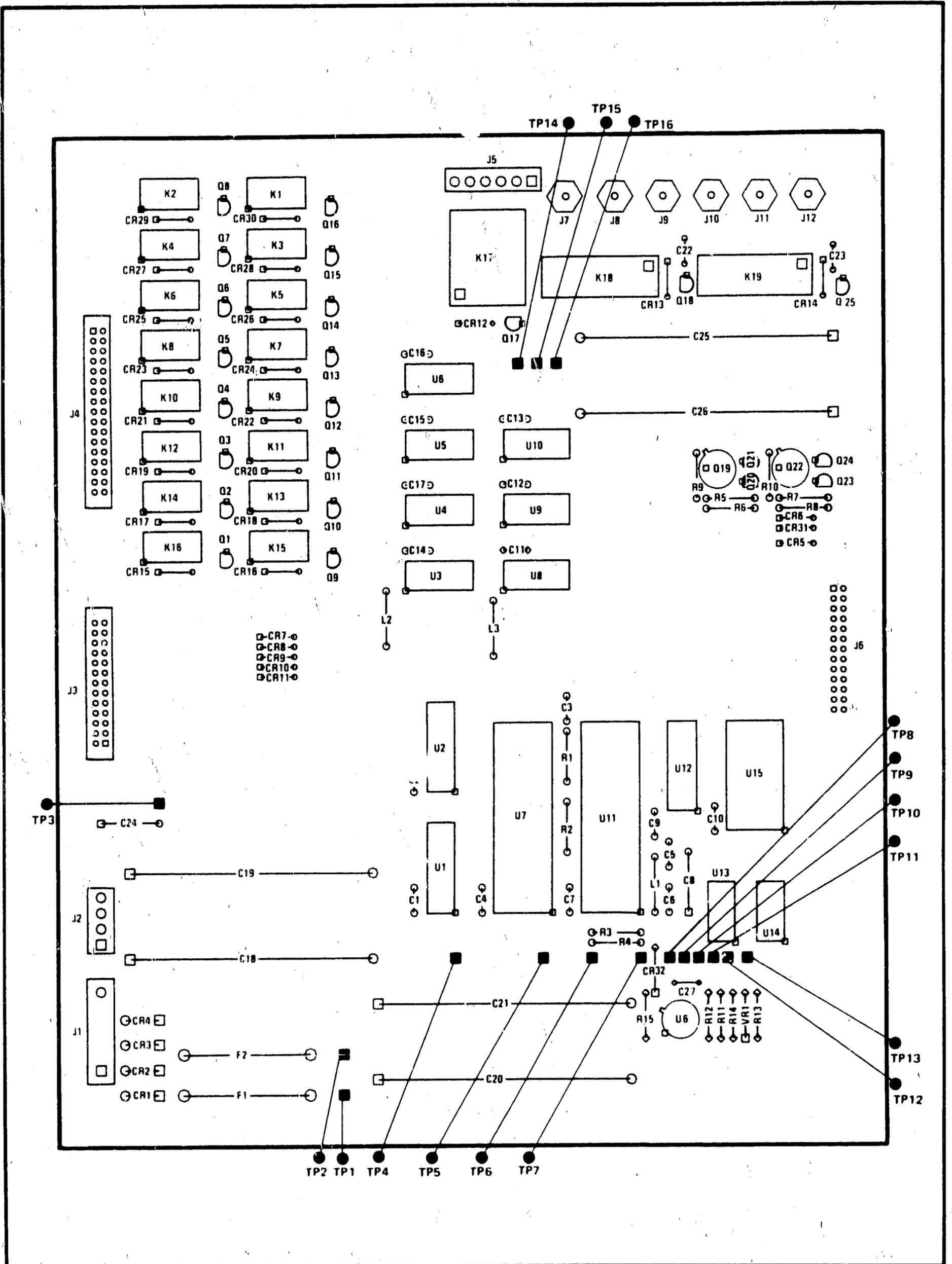
Figure 8-23. Interface Control Board (A2 Assembly) Component Locations
