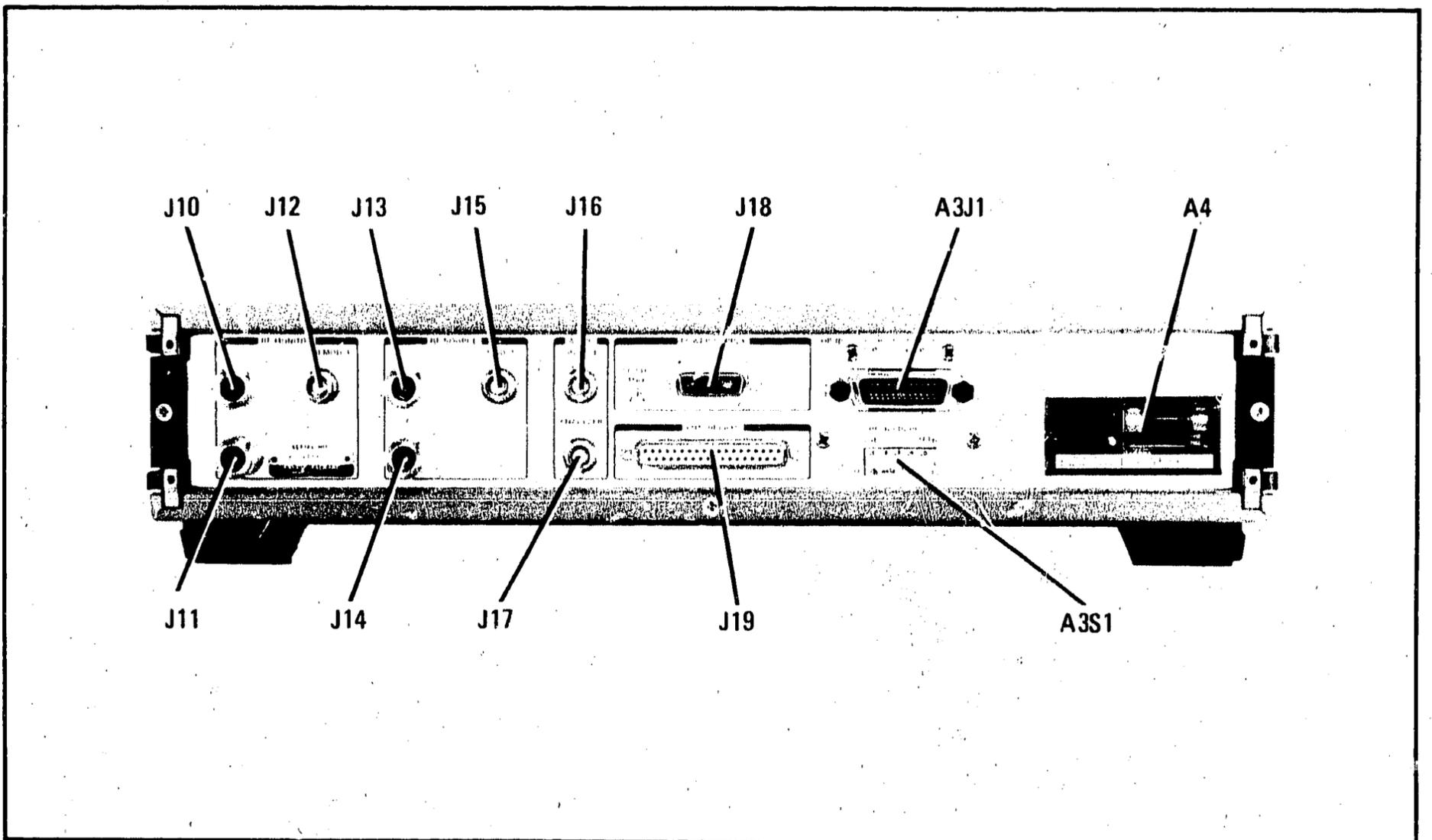
Figure 6-4. Chassis and Mechanical Parts Identification—Rear Panel
