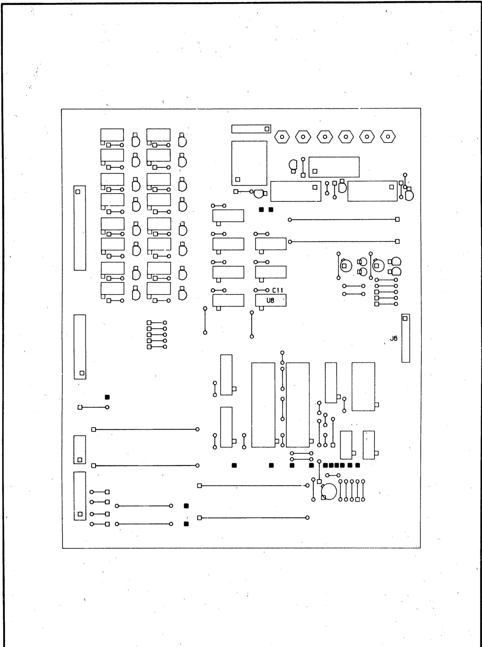
Figure 8-26. Interface Control Board (A2 Assembly) Component Locations
