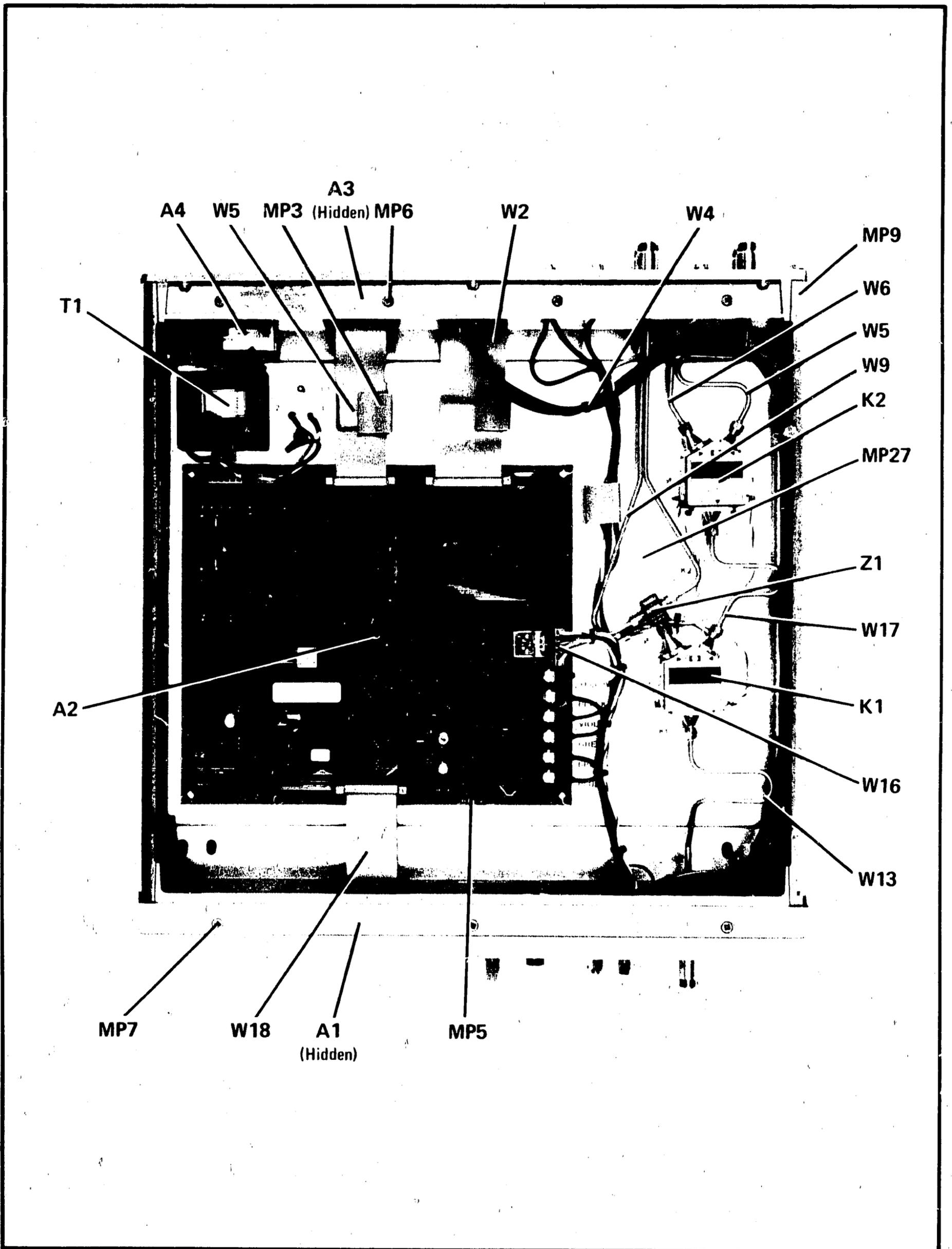
Figure 6-1. Top Chassis Parts, Mechanical Parts, Cables, and Assembly Identification
