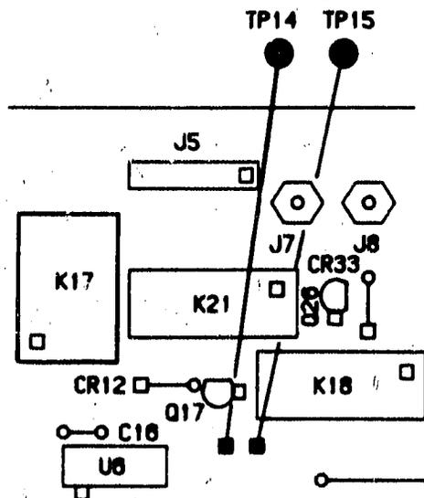
P/O Figure 8-23. Interface Control Board (A2 Assembly) Component Locations (P/O CHANGE 4).
