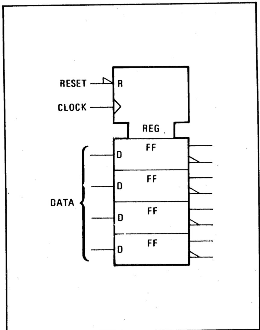
Figure 8-11. Quad D-Type Latch (Combined)
