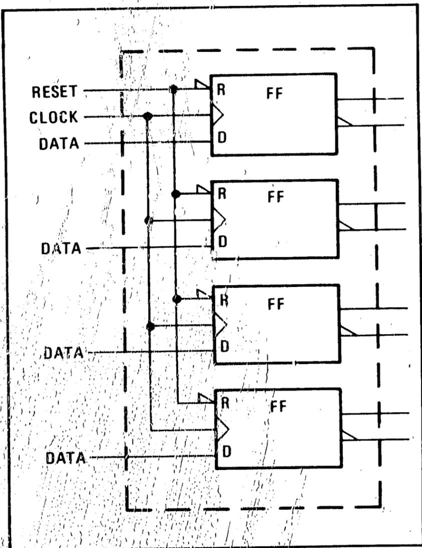
Figure 8-10. Quad D-Type Latch (Individual)
