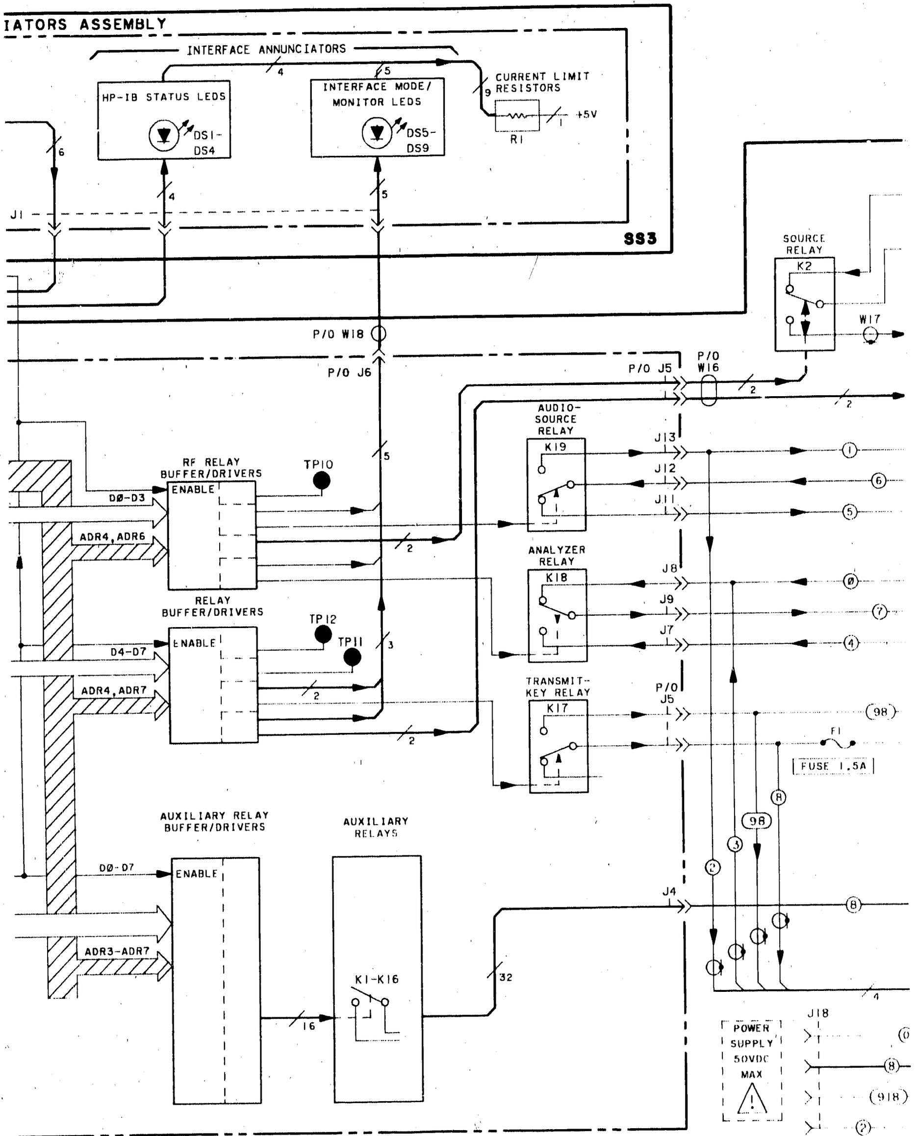
P/O Figure 8-24. Service Sheet 2, Relay Control Driver and Relays
