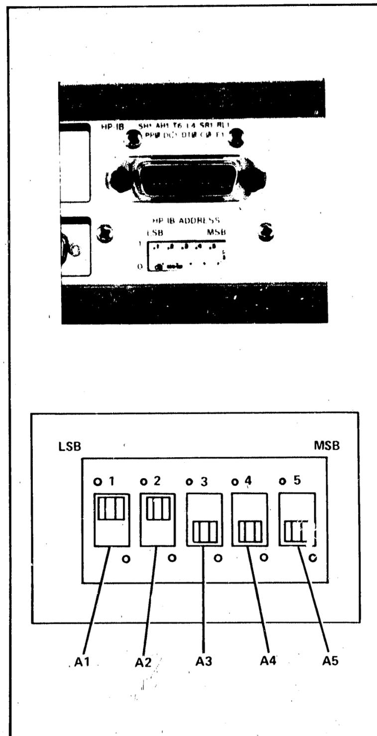
Figure 2-2. HP-IB Address Switch Location and Settings
