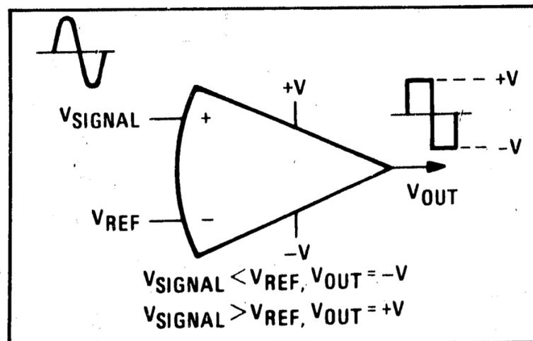
Figure 8-16. Non-inverting Comparator
