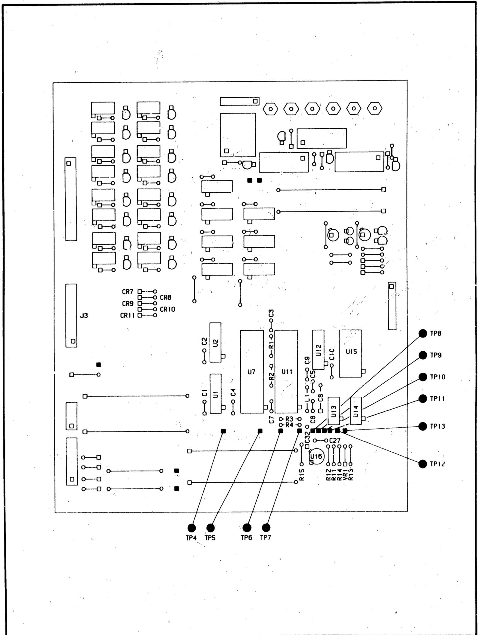
Figure 8-21. Interface Control Board (A2 Assembly) Component Locations
