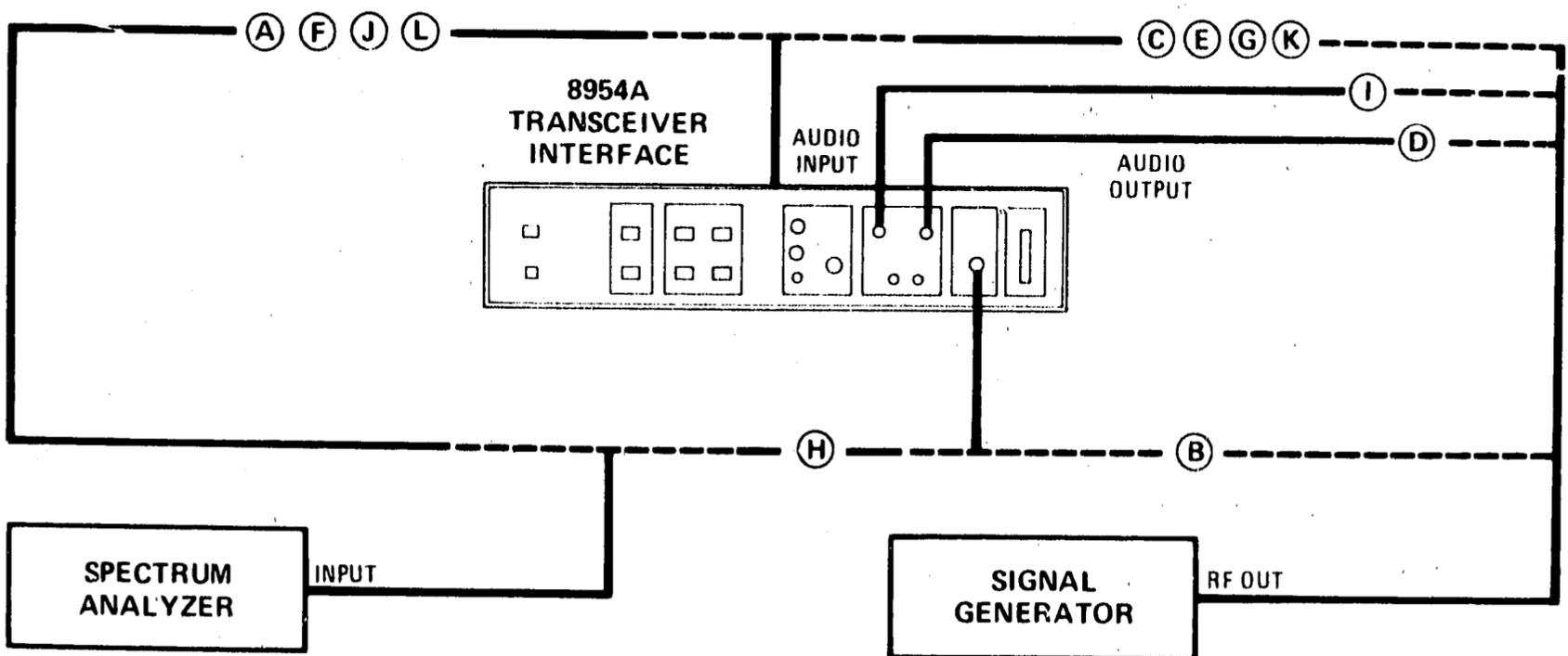
*Figure 3-3. Test Configuration for Basic Function Checks*
