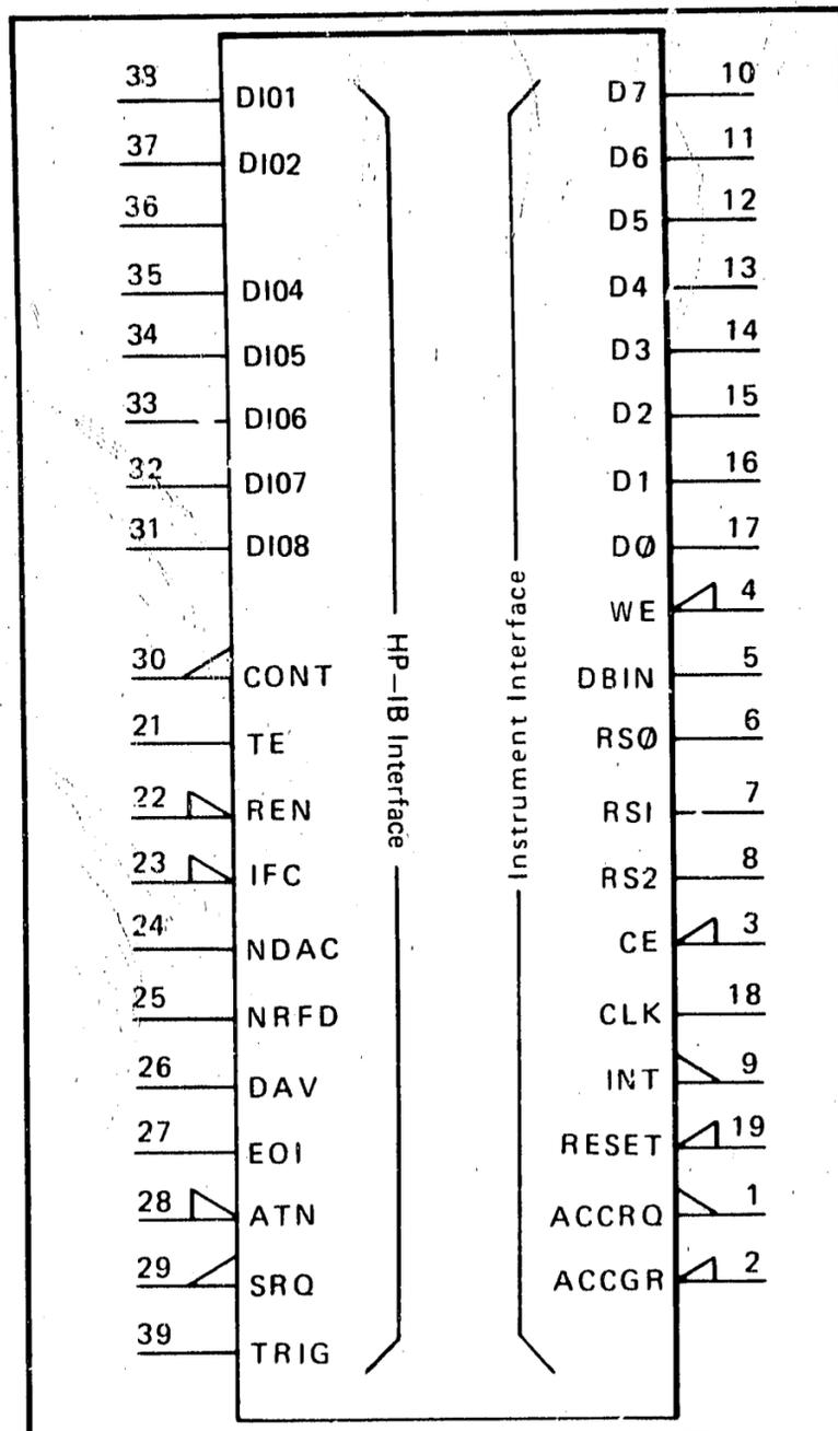
Figure 8-15. General Purpose Interface Adapter (GPIA)
