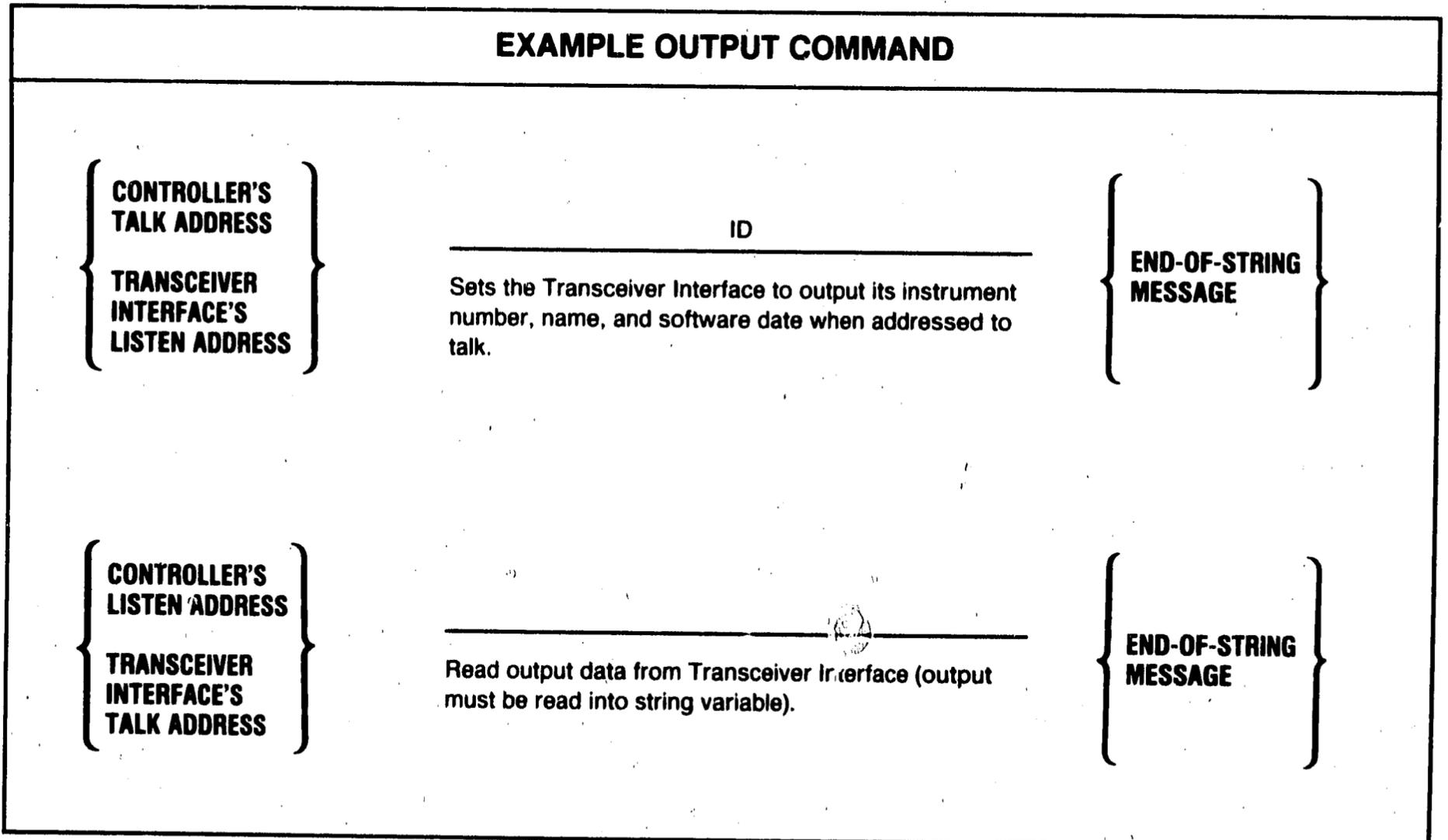
Figure 3-5. Output Command Example
