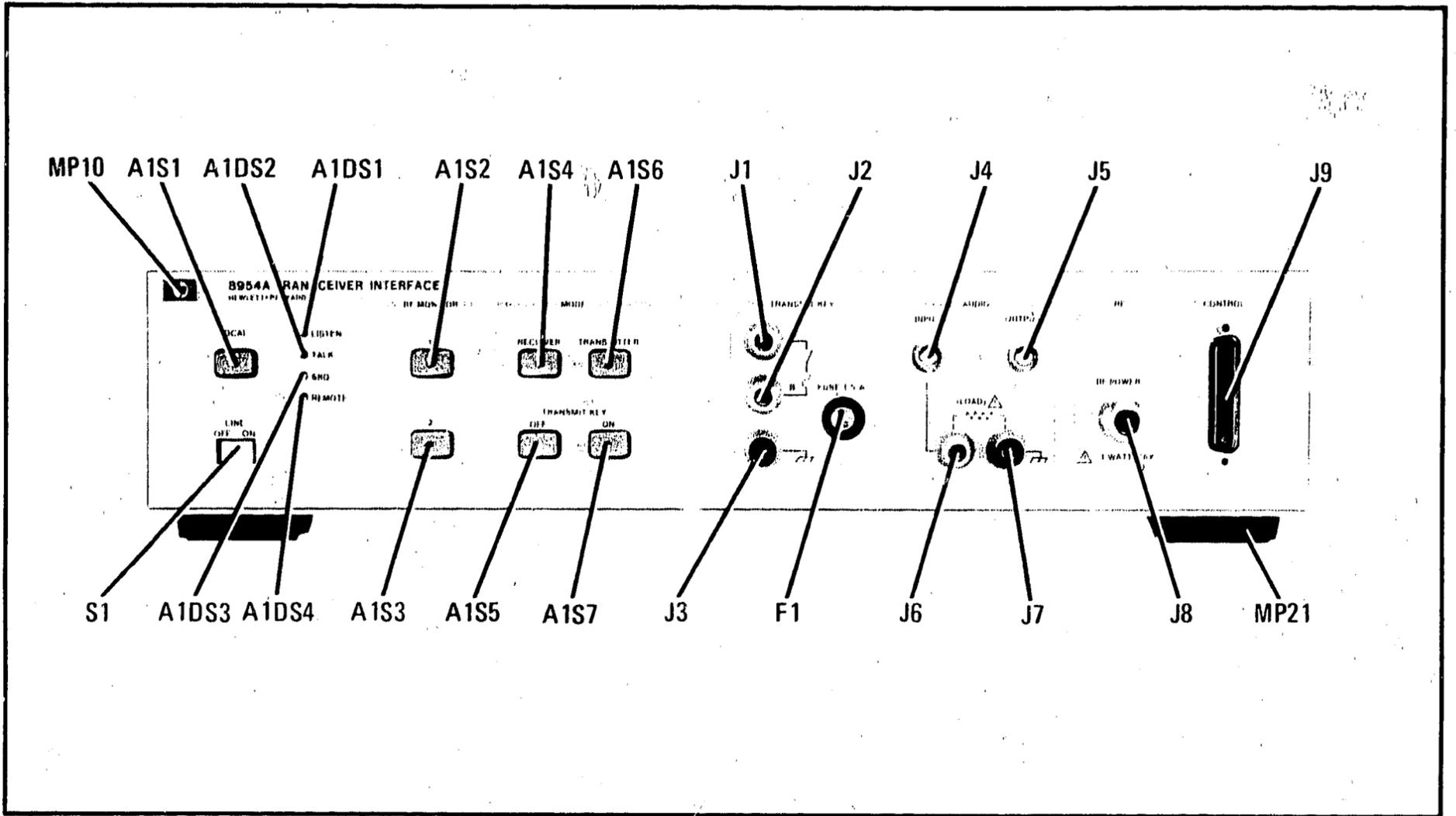
Figure 6-3. Chassis and Mechanical Parts Identification—Front Panel
