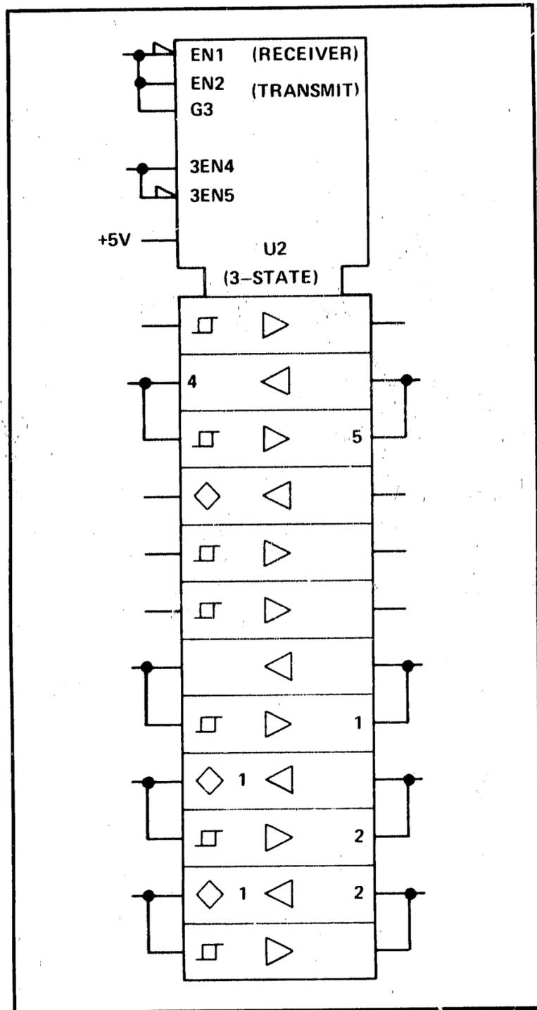
Figure 8-14. HP-IB Handshake and Control Buffer
