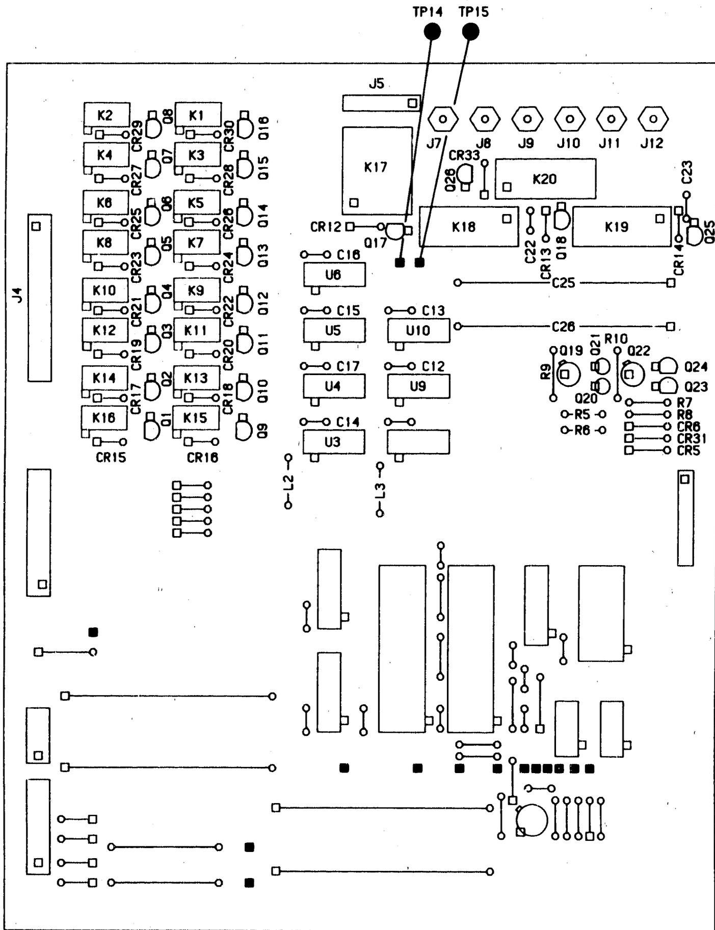
Figure 8-23. Interface Control Board (A2 Assembly) Component Locations
