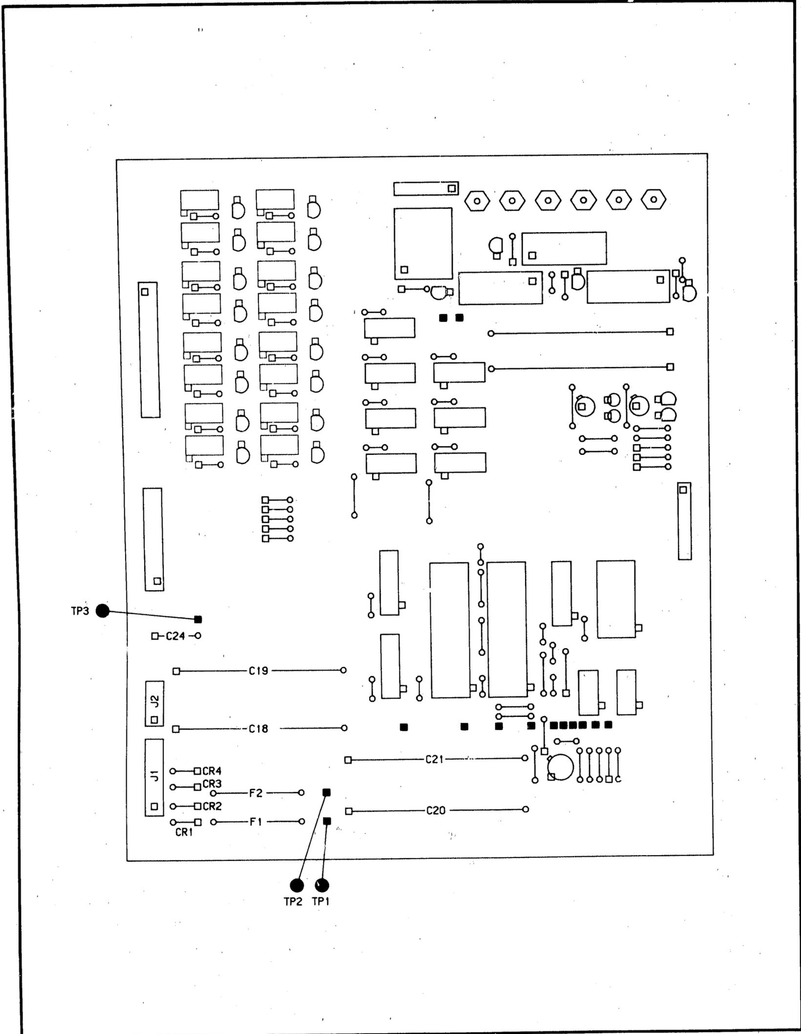
Figure 8-28. Interface Control Board (A2 Assembly) Component Locations
