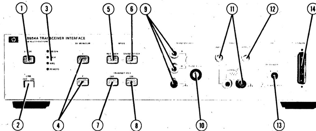
1. **LOCAL Key.** The LOCAL key returns the instrument to the local operating mode (full, front-panel control) from the remote mode of operation. The LOCAL key is disabled if a Local Lockout command has been given by the HP-IB controller.
