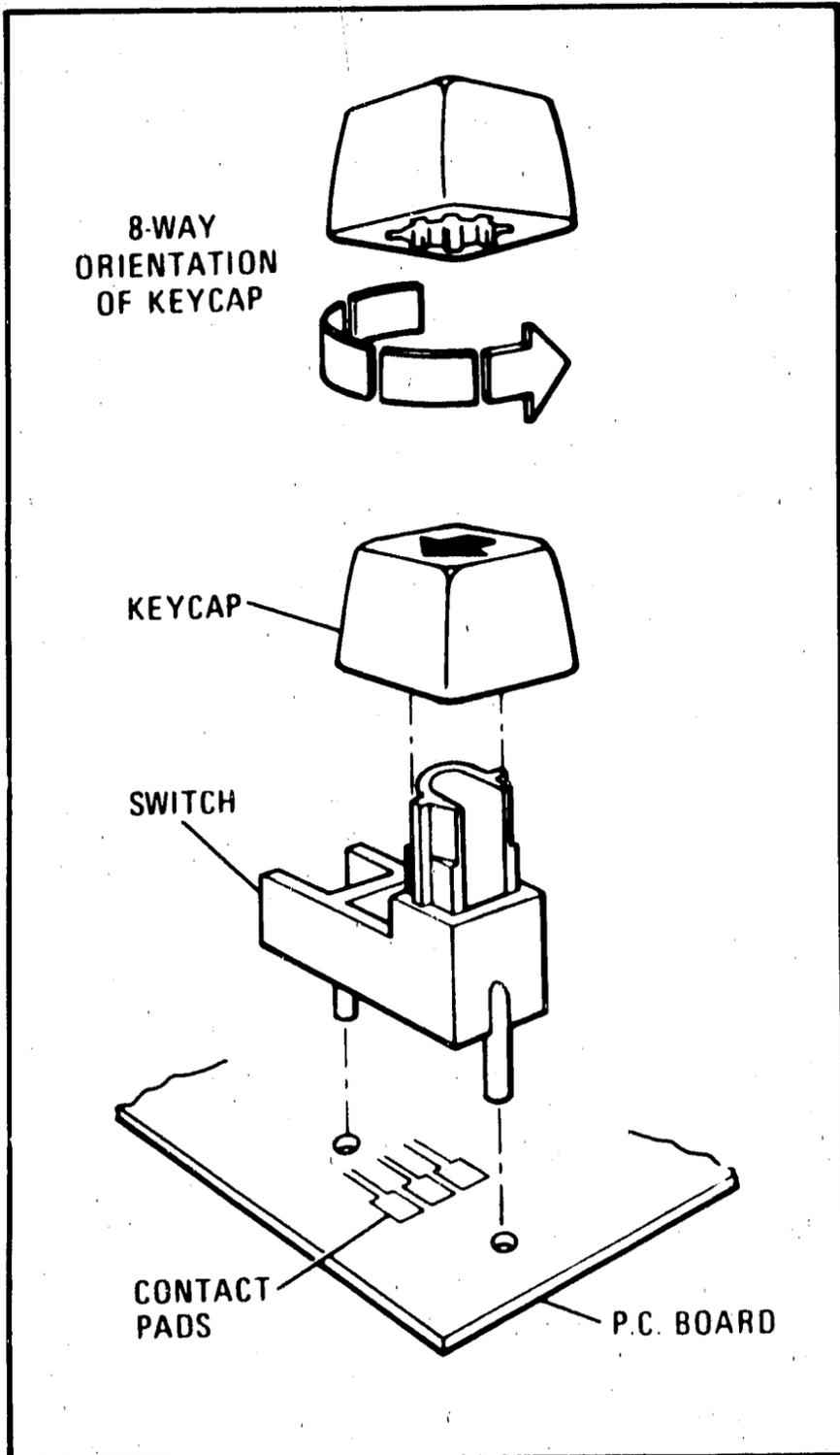
Figure 8-2. Front-Panel Pushbutton Switch Assembly
