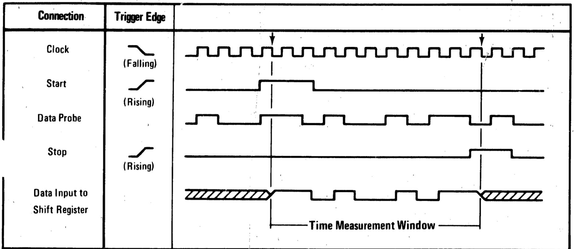
Figure 8-1. Signature Multimeter Timing Diagram
