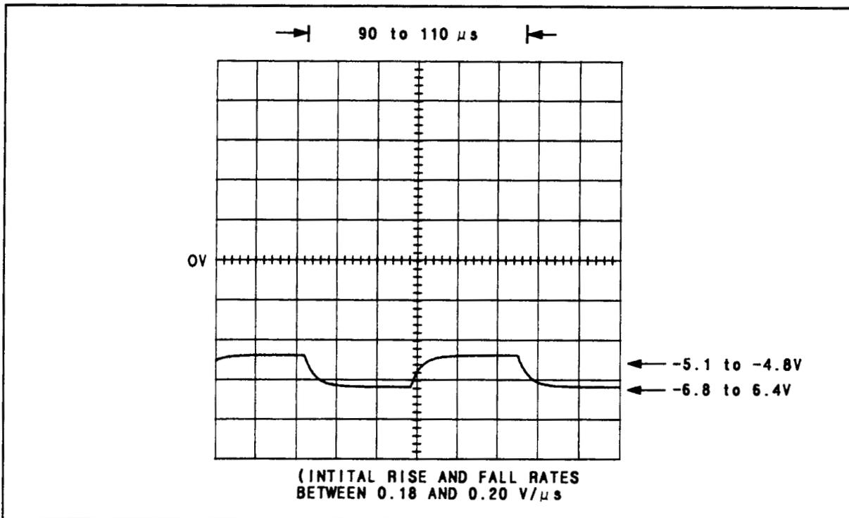
Figure 8F-45. Waveform for  $\sqrt{1}$  Step 2 (Q6 Collector)
