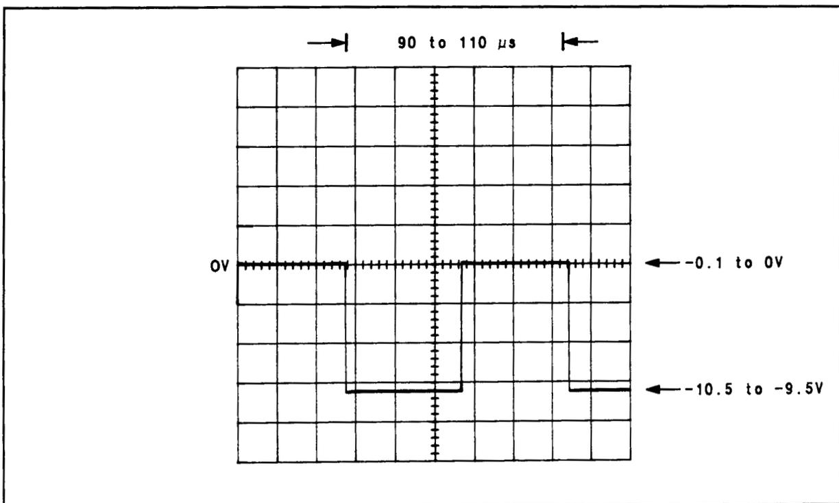
Figure 8F-40. Waveform for  $\sqrt{1}$  Step 4 (U5A pin 1)
