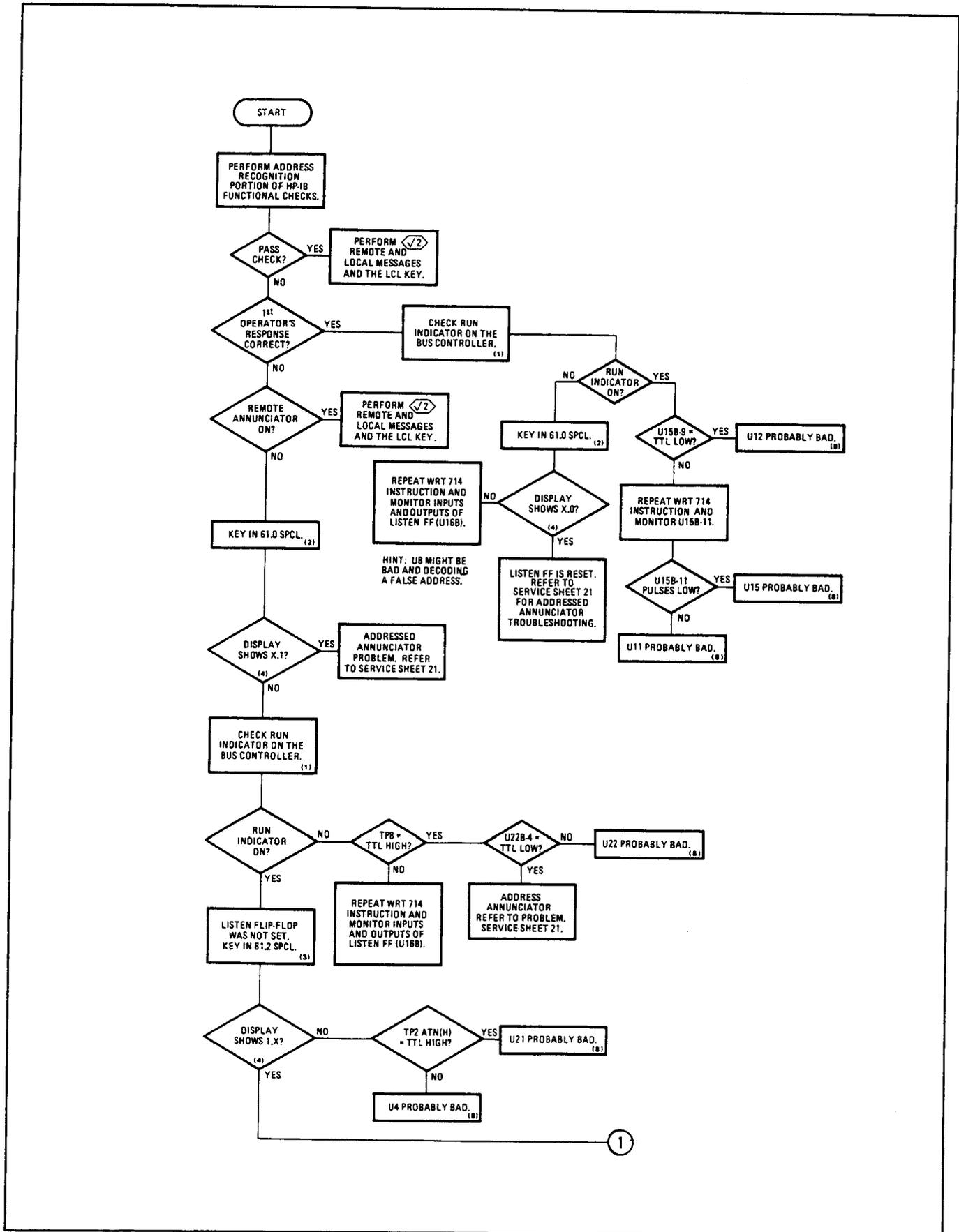
Figure 8F-35. Address Recognition Check Troubleshooting Flowchart, (√1) (1 of 2)
