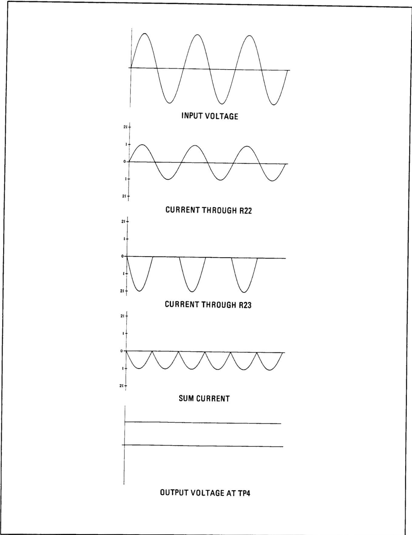
*Figure 8F-19. Waveforms in the Audio Average Detector*
