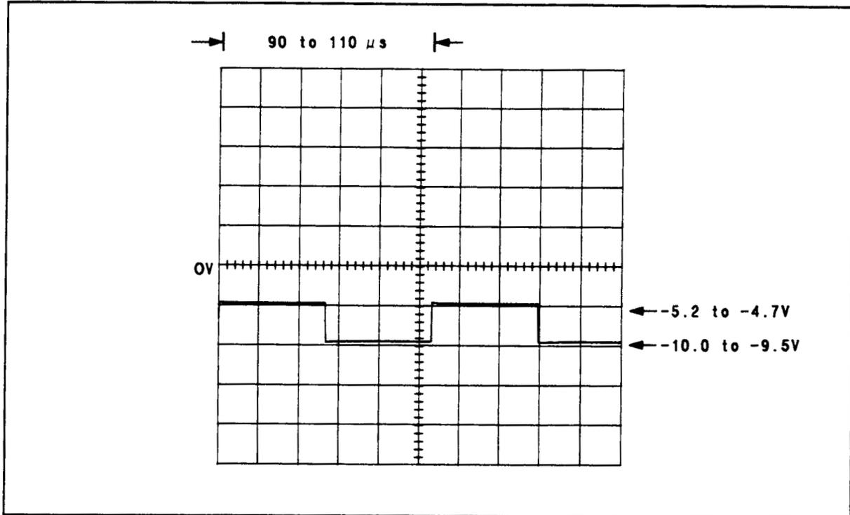
Figure 8F-44. Waveform for  $\sqrt{1}$  Step 2 (U7A pin 1)
