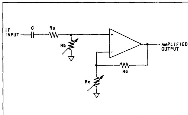
**Figure 8F-10.** Simplified Diagram of the Current-Variable Amplifier
