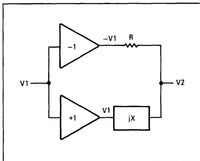
Figure 8F-8. Simplified Diagram of Phase Compensation Amplifier
