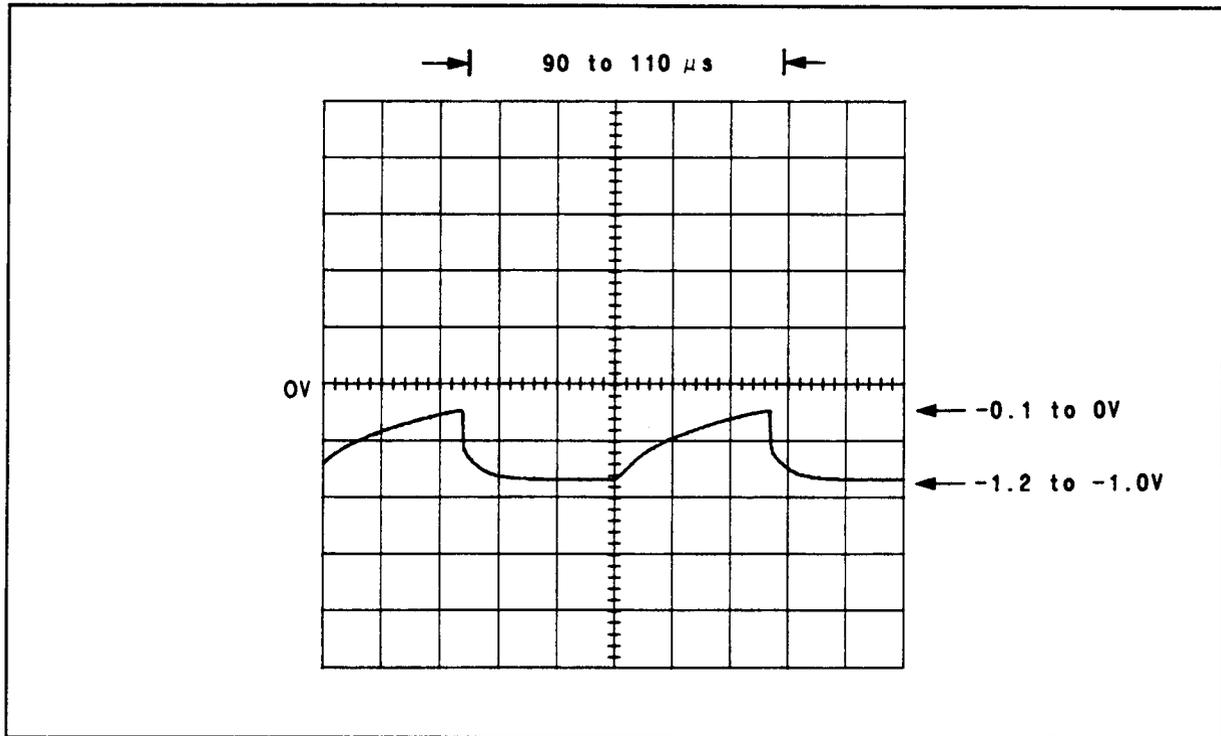
**Figure 8F-46.** Waveform for  $\sqrt{1}$  Step 2 (CR6 Cathode)
