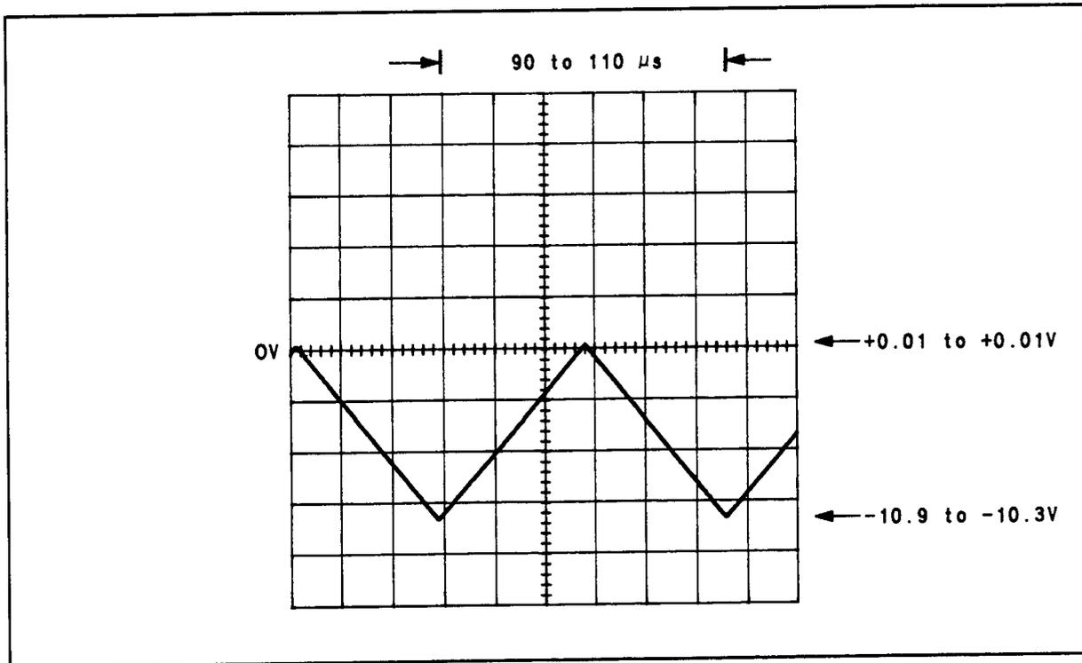
Figure 8F-41. Waveform for  $\sqrt{1}$  Step 4 (A51TP3)
