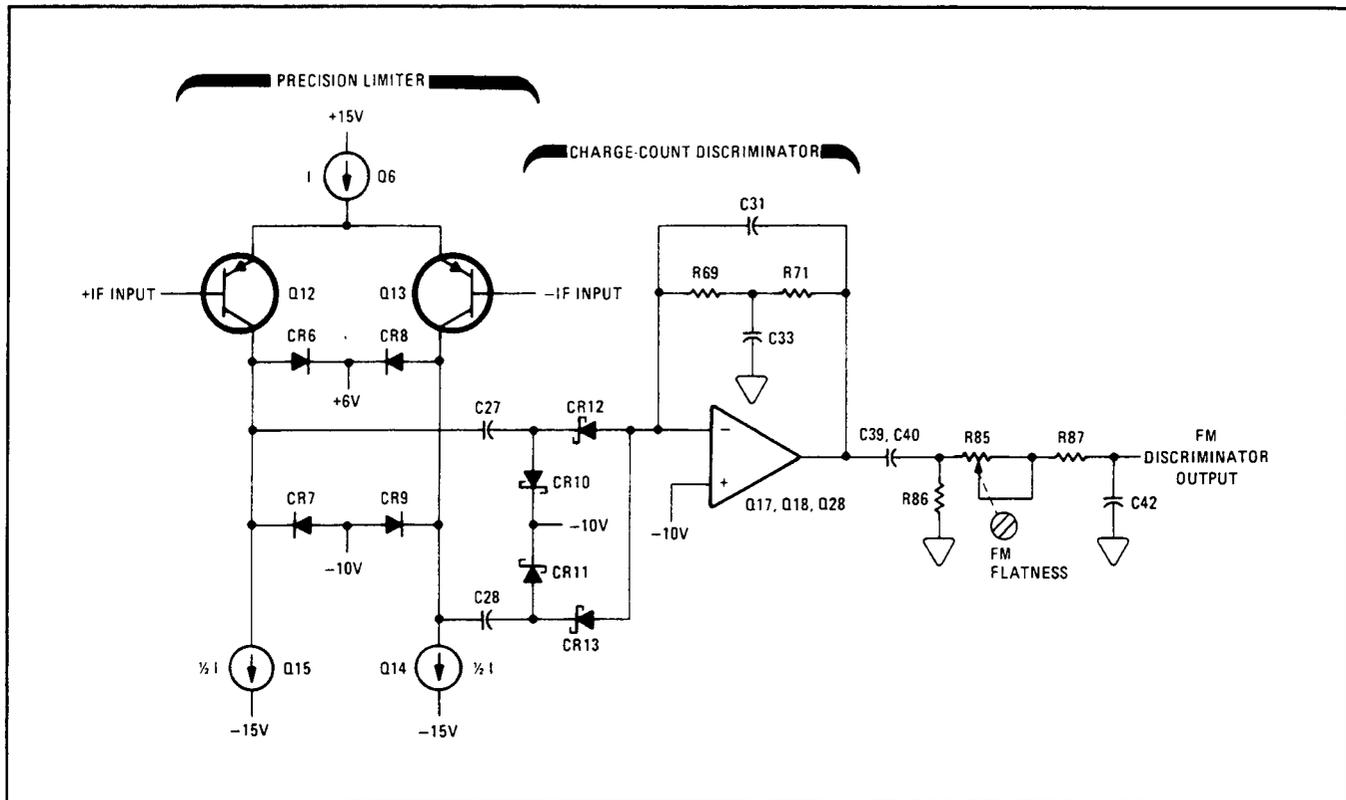
*Figure 8F-13. Simplified Schematic Diagram of FM Discriminator*
