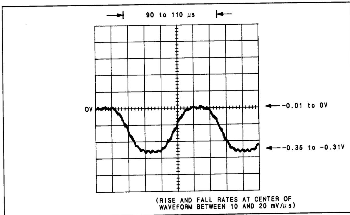
Figure 8F-42. Waveform for  $\sqrt{1}$  Step 4 (A51TP2)
