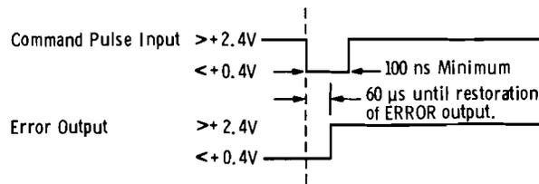
Figure 3-3. HP 8660D Data Input and Error Output Timing
