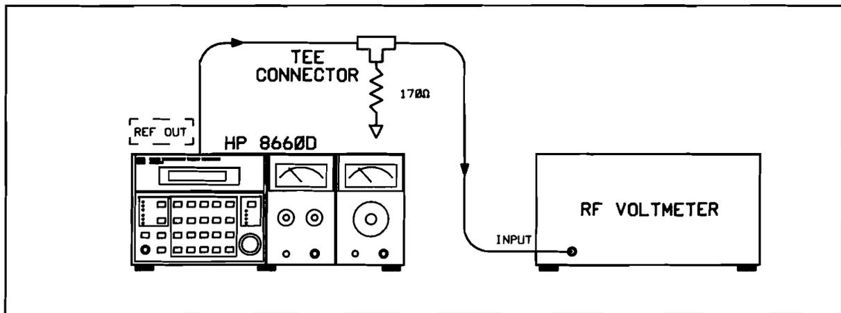
*Figure 4-2. Internal Reference Test Setup*
