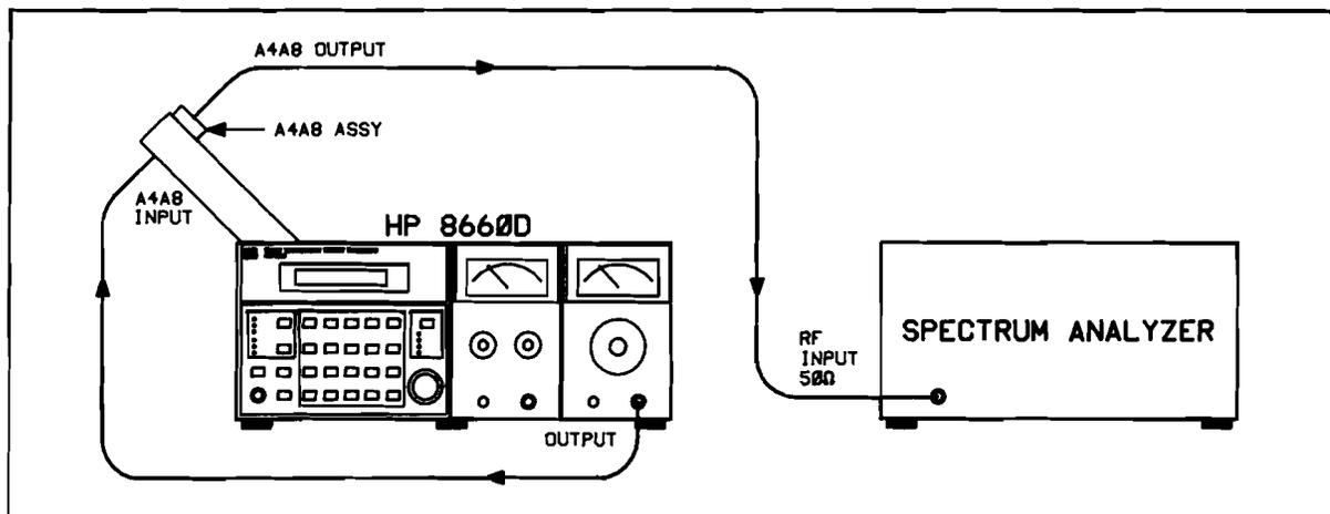
**Figure 5-7.** 100 MHz Band-pass Filter Adjustment Test Setup
