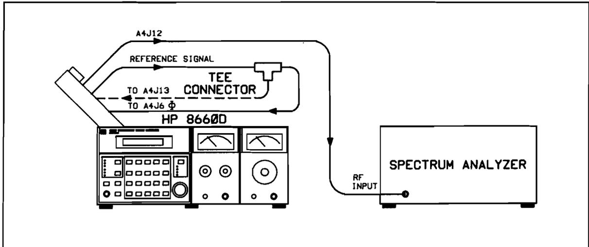
**Figure 5-16.** 10 MHz Trap Adjustment Test Setup
