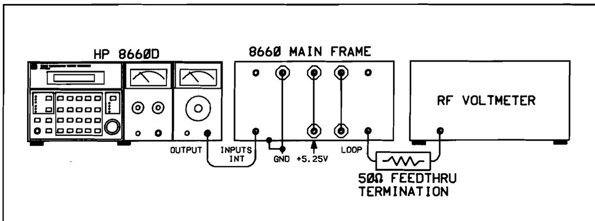
*Figure 5-9. A22A1 Adjustment Test Setup (After Repair)*
