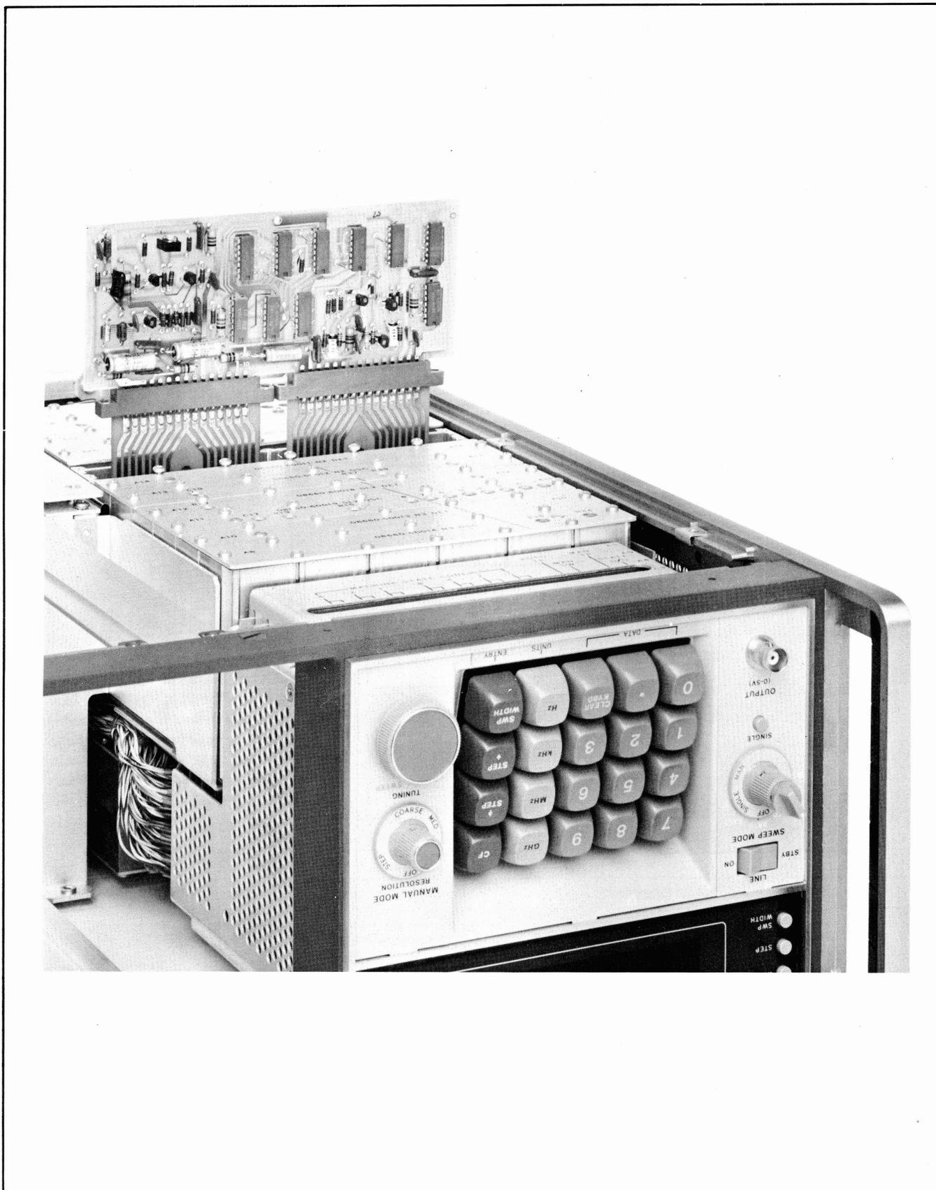
Figure 8-3. Model 8660C With Circuit Board Extended for Maintenance
