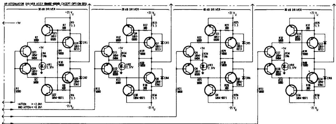
Figure 7-6. P/O Attenuator Section Schematic Diagram (Change D)
