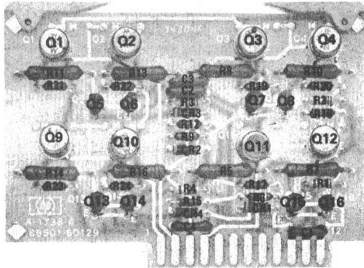
Figure 8-21. A9 Attenuator Driver Assembly Component Locations (P/O Change 1)
