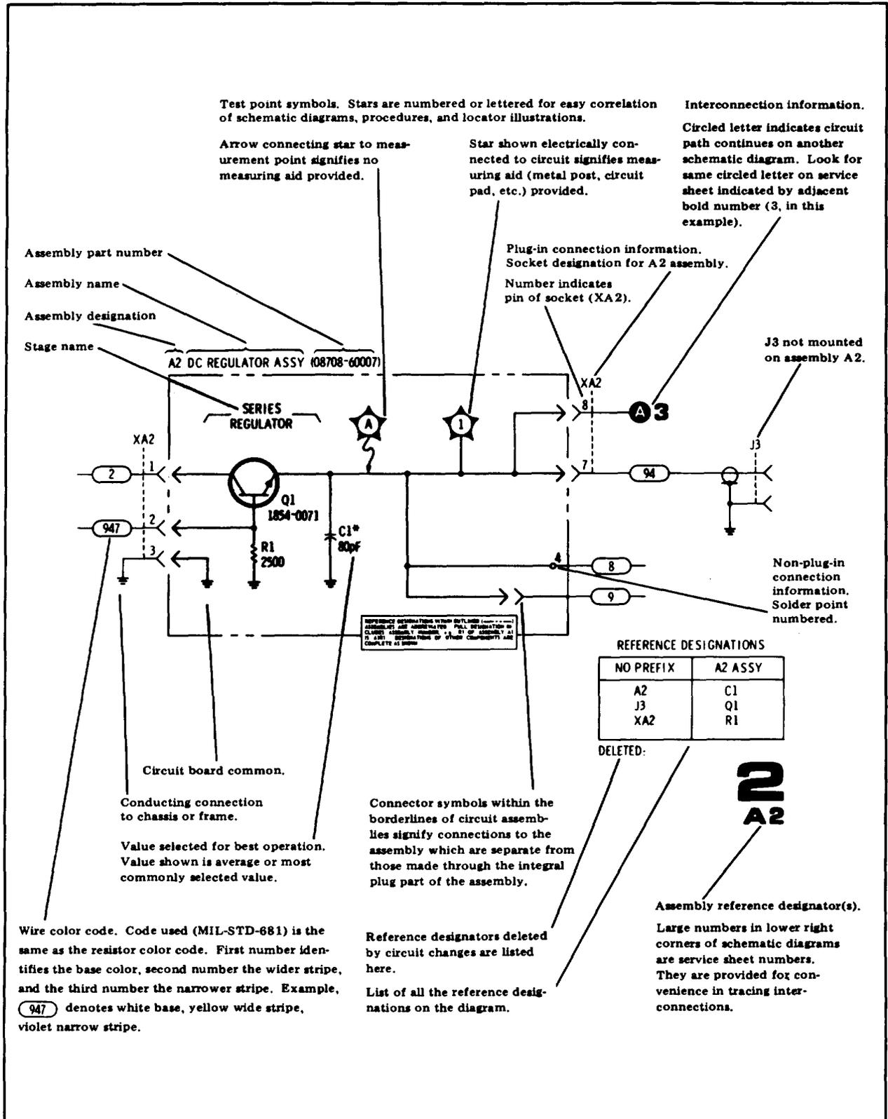
Figure 8-3. Schematic Diagram Notes (3 of 3)
