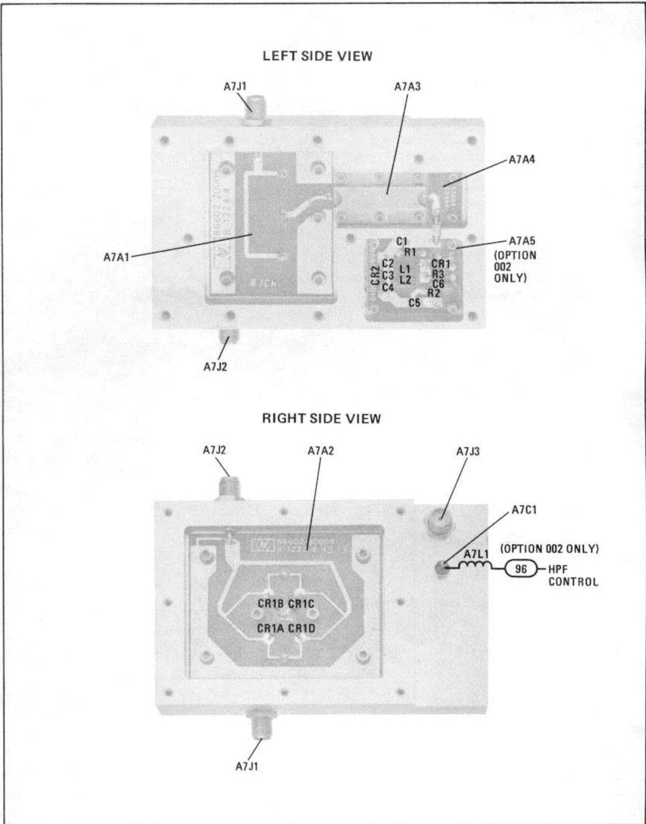
Figure 8-10. A7 Mixer Assembly's subAssembly and Component Locations
