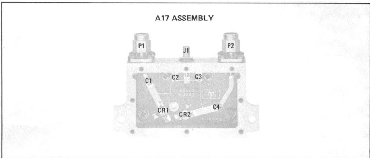
Figure 8-13. A17 Phase Modulator Assembly component Locations
