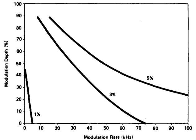
Typical AM Distortion (Center Frequency > 10 MHz)
