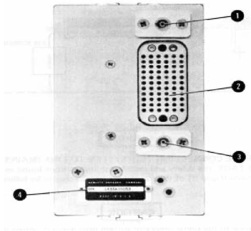
① **Coaxial Plug.** Connects the 3.95 to 2.75 GHz RF Input signal to the RF Section from the Frequency Extension Module.
