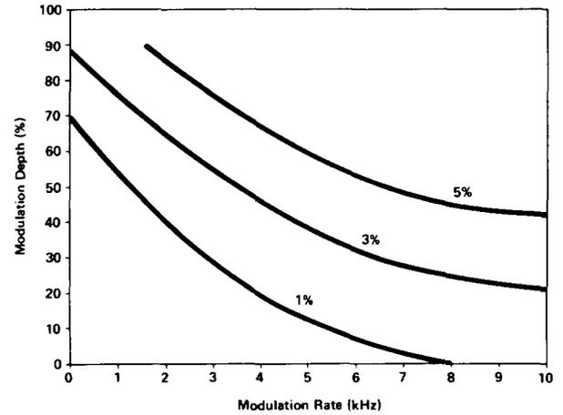
Typical AM Distortion (Center Frequency <10 MHz)
