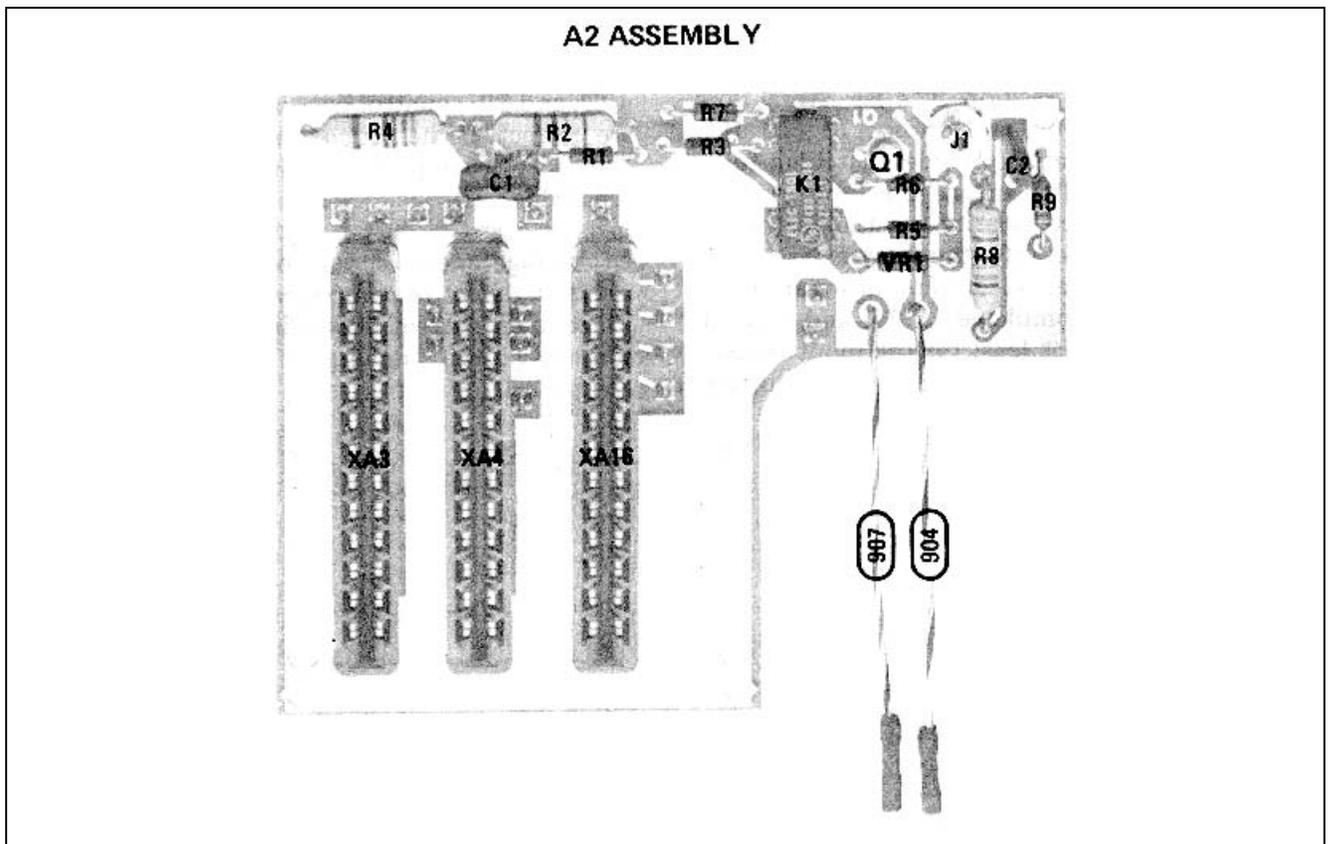
Figure 8-19. A2 ALC Mother Board Assembly Component Locations
