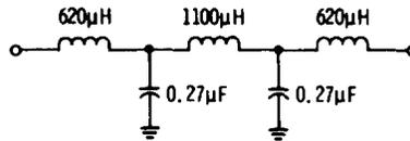
Figure 1-3. 15 kHz Low Pass Filter
