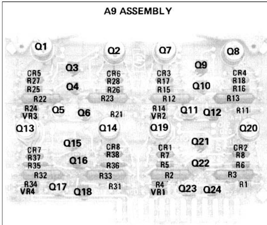
Figure 8-21. A9 Attenuator Driver Assembly Component Locations.
