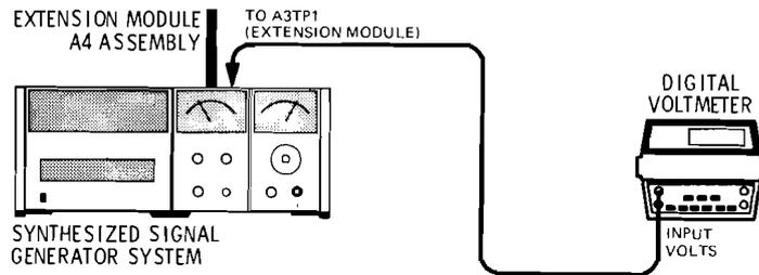
Figure 5-8. Sum Loop Pretune Adjustment Test Setup
