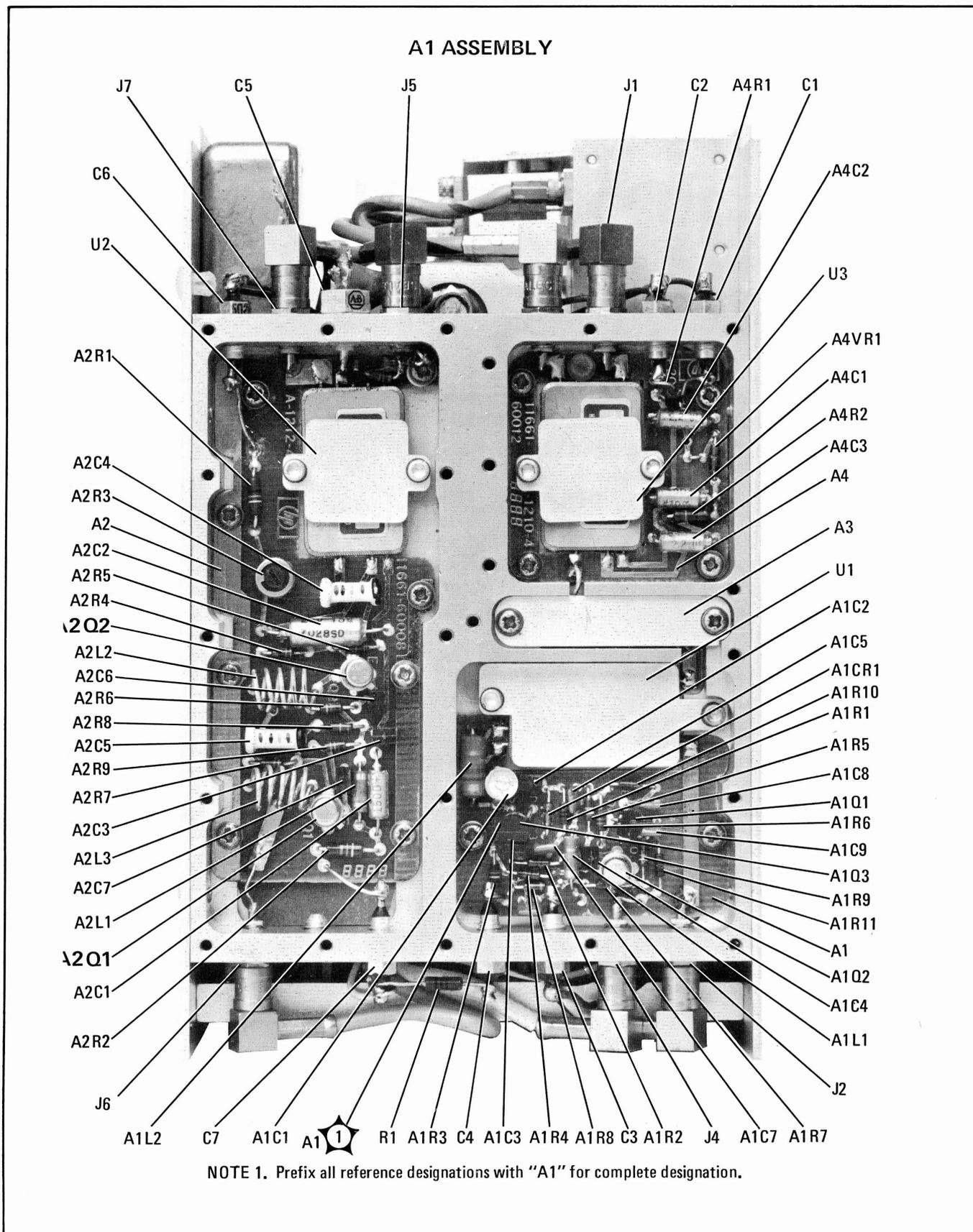
Figure 8-6. A1 Oscillator/Mixer Housing Assembly Component and Test Point Locations
