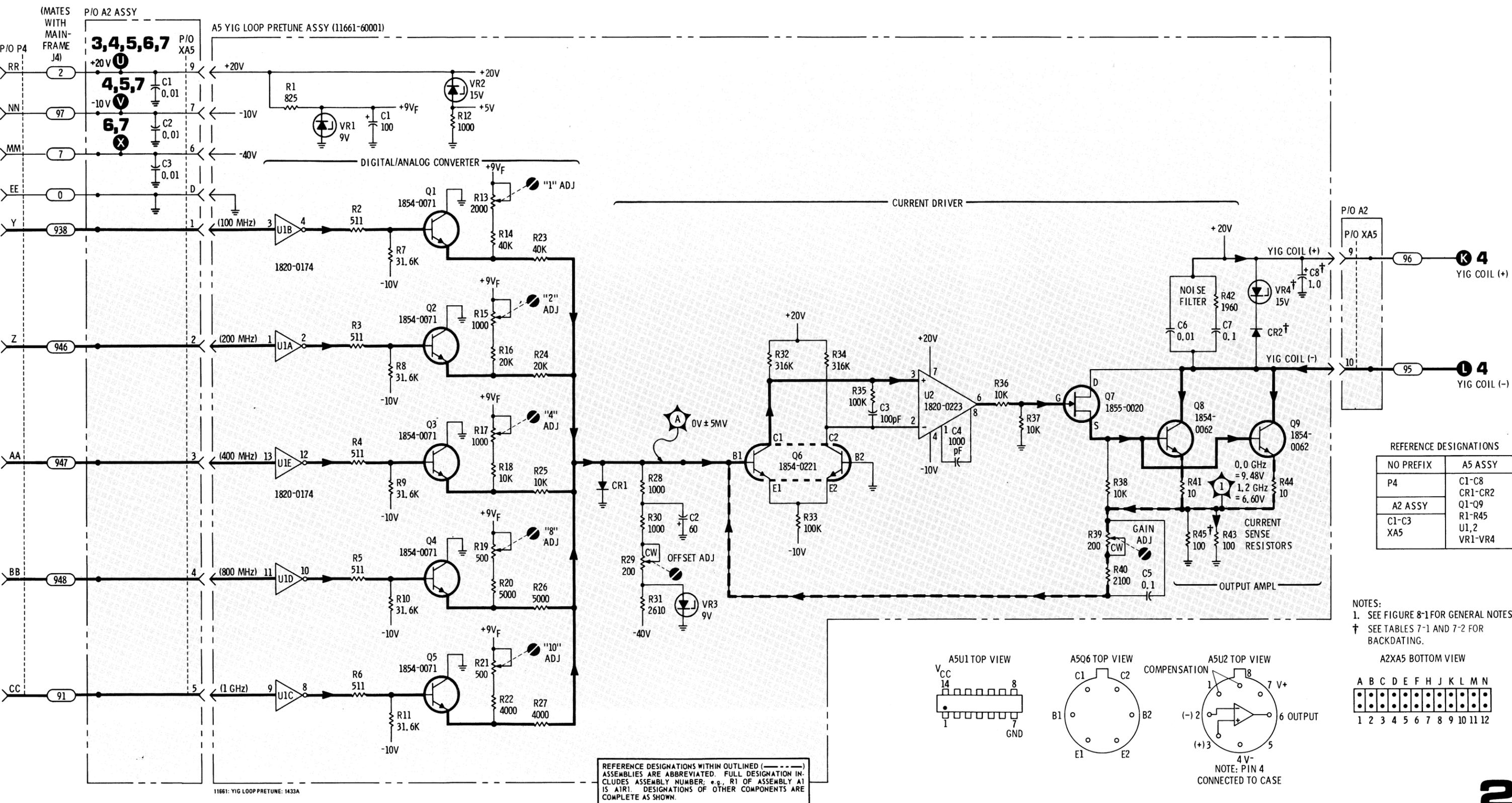
Figure 8-5. YIG Loop Pretune Section Schematic Diagram
