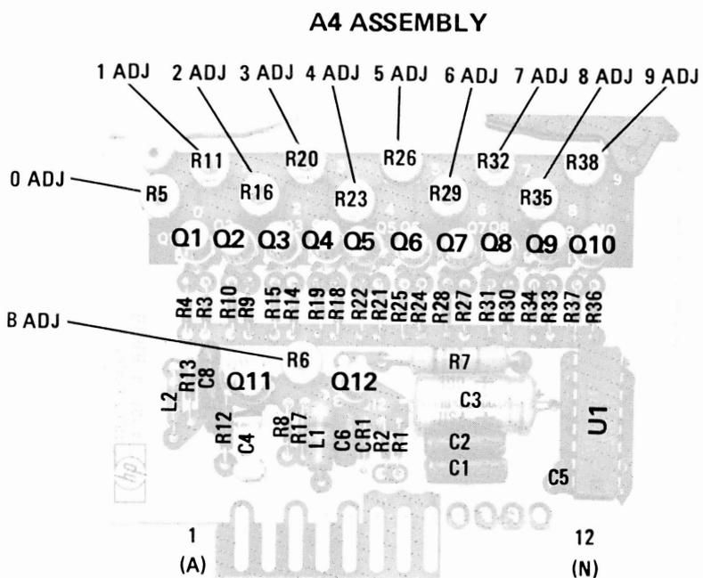
Figure 8-14. A4 Sum Loop Pretune Assembly Component Locations
