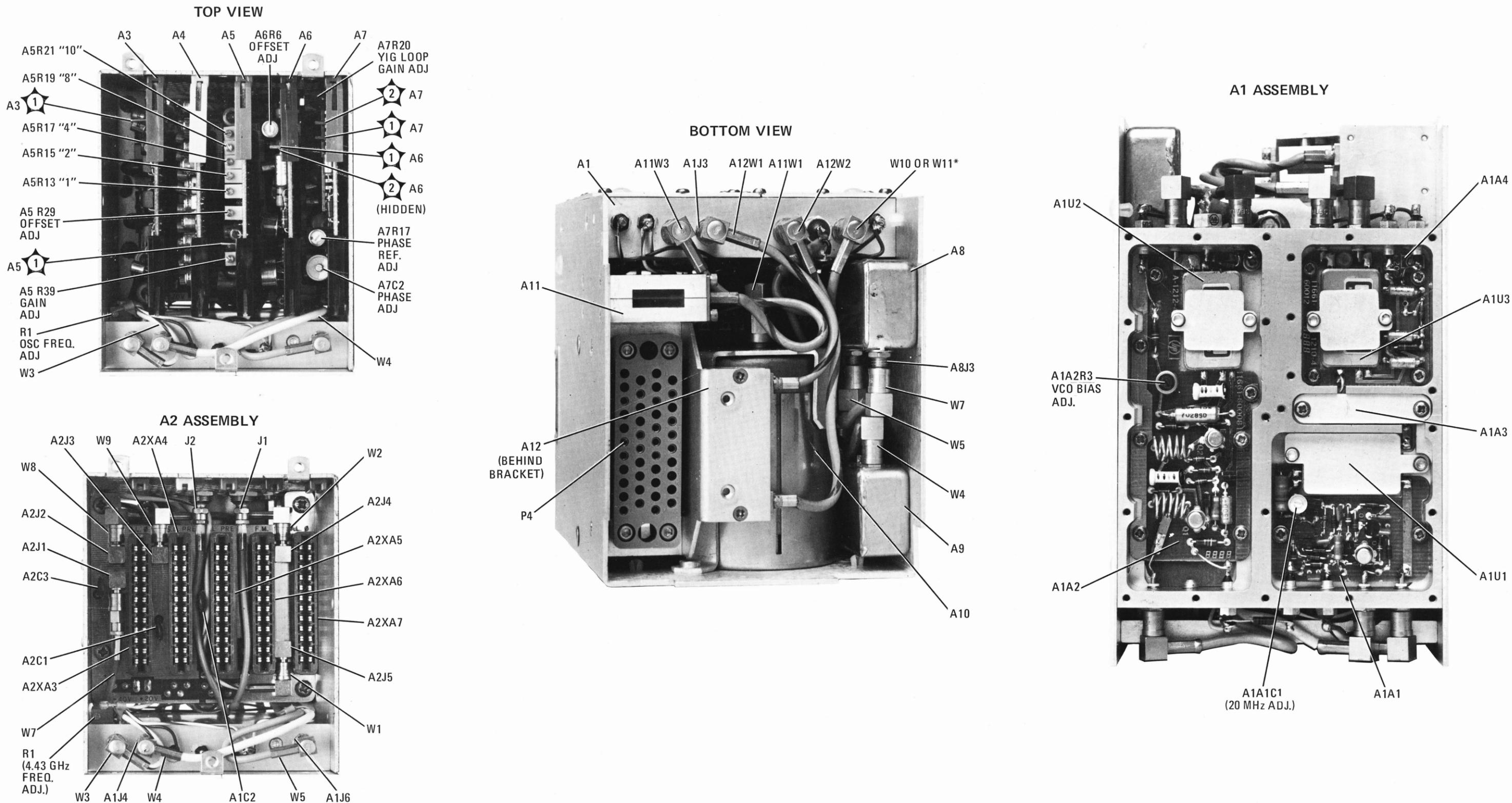
Figure 8-17. Assemblies, Chassis Mounted Parts, Adjustment Locations and Test Point Locations
