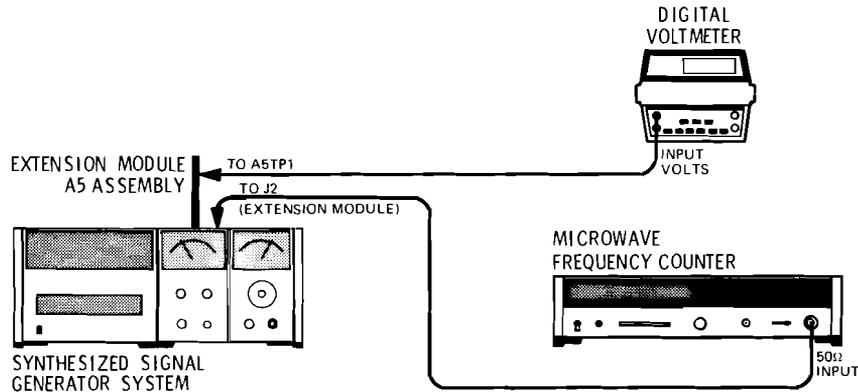
*Figure 5-5. YIG Pretune Driver Adjustment Test Setup*
