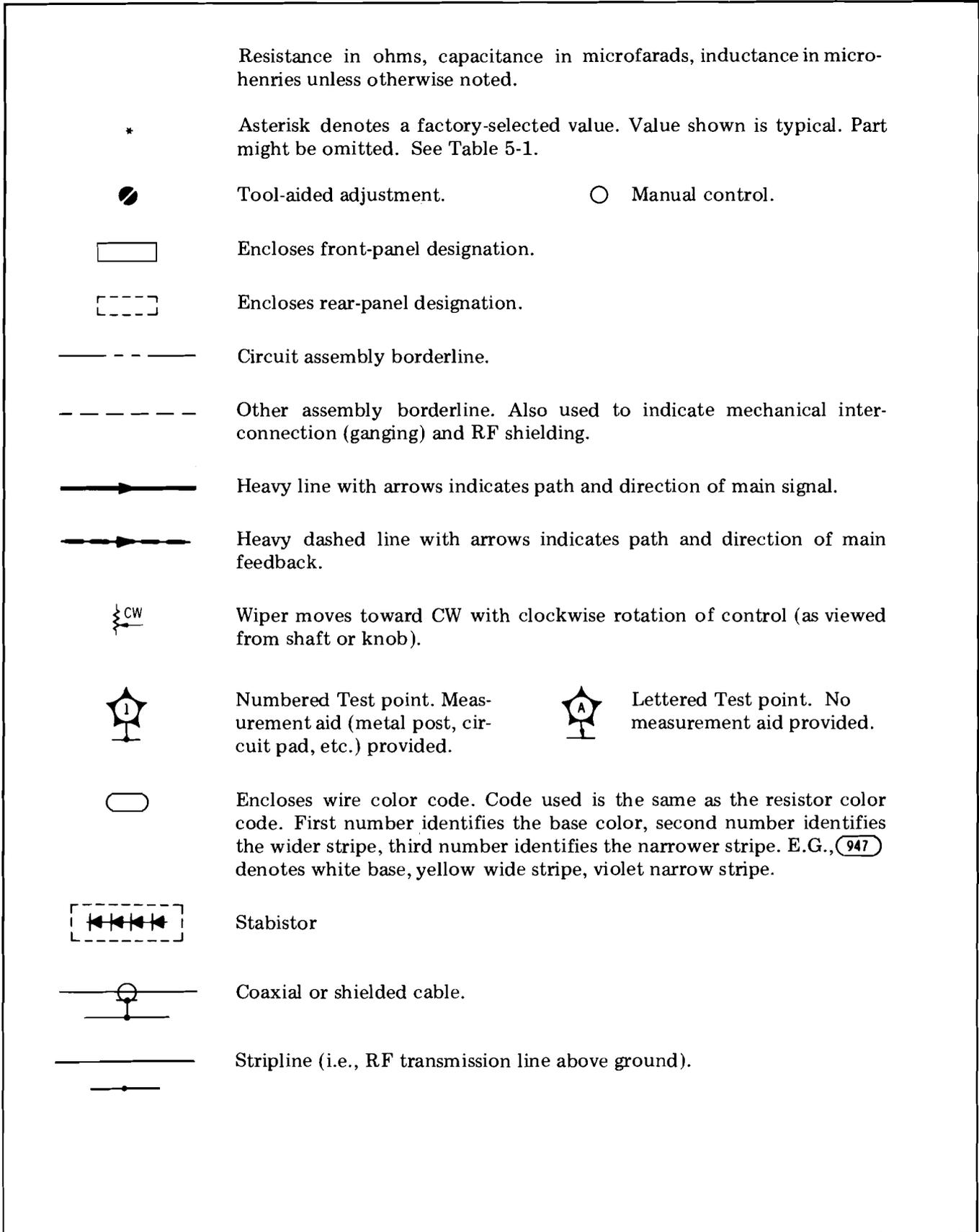
Figure 8-1. Schematic Diagram Notes (1 of 2)
