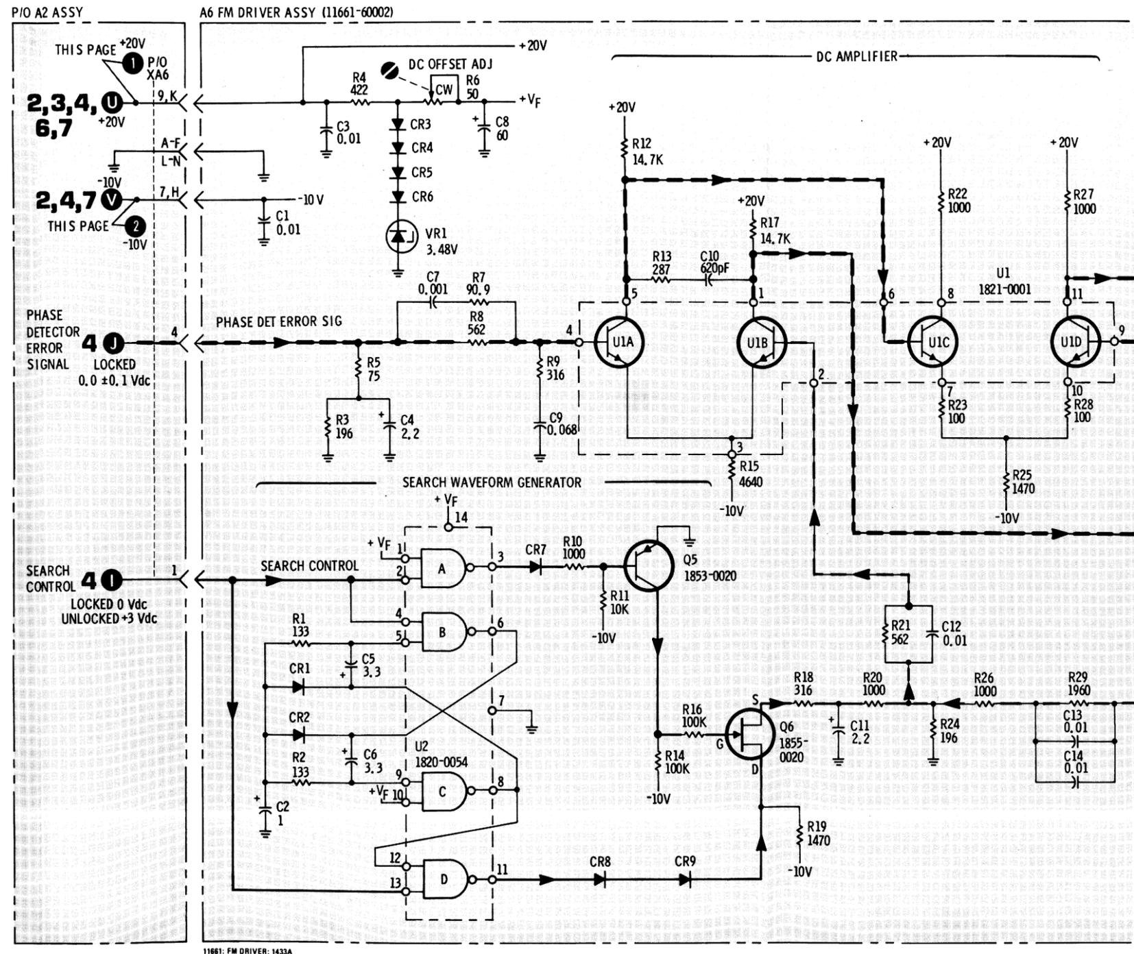
Figure 8-10. A6 FM Driver Assembly Component and Test Point Locations
