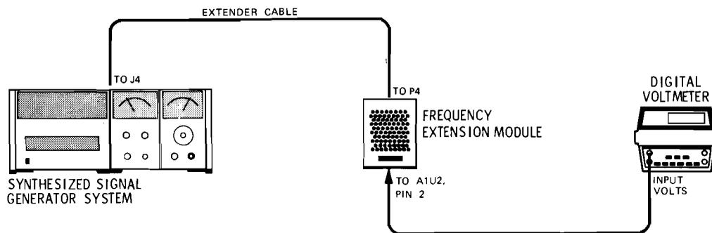
Figure 5-4. 3.95 to 4.05 GHz VCO Bias Adjustment Test Setup
