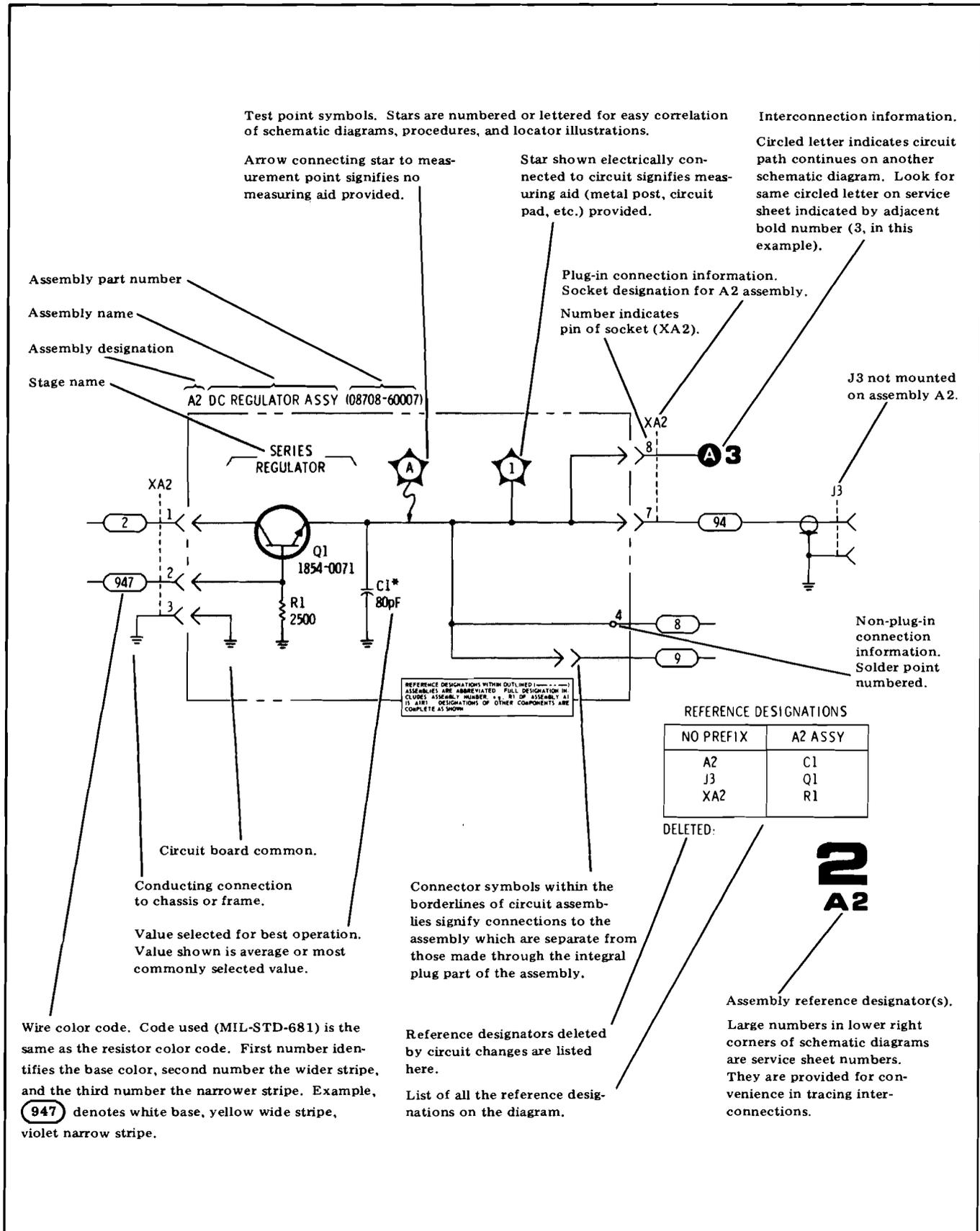
Figure 8-1. Schematic Diagram Notes (2 of 2)
