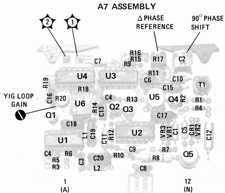
Figure 8-8. A7 YIG Loop Phase Detector Assembly Component and Test Point Locations
