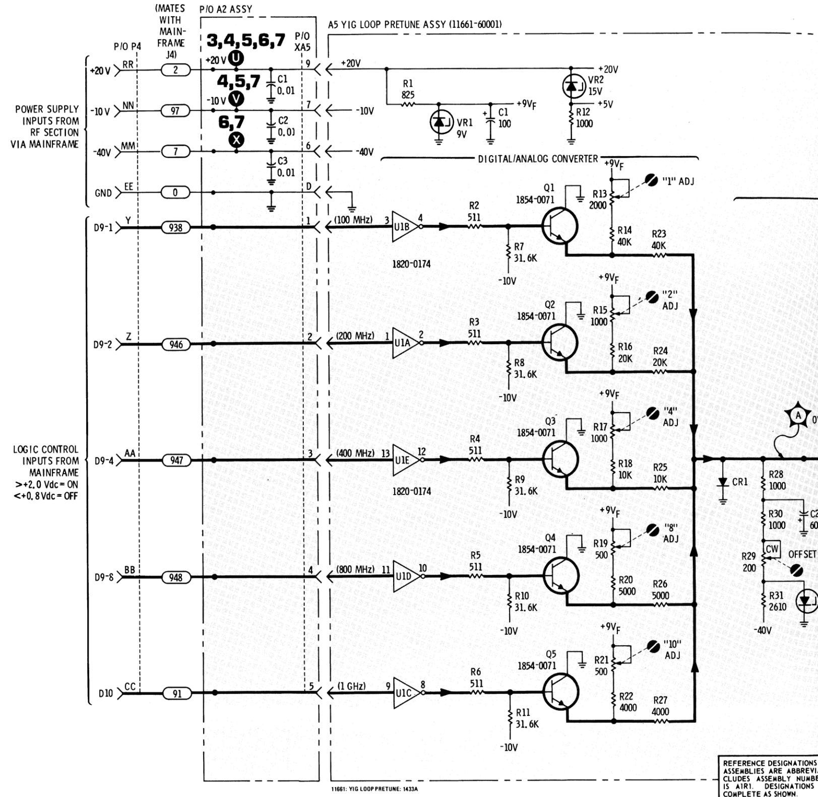
Figure 8-4. A5 YIG Loop Pretune Assembly Component and Test Point Locations
