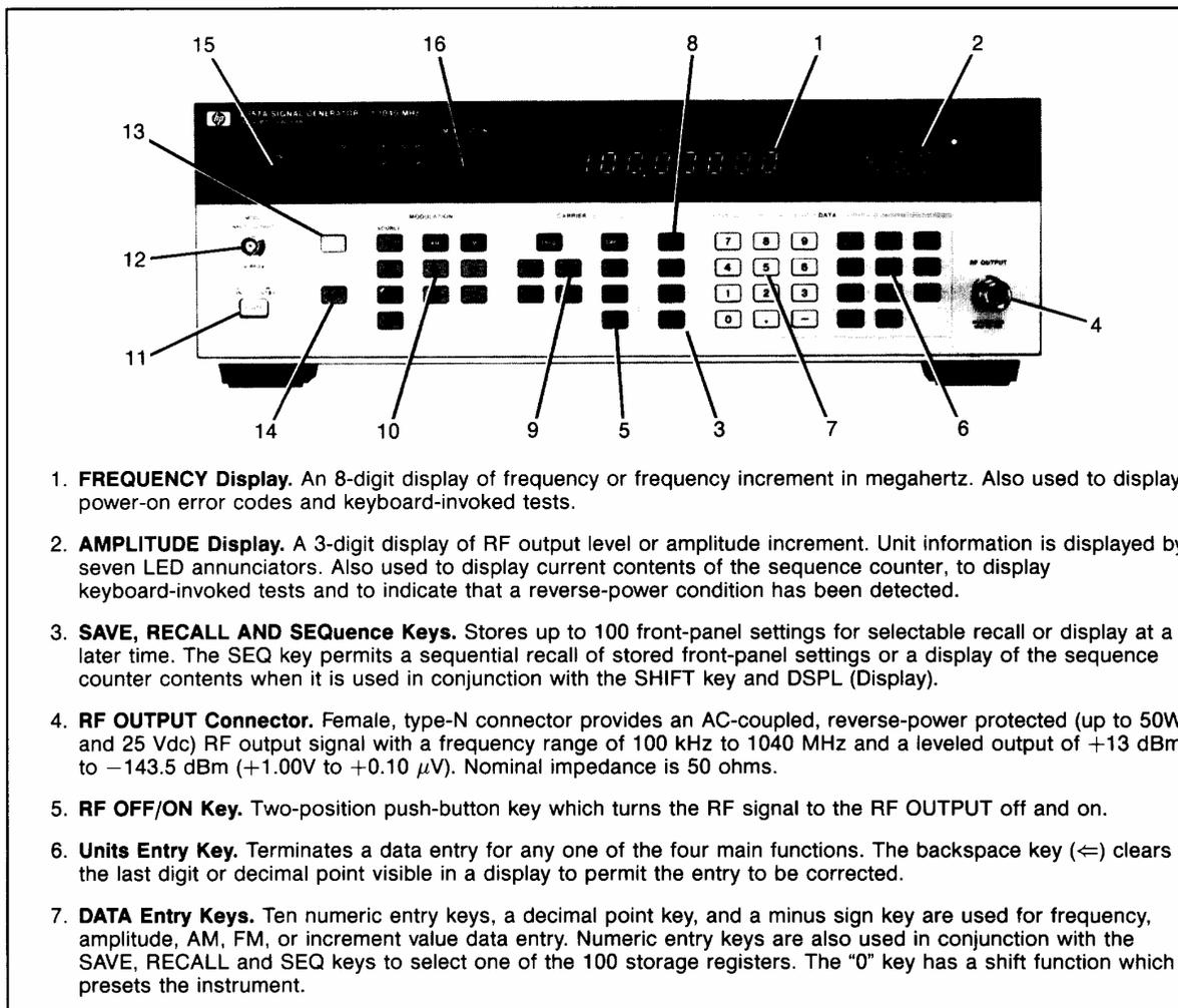
*Figure 3-1. Front Panel Features and Simplified Operation (1 of 3)*
