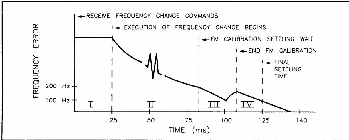
**Figure 3-6.** Typical Frequency Switching Characteristics.
