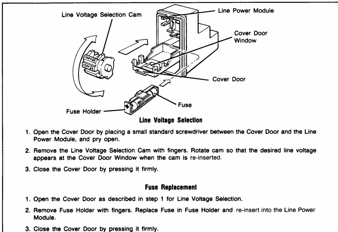
*Figure 2-1. Line Voltage Selection and Fuse Replacement*
