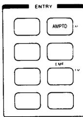
This key makes amplitude the active function so its value can be set using either Data keys, the Knob, Step keys, or the Off/On key.
