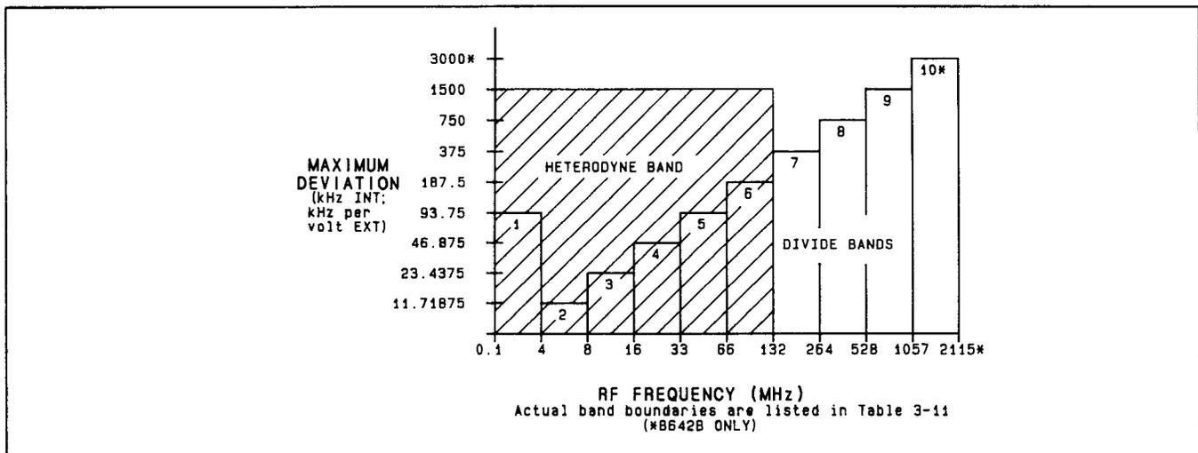
**Figure 3-13. FM Deviation Limitations for each RF Frequency Band;
