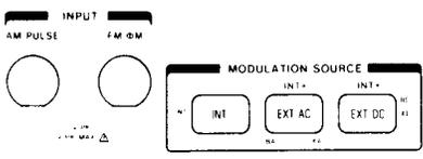
The Modulation Source keys select whether an internal or external source is used (or internal and external sources combined). The source of the external modulation is coupled through the input connectors.
