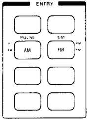
These keys make AM, FM, or  $\Phi$ M the active function so its value can be set using either Data keys, the Knob, Step keys, or the Off/On key. Also Pulse Modulation can be turned on or off. You can select either AM or Pulse Modulation simultaneously with either FM or  $\Phi$ M.
