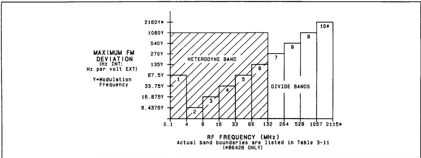
**Figure 3-12. FM Deviation Limitations for each RF Frequency Band;
