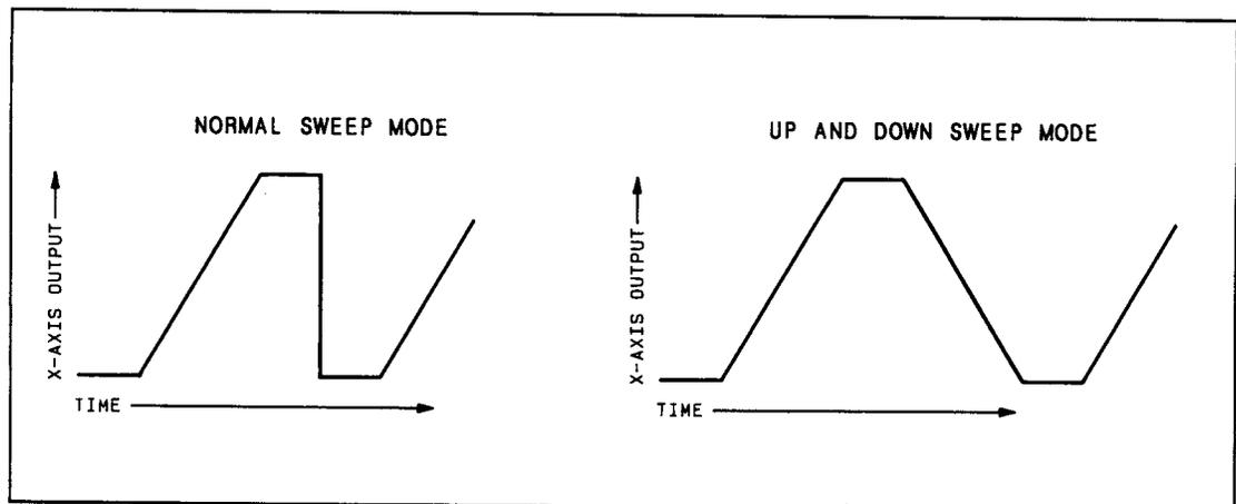
Figure 3-7. Sweep Waveforms
