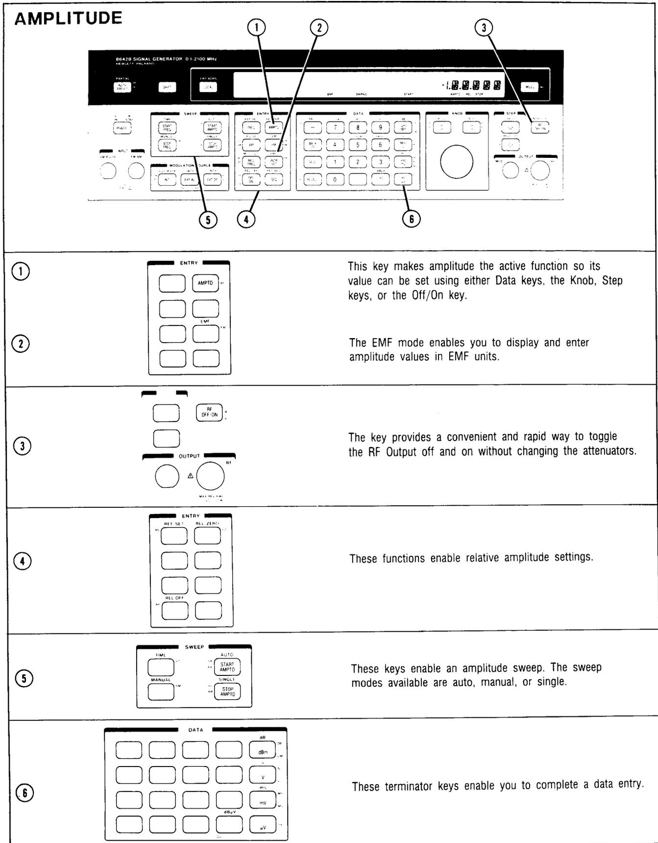
Figure 3-8. Amplitude-Related Functions
