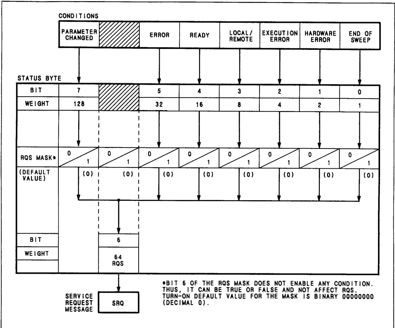
Figure 3-4. The Status Byte and RQS Mask
