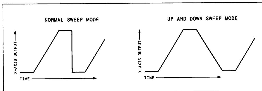
Figure 3-10. Sweep Waveforms
