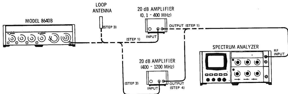
Figure 4-15. Output Leakage Test Setup
