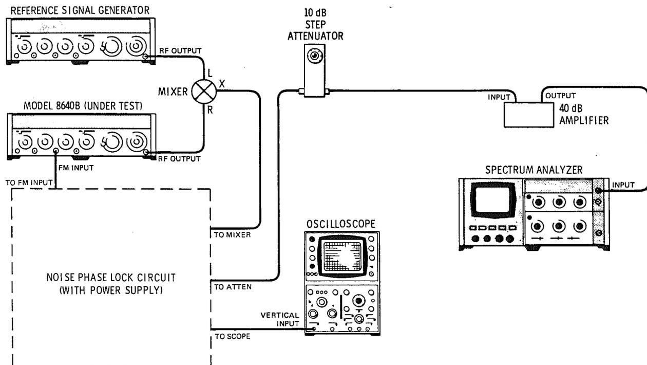
Figure 4-6. Single Sideband Phase Noise Test Setup
