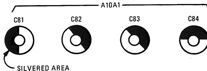
Figure 5-6. 256-512 MHz High Band Capacitor Adjustment Orientation
