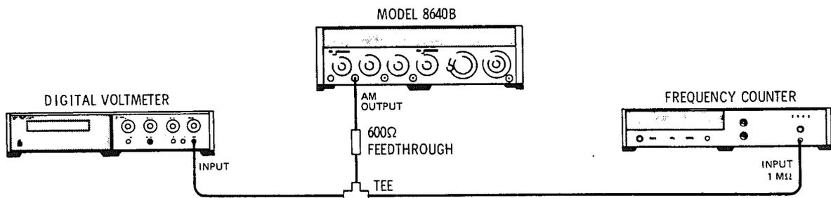
Figure 4-16. Internal Modulation Oscillator Test Setup
