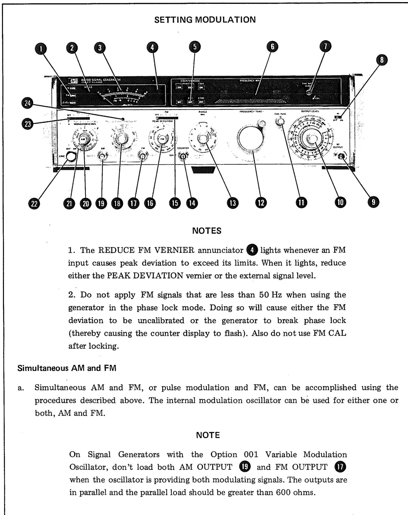
Figure 3-6. Setting the Modulation Controls (4 of 4)
