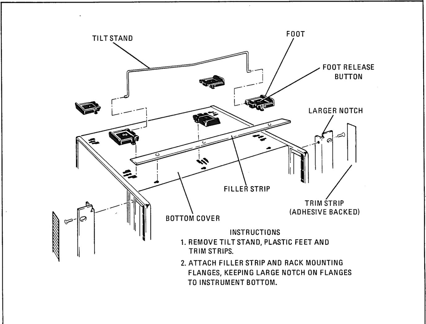
Figure 2-3. Preparation for Rack Mounting
