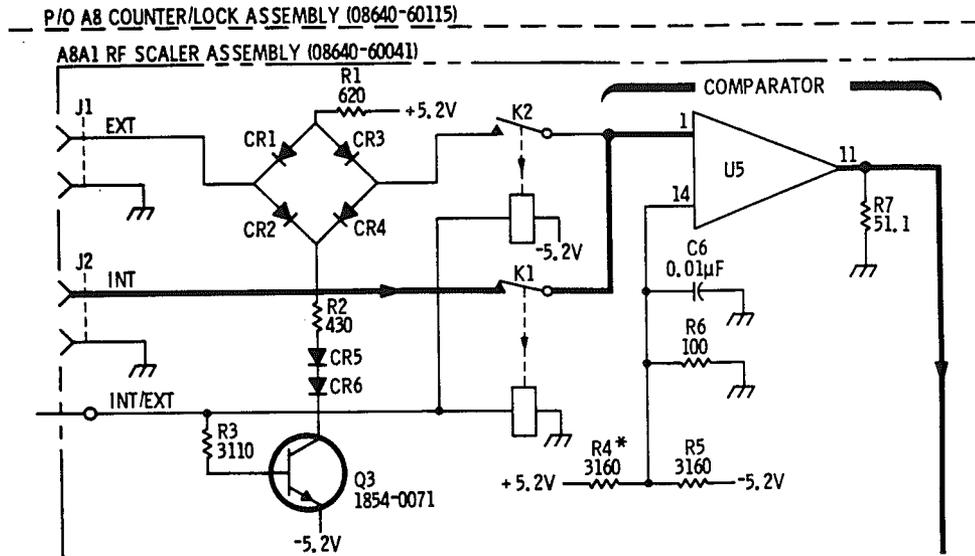
Figure 7-7. A8A1 RF Scaler Assembly Backdating (Change J)
