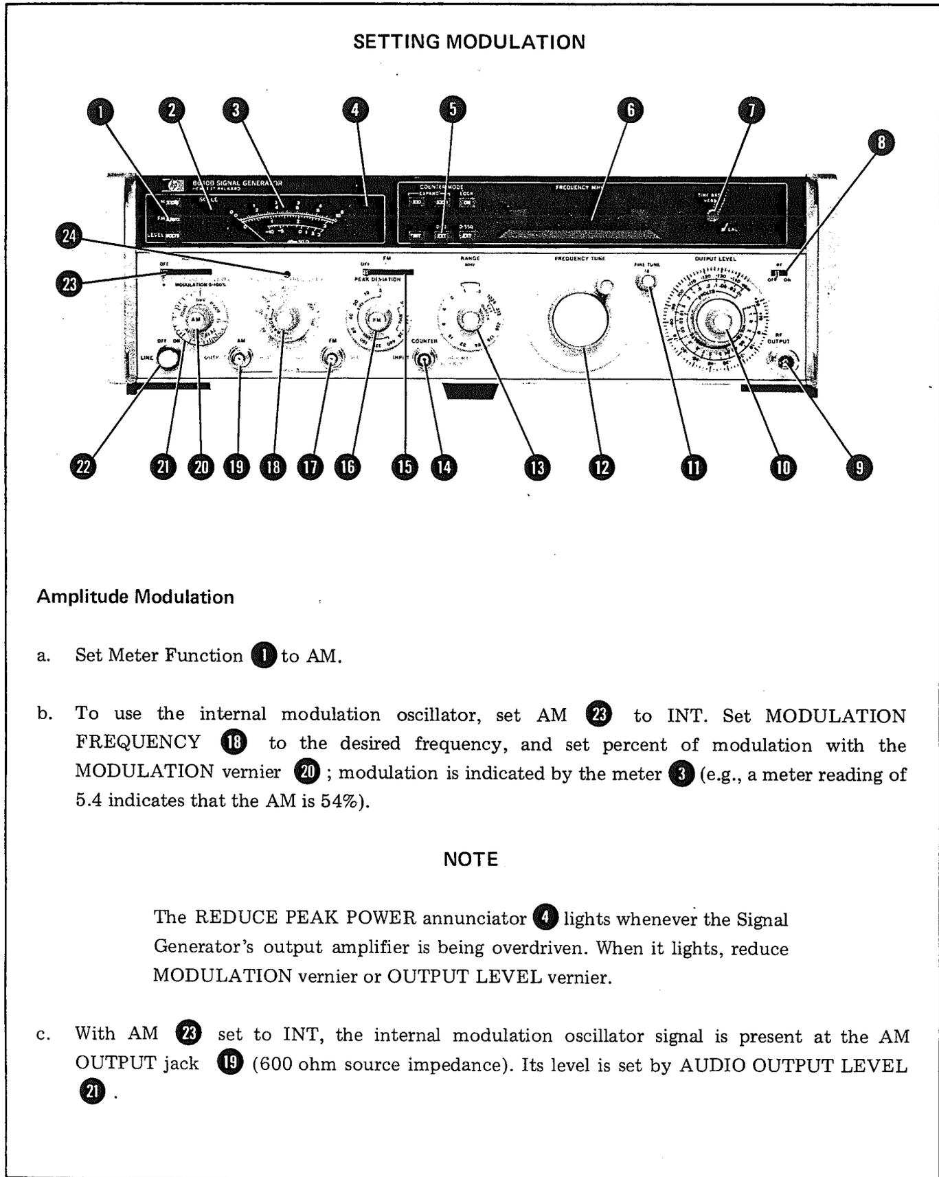
Figure 3-6. Setting the Modulation Controls (1 of 4)
