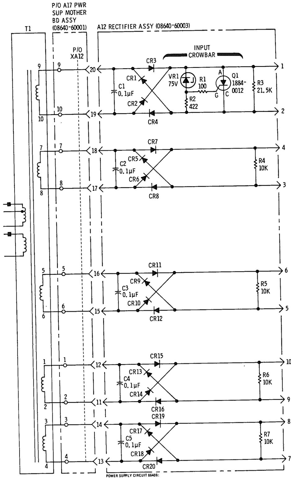
Figure 7-6. A12 Rectifier Assembly Backdating (Change F)
