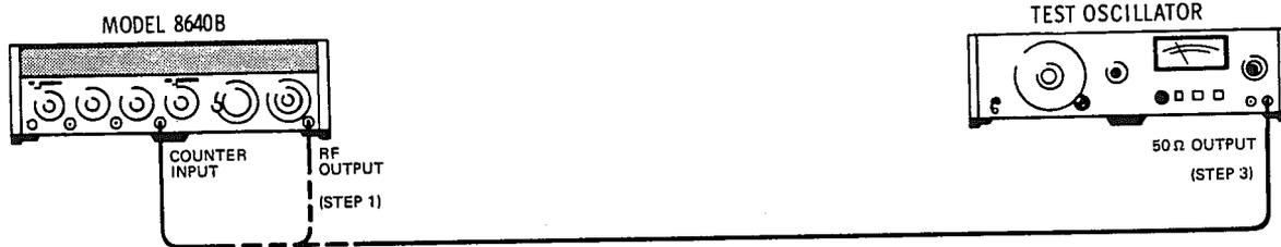
Figure 4-28. Counter External Sensitivity Test Setup
