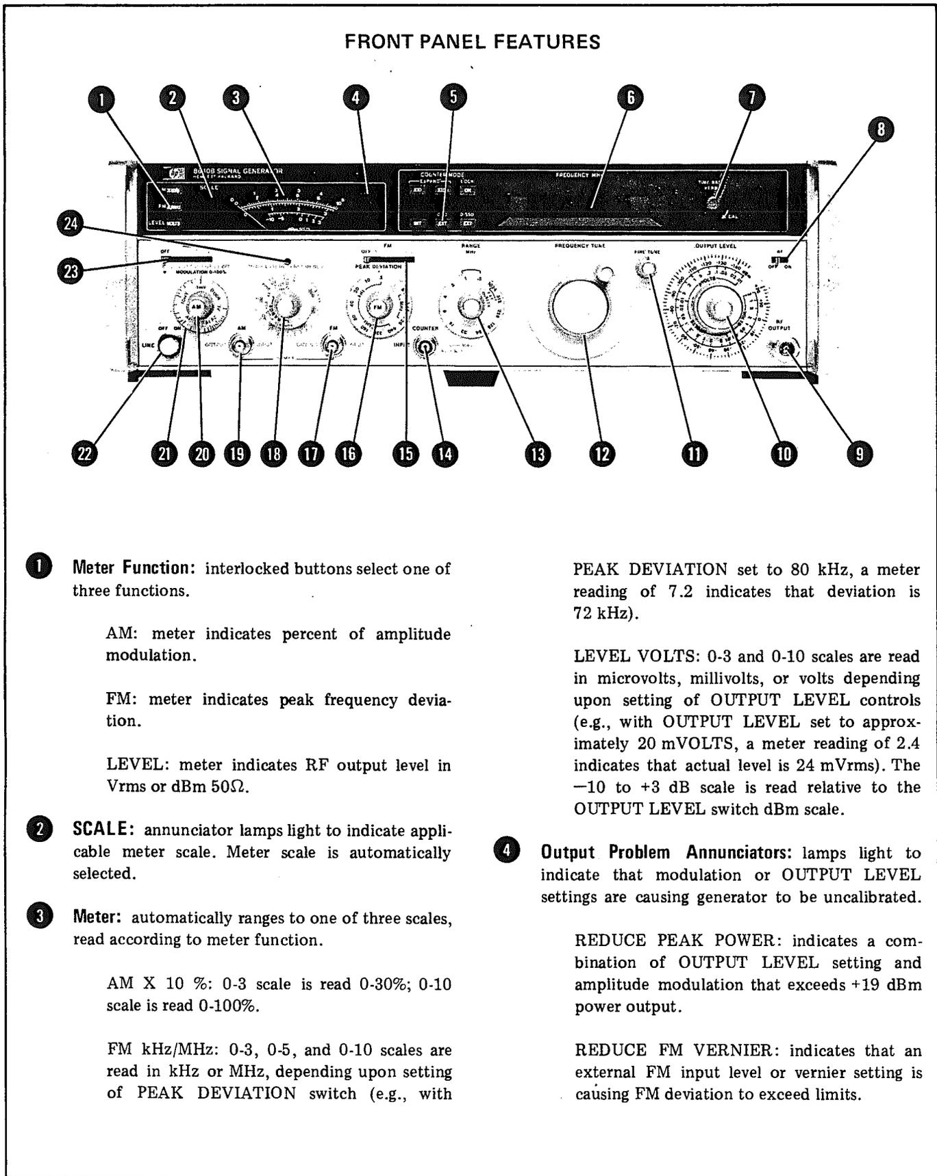
**1 Meter Function:** interlocked buttons select one of three functions.
