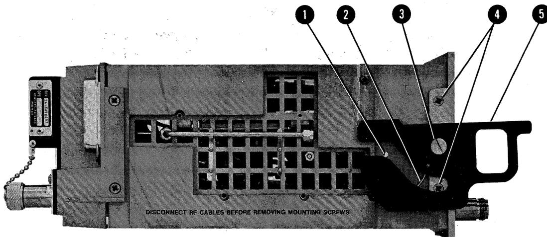
Figure 3-13. Band Indicator Lamp Replacement (1 of 2)
