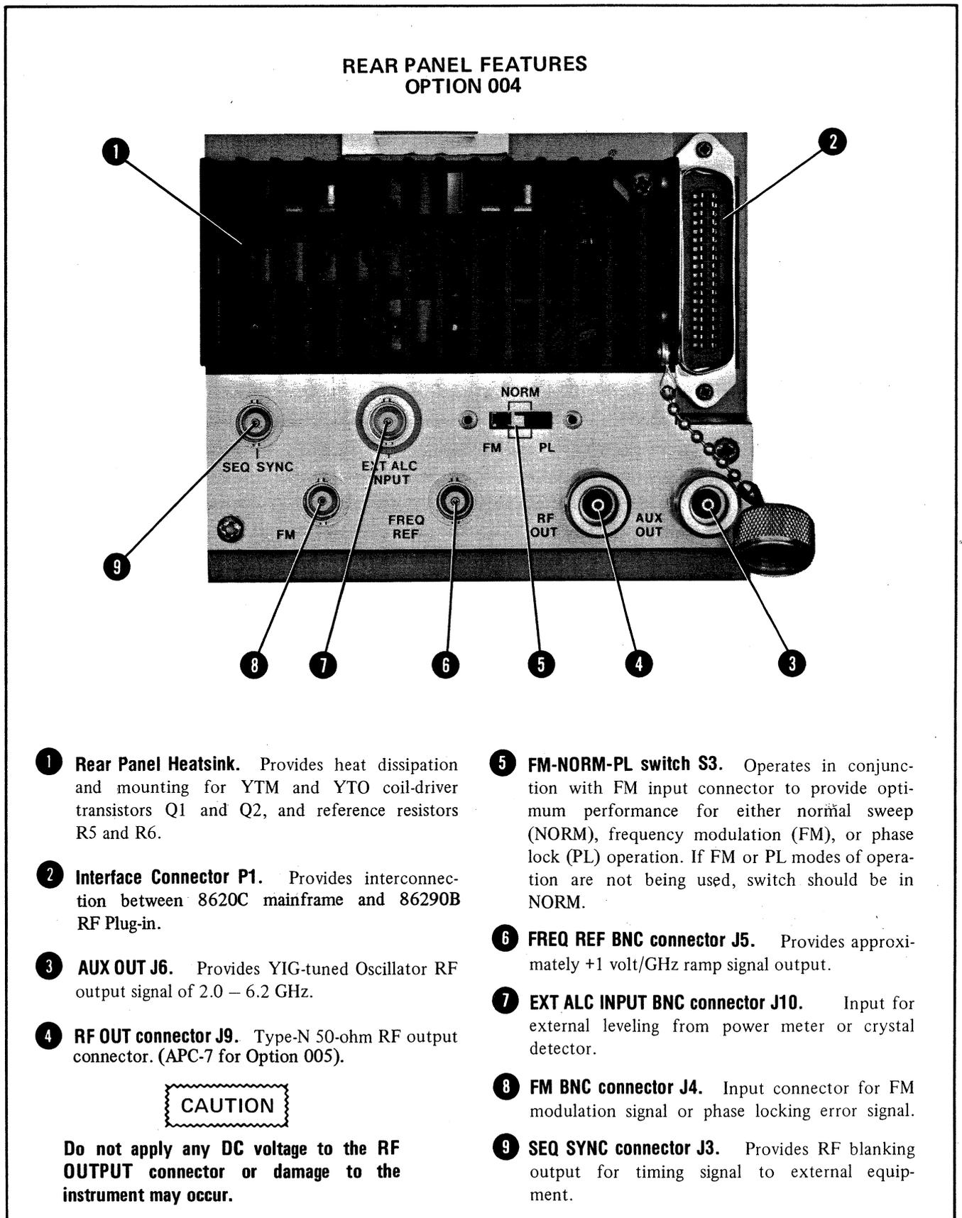
Figure 3-3. Rear Panel Connectors and Switch (2 of 2), Option 004
