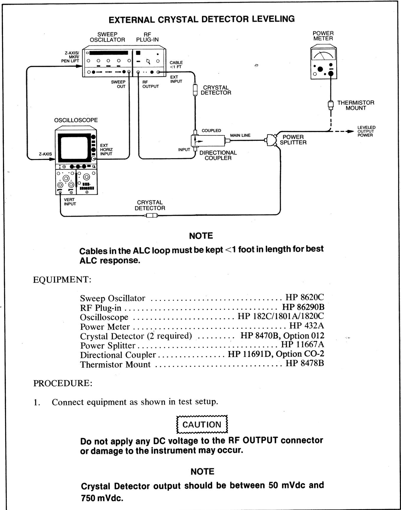
Figure 3-11. External Crystal Detector Leveling (1 of 2)
