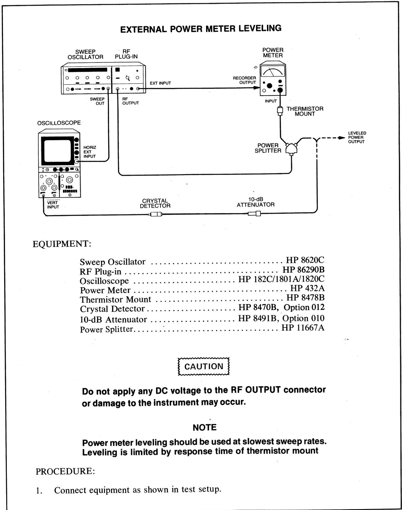
Figure 3-10. External Power Meter Leveling (1 of 2)
