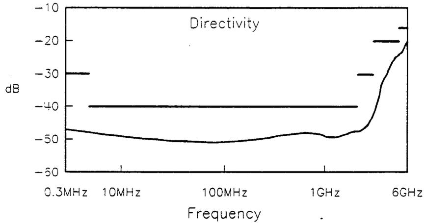
**Figure 1-1. Example Plot of HP 86205A Directivity**
