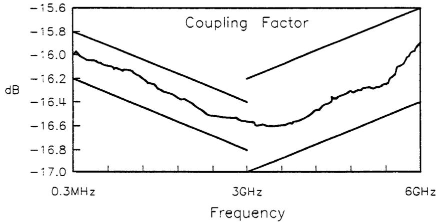
**Figure 1-3. Example Plot of HP 86205A Coupling Factor**
