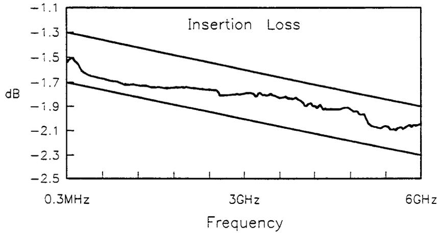
**Figure 1-2. Example Plot of HP 86205A Insertion Loss**
