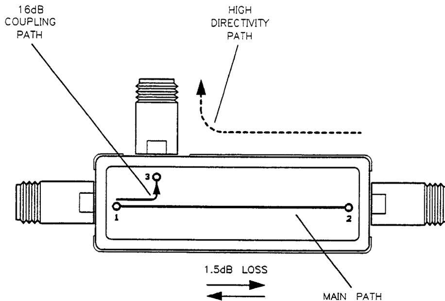
Figure 2-1. HP 86205A Bridge Ports and Measurement Paths
