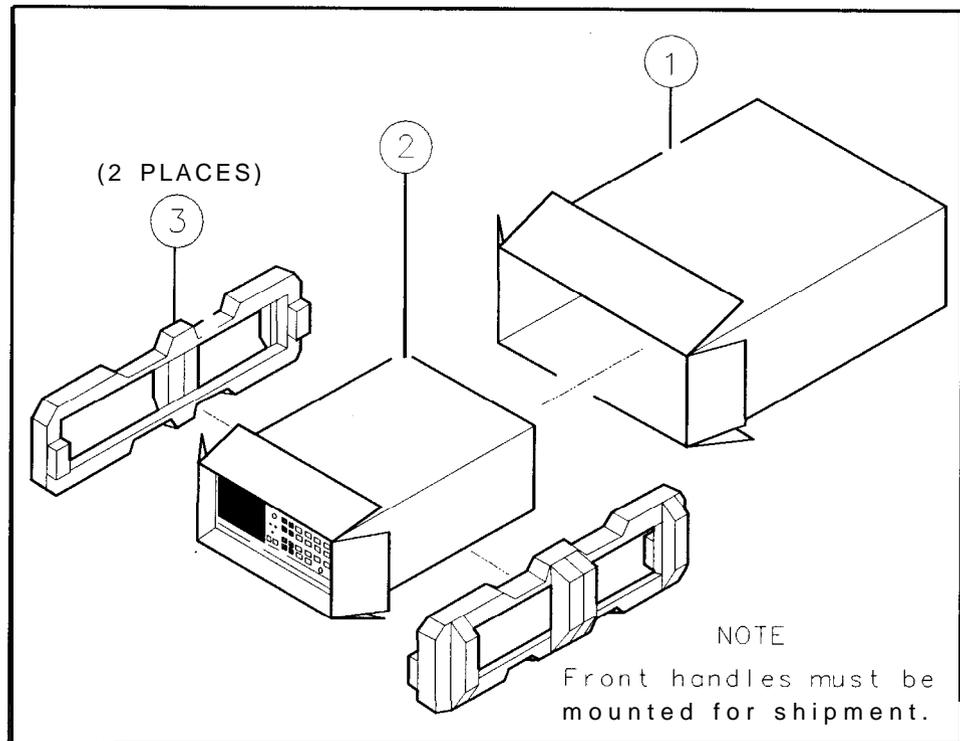
**Figure I-9. Factory Packaging Materials for Each Section**
