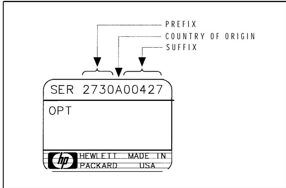
**Figure 1-3. Typical Serial Number Label**
