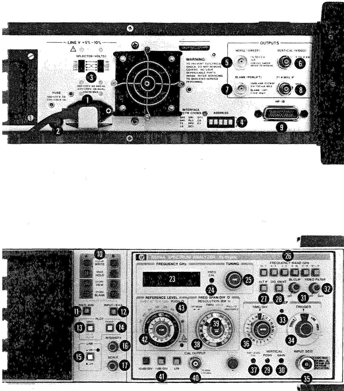
FIGURE 3-1. HP 8559A/853A CONTROLS, CONNECTORS, AND INDICATORS
