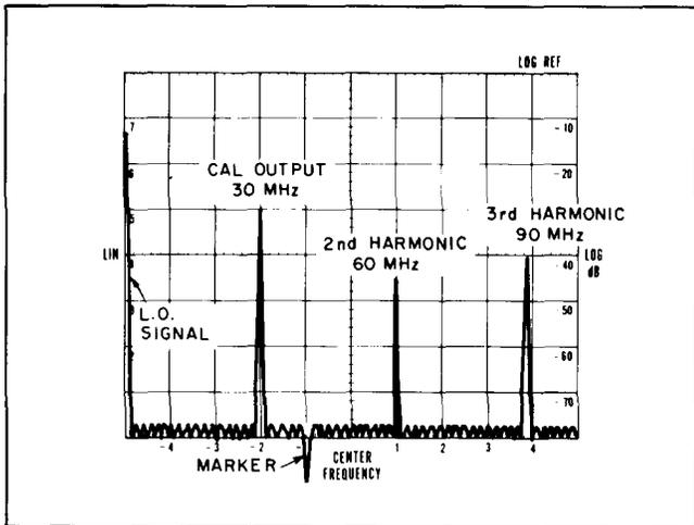
Figure 4-1. 30 MHz Calibrator Signal & Harmonics
