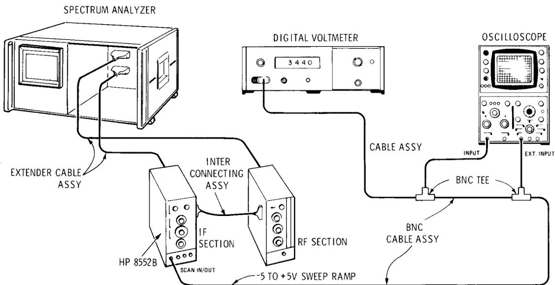
*Figure 5-2. Scan Generator Check and Adjustment Test Setup*
