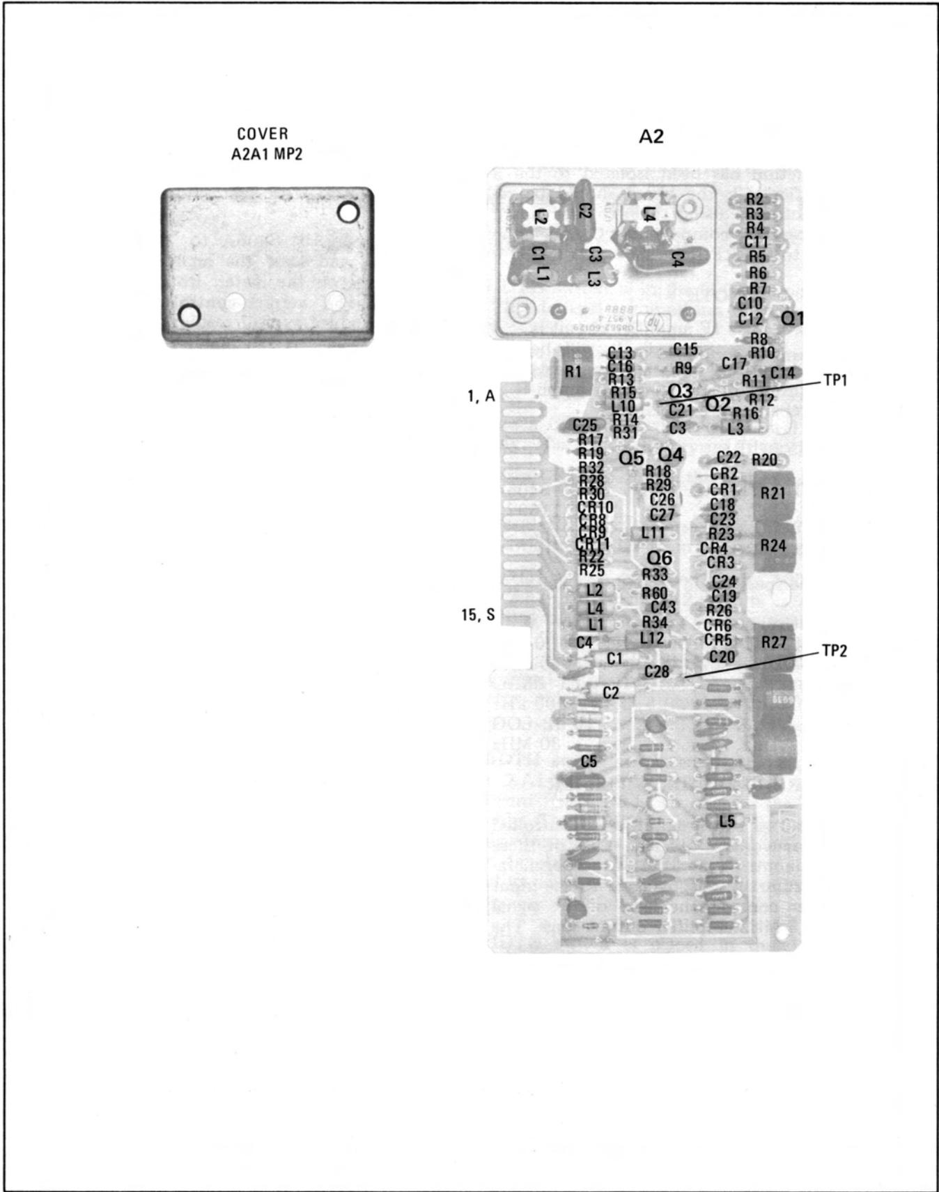
Figure 8-24. P/O 3 MHz Amplifier A2 Component Identification
