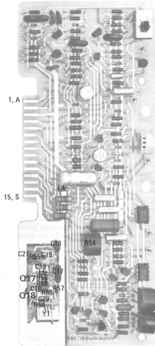
Figure 8-48. P/O Scan Generator A6 Component Identification
