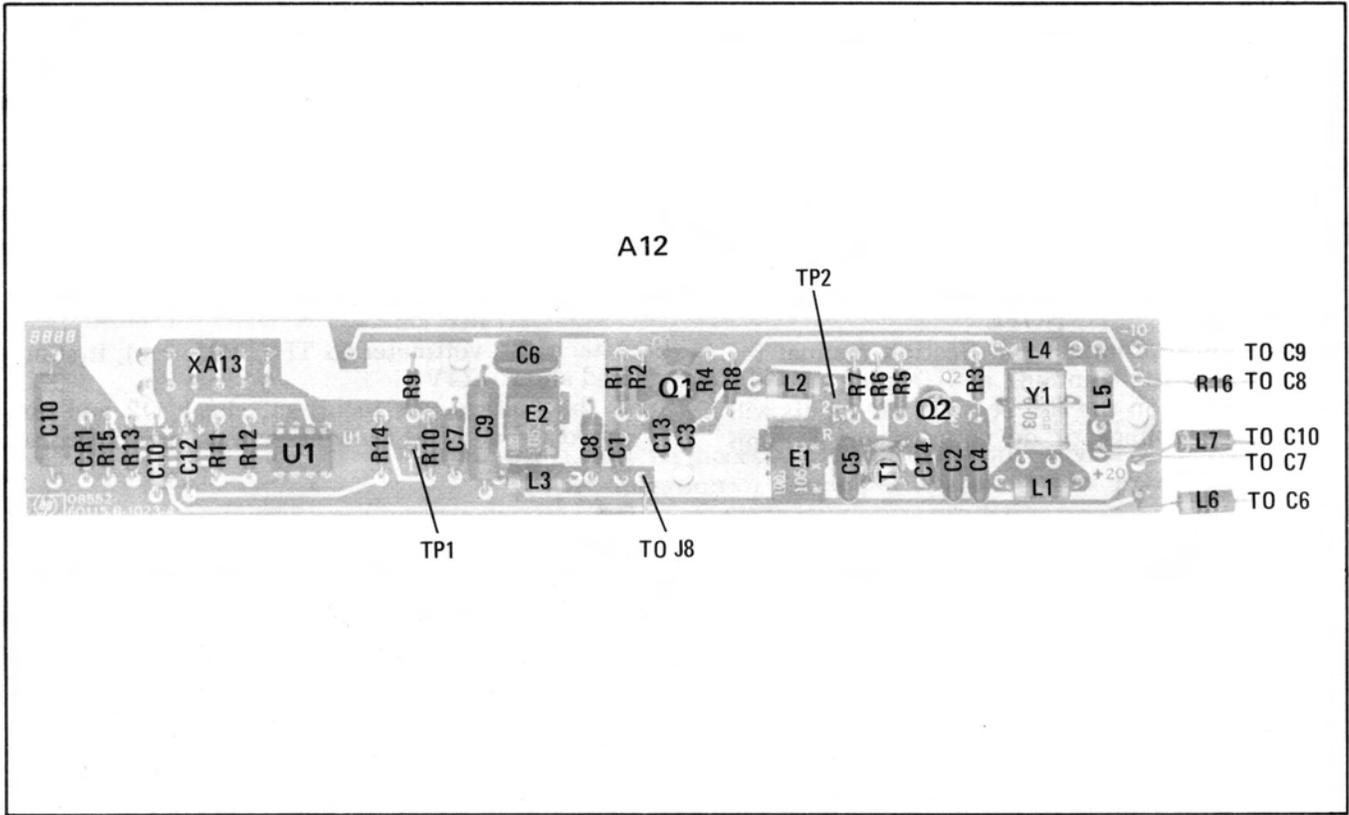
Figure 8-19. 47 MHz APC A12 Component Identification
