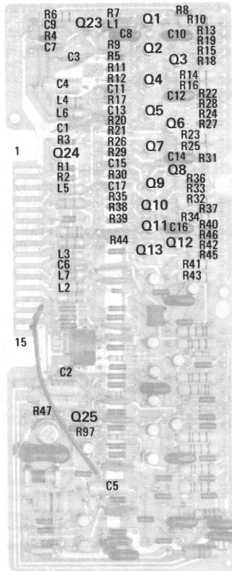
Figure 8-36. P/O Log/Linear Amplifier A8 Component Identification
