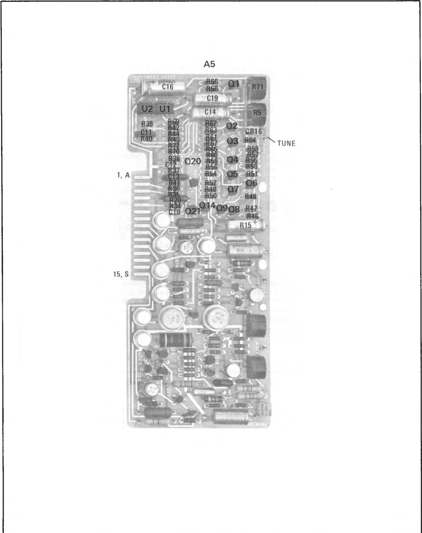
Figure 8-22. P/O Power Supply A5 Component Identification
