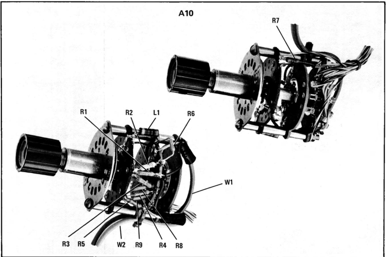
Figure 8-12. Log Reference Level Switch Assembly A10
