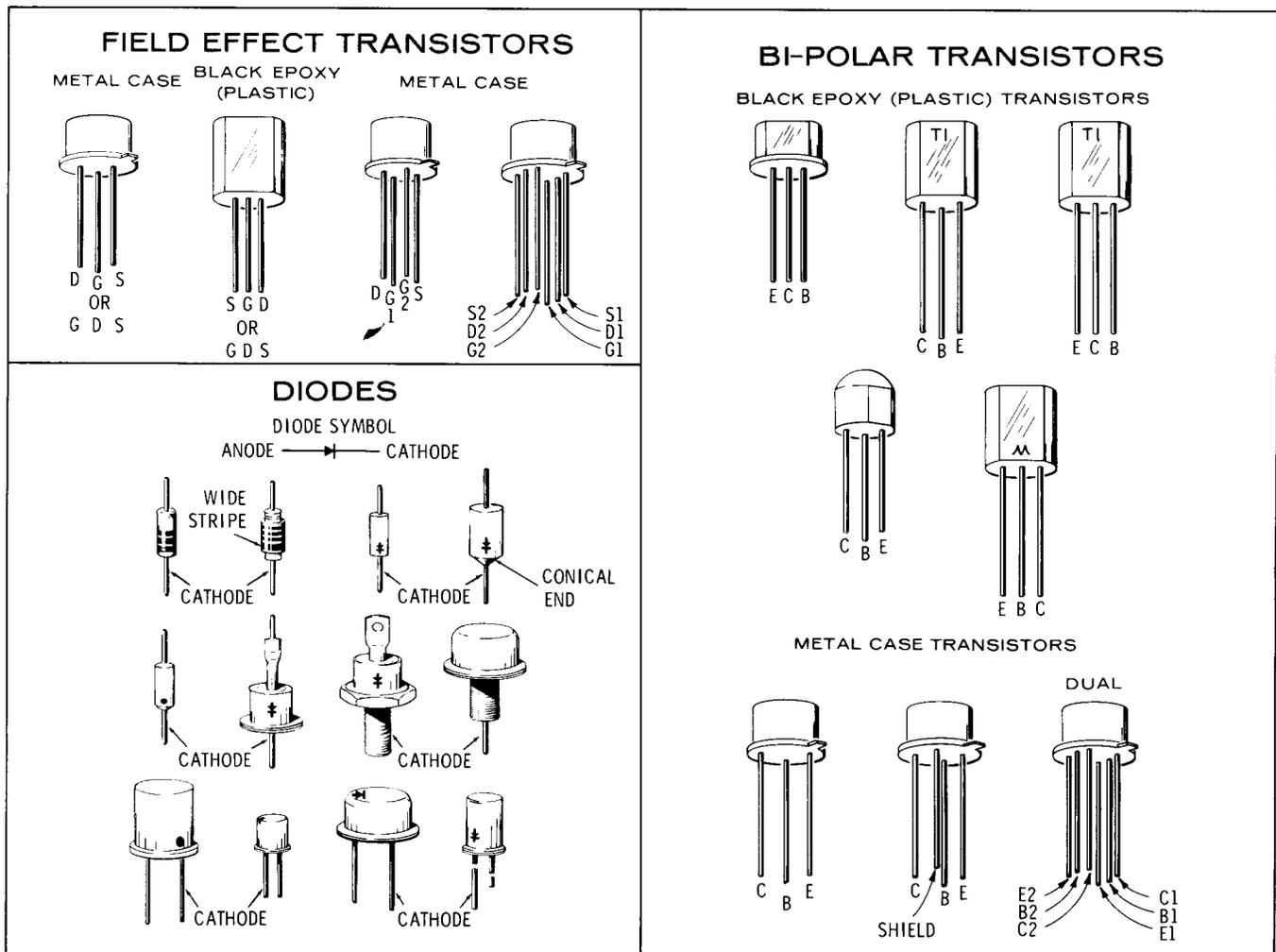
Figure 8-3. Examples of Diode and Transistor Marking Methods
