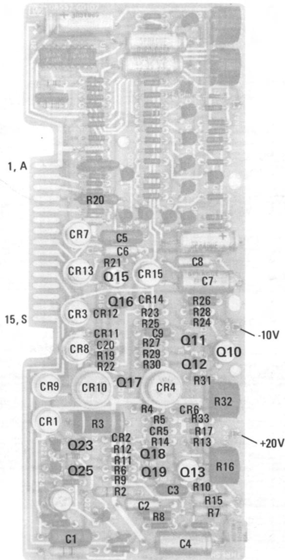
Figure 8-50. P/O Power Supply A5 Component Identification
