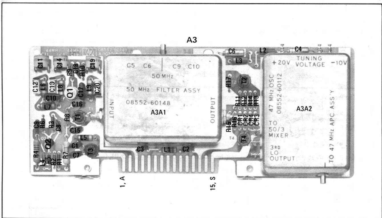
Figure 8-17. 50 MHz Converter A3 Component Identification
