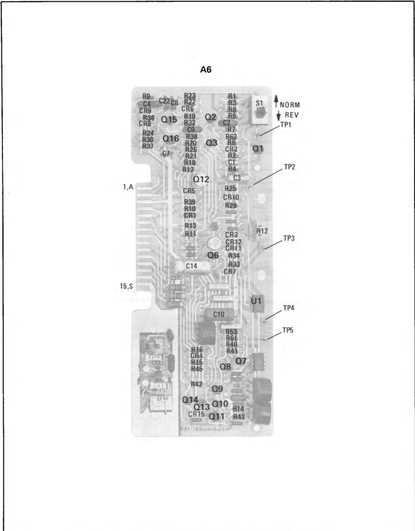
Figure 8-42. P/O Scan Generator A6 Component Identification
