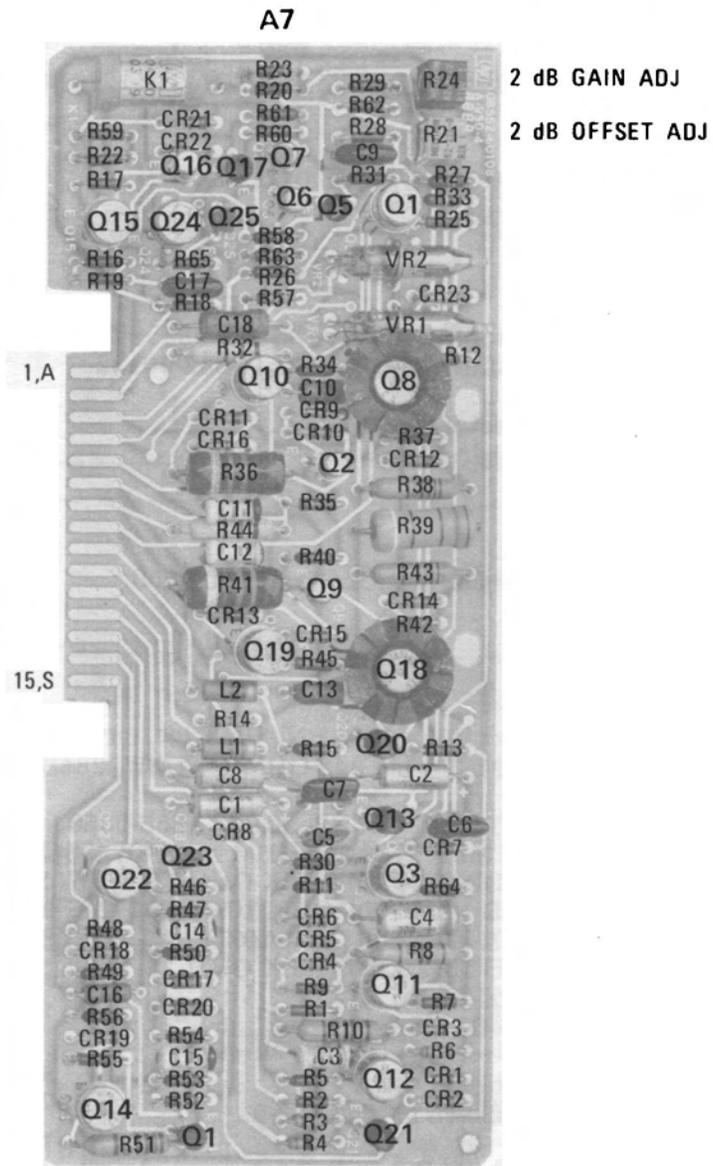
Figure 7-6. Deflection Amplifier A7 Component Identification (Part of Change O)
