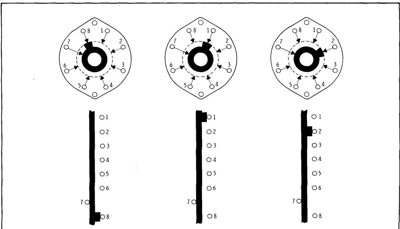
Figure 8-6. Three Positions of Typical Switch Wafers
