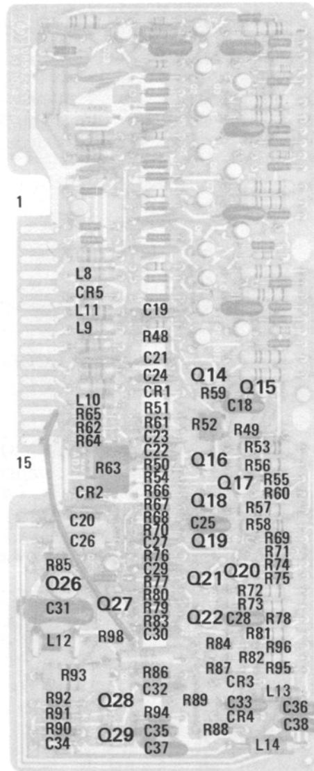
Figure 8-38. P/O Log/Linear Amplifier A8 Component Identification
