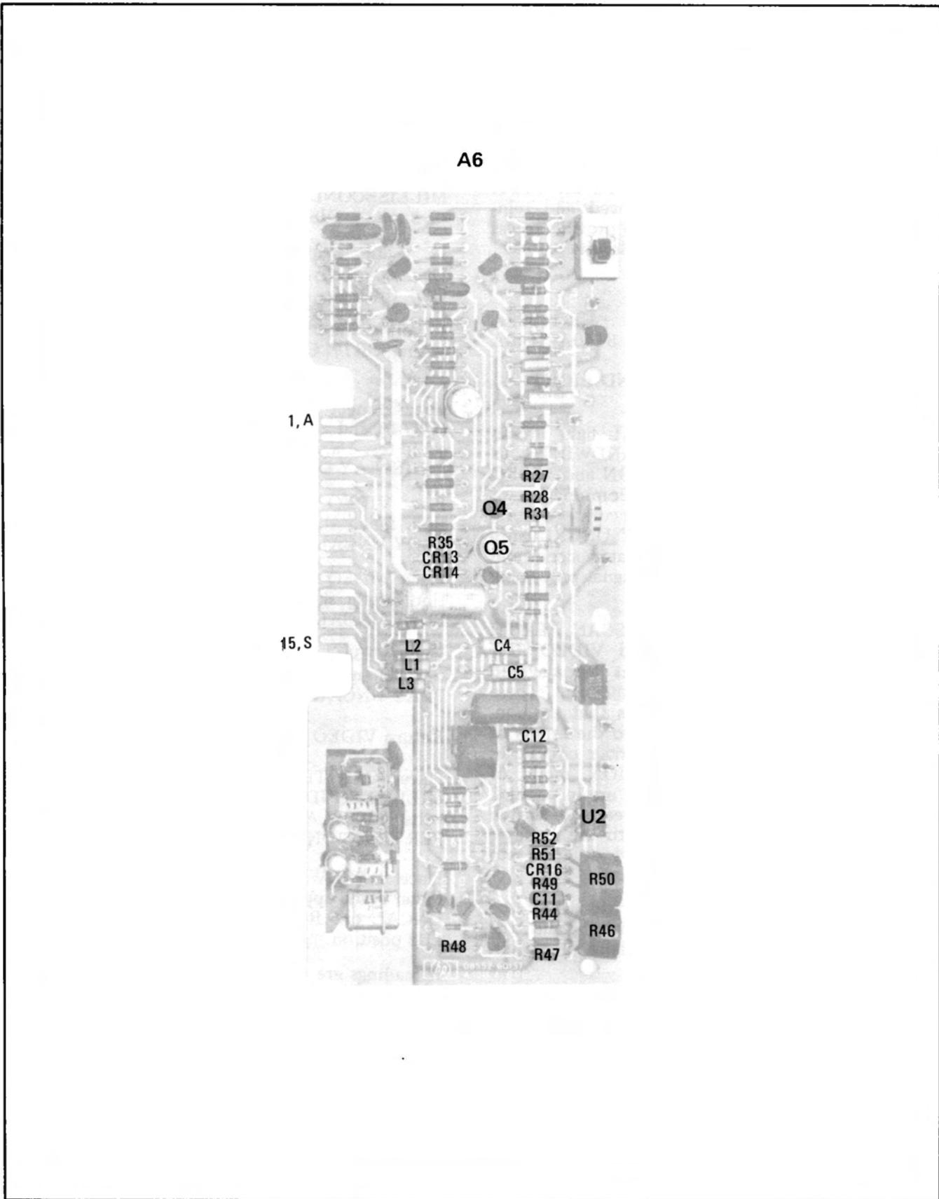
Figure 8-44. P/O Scan Generator A6 Component Identification
