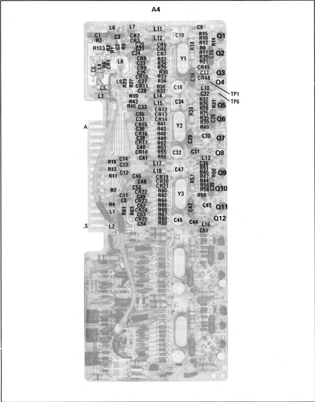
Figure 8-31. P/O Crystal Filter A4 Component Identification
