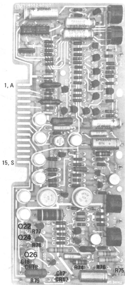
Figure 8-46. P/O Power Supply A5 Component Identification
