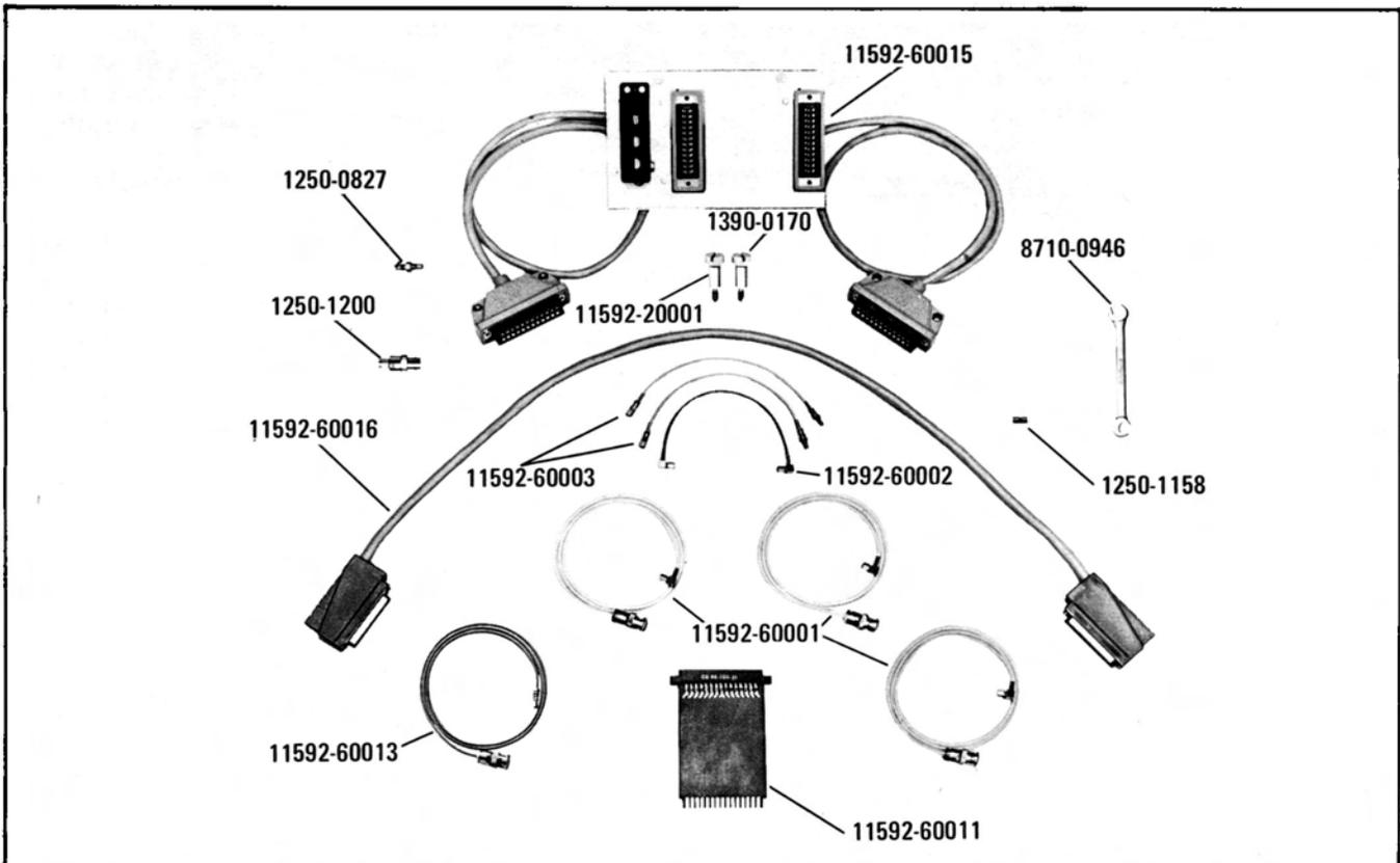
Figure 1-2. HP 11592A Service Kit Required for Maintenance
