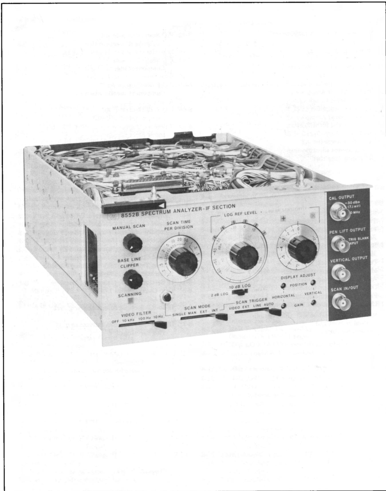
Figure 1-1. Model 8552B Spectrum Analyzer IF Section
