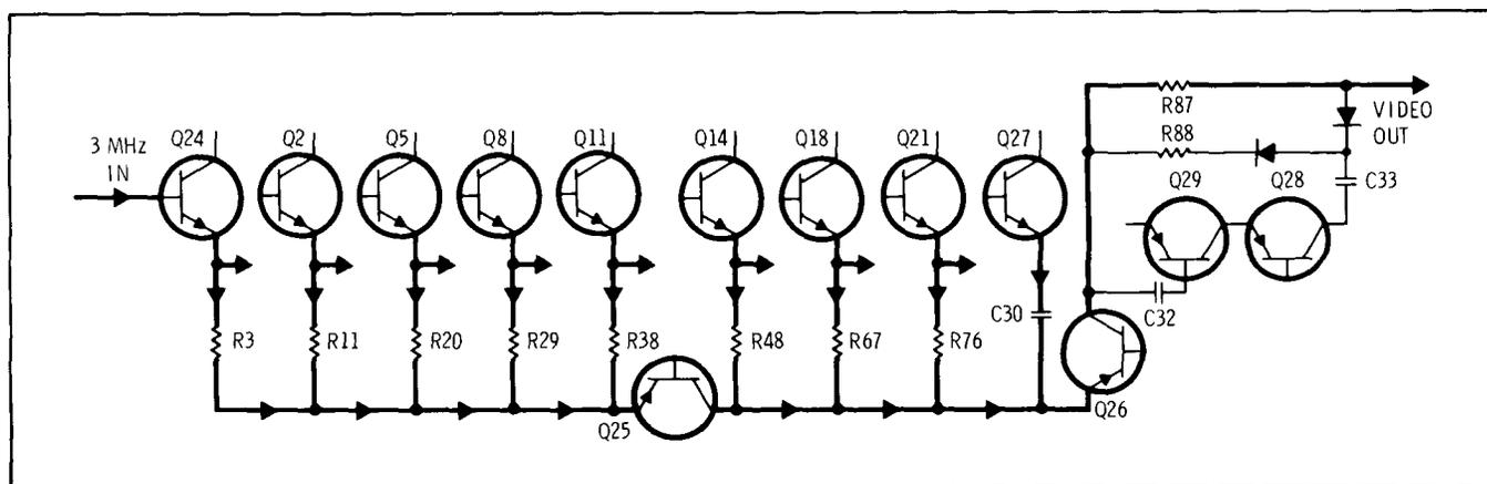
Figure 8-35. Simplified Diagram — Log Mode of Operation
