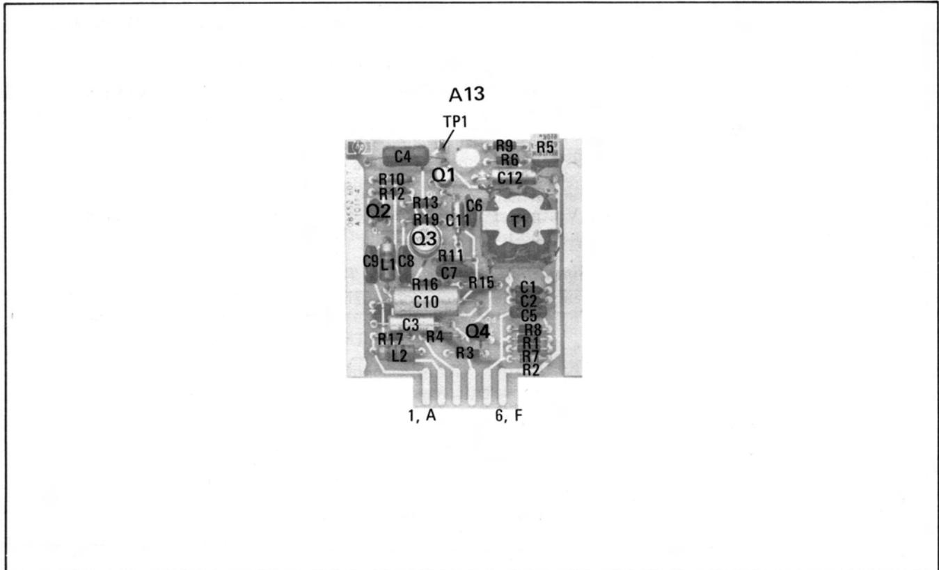
Figure 8-20. 2 MHz VTO A13 Component Identification
