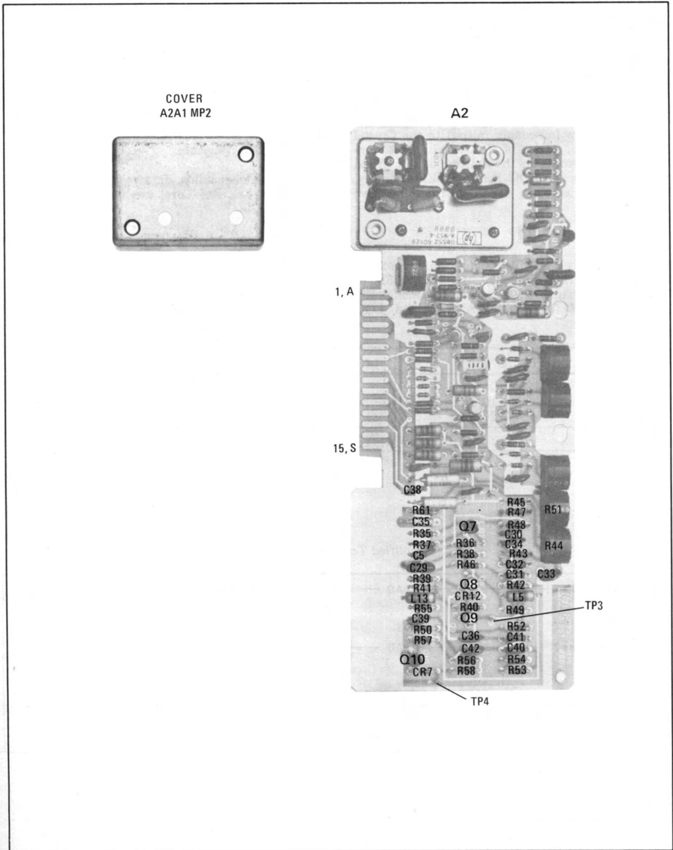
Figure 8-26. P/O 3 MHz Amplifier A2 Component Identification
