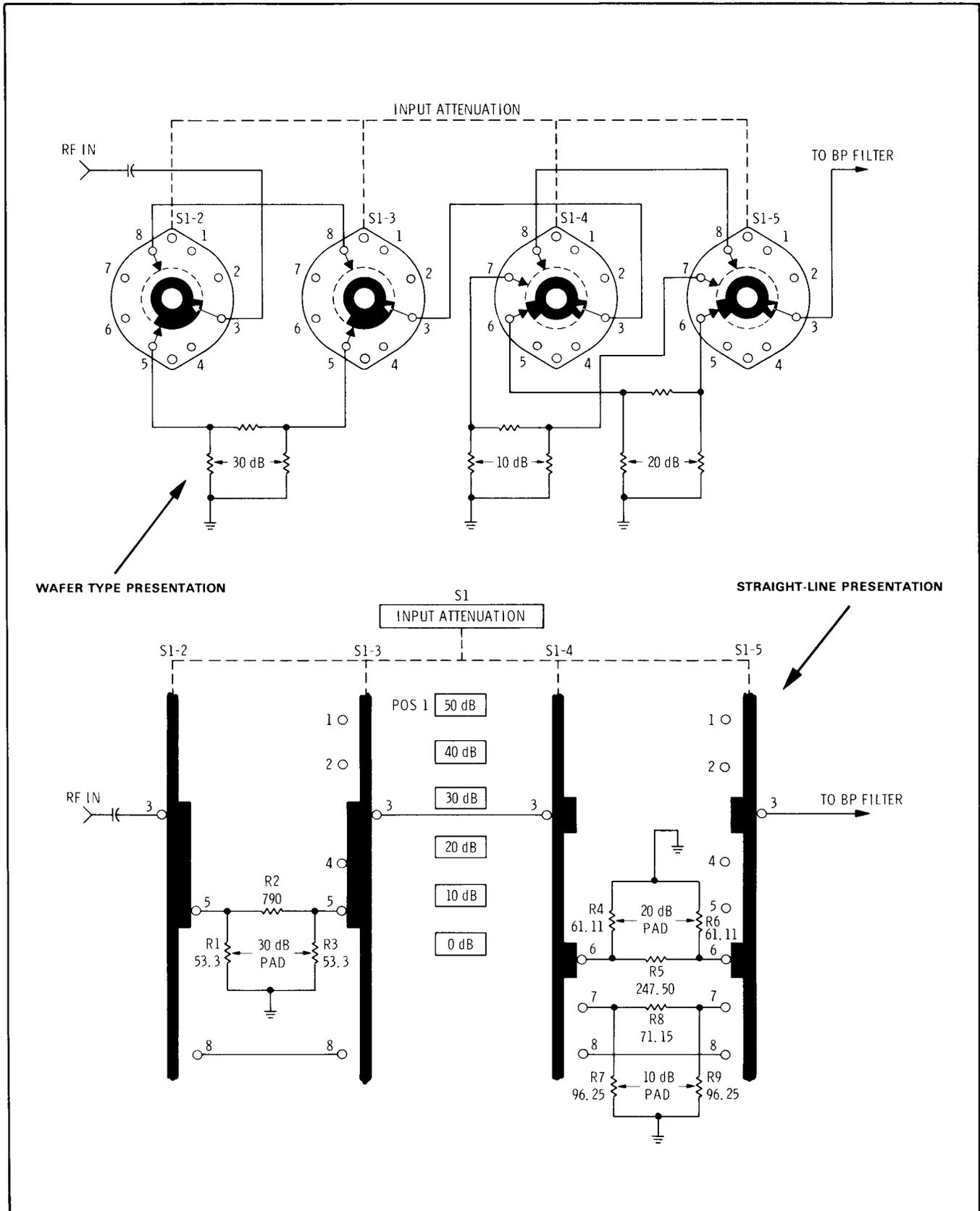
Figure 8-7. Wafer Switch Presentation Versus Straight-Line Presentation
