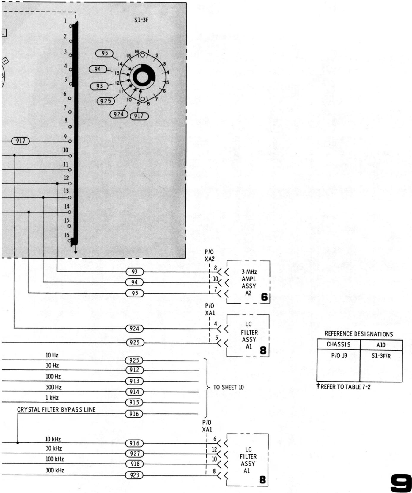
Figure 8-30. Amplifier/Filter Control Circuits
