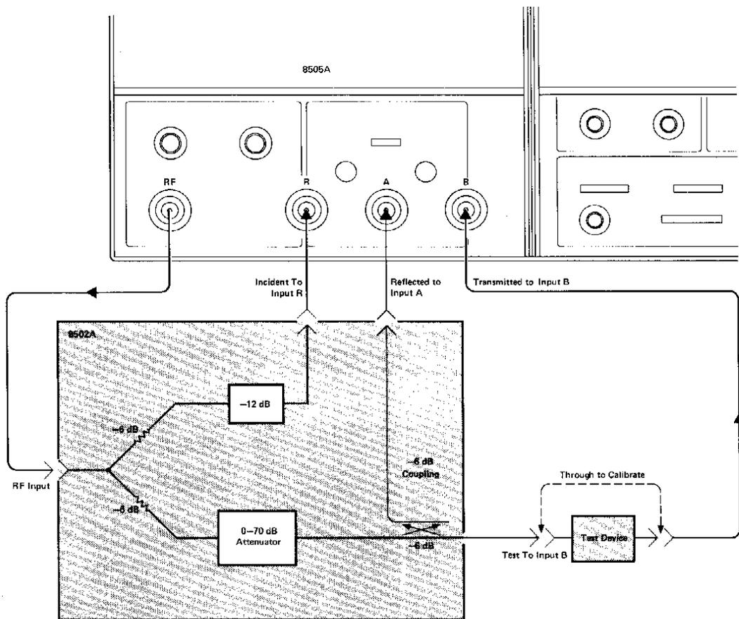
Connections to the test set and test device are made using the cables supplied in the 11851A Cable Kit. The test device input port is connected to the 8502 front panel TEST connector. For transmission calibration, the cable which connects to the device output is connected to the 8502 TEST output. Whatever configuration is used, all cables, adapters, and fixtures required for the measurement should also be used for calibration.
