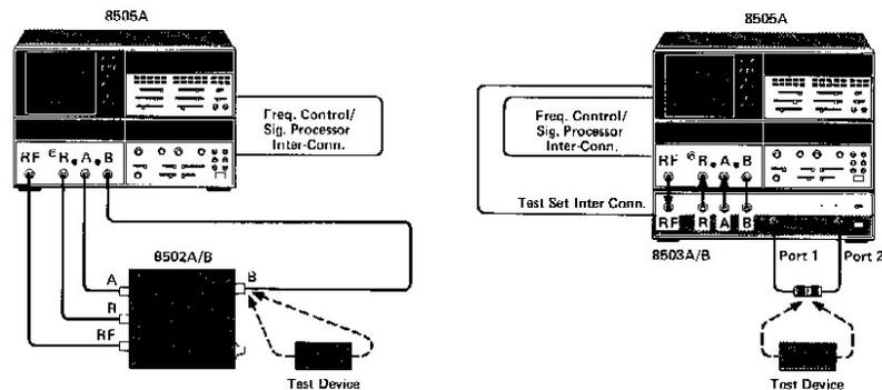
**Set Signal Levels** — Set the INPUT LEVEL dBm MAX switch to  $-10$ . Use the OUTPUT LEVEL dBm and VERNIER to set the approximate signal levels to the test device. (Refer to the Power Level Measurements sequence on page 25 to measure the absolute power, if necessary.)
