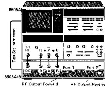
The 8503A front panel FORWARD/REVERSE control switches the incident RF to Port 1 for FORWARD or Port 2 for reverse. These illustrations show the functions of the 8505A R, A, and B connections in FORWARD and REVERSE.
