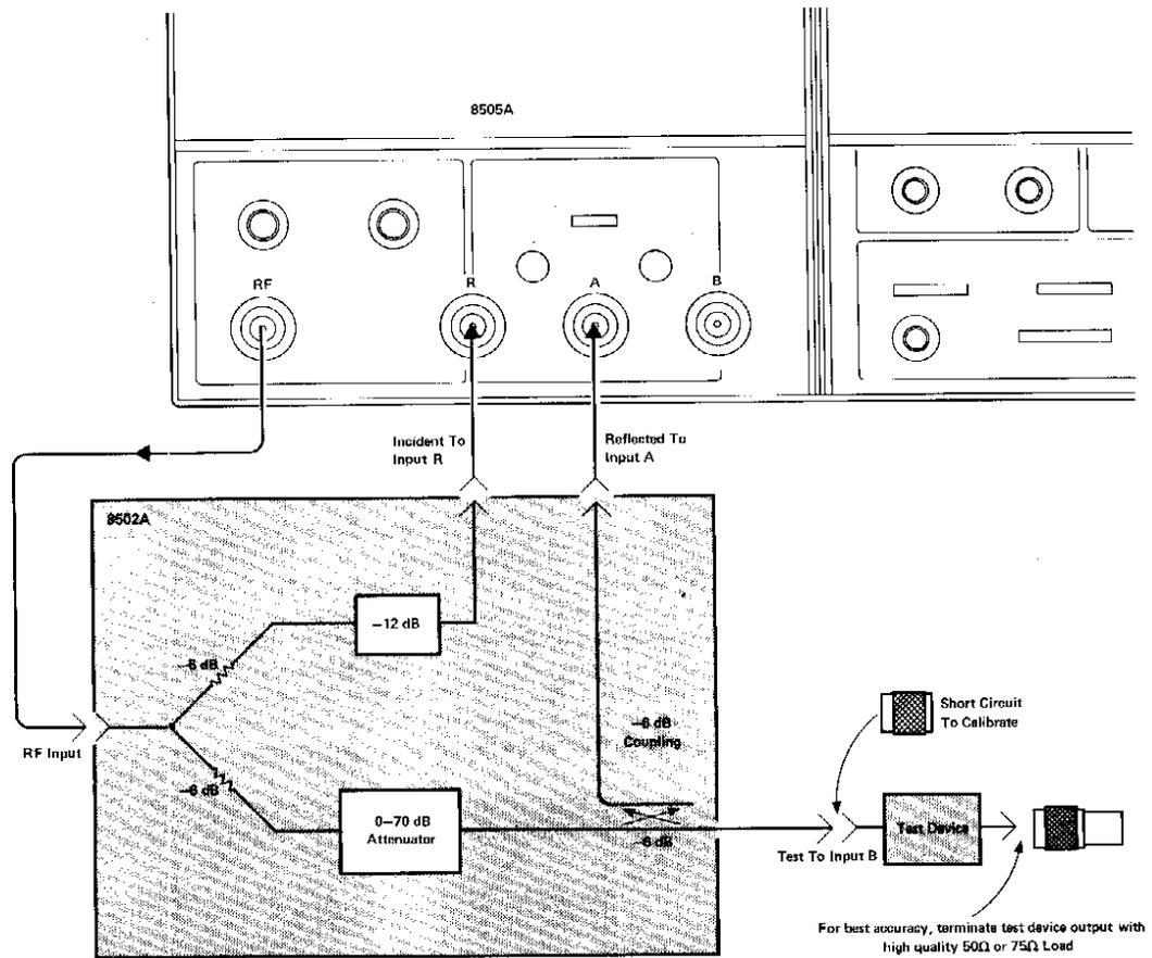
Connections to the test set and test device are made using the cables supplied in the 11851A Cable Kit. The test device input port is connected to the 8502 front panel TEST connector. For reflection calibration, connect the short circuit at the same point to which the test device will be connected. Whatever configuration is used, all cables, adapters, and fixtures required for the measurement should also be used during calibration.
