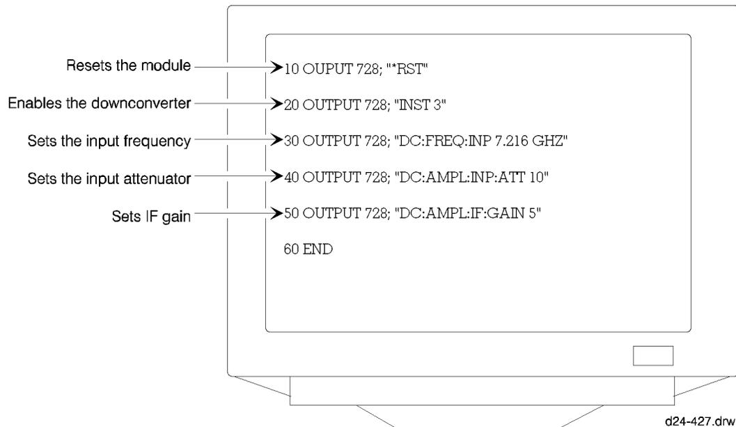
**Figure 2-26** *HP BASIC on an HP 9000 series 200/300 Controller*
