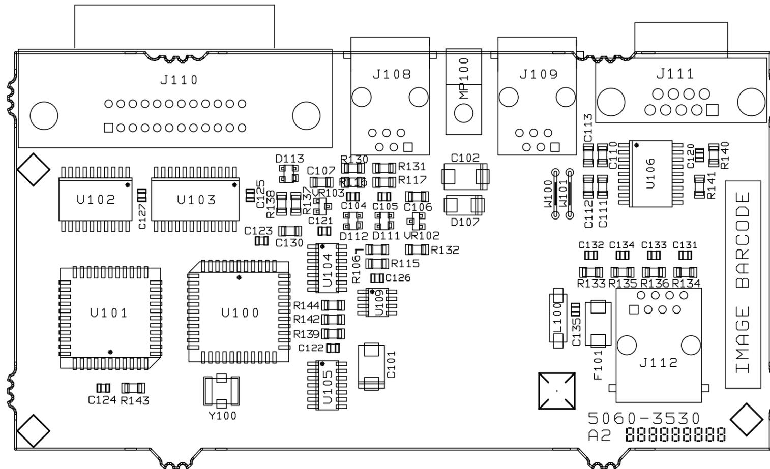
Figure 6-4. GPIB Assembly, Component Locations
