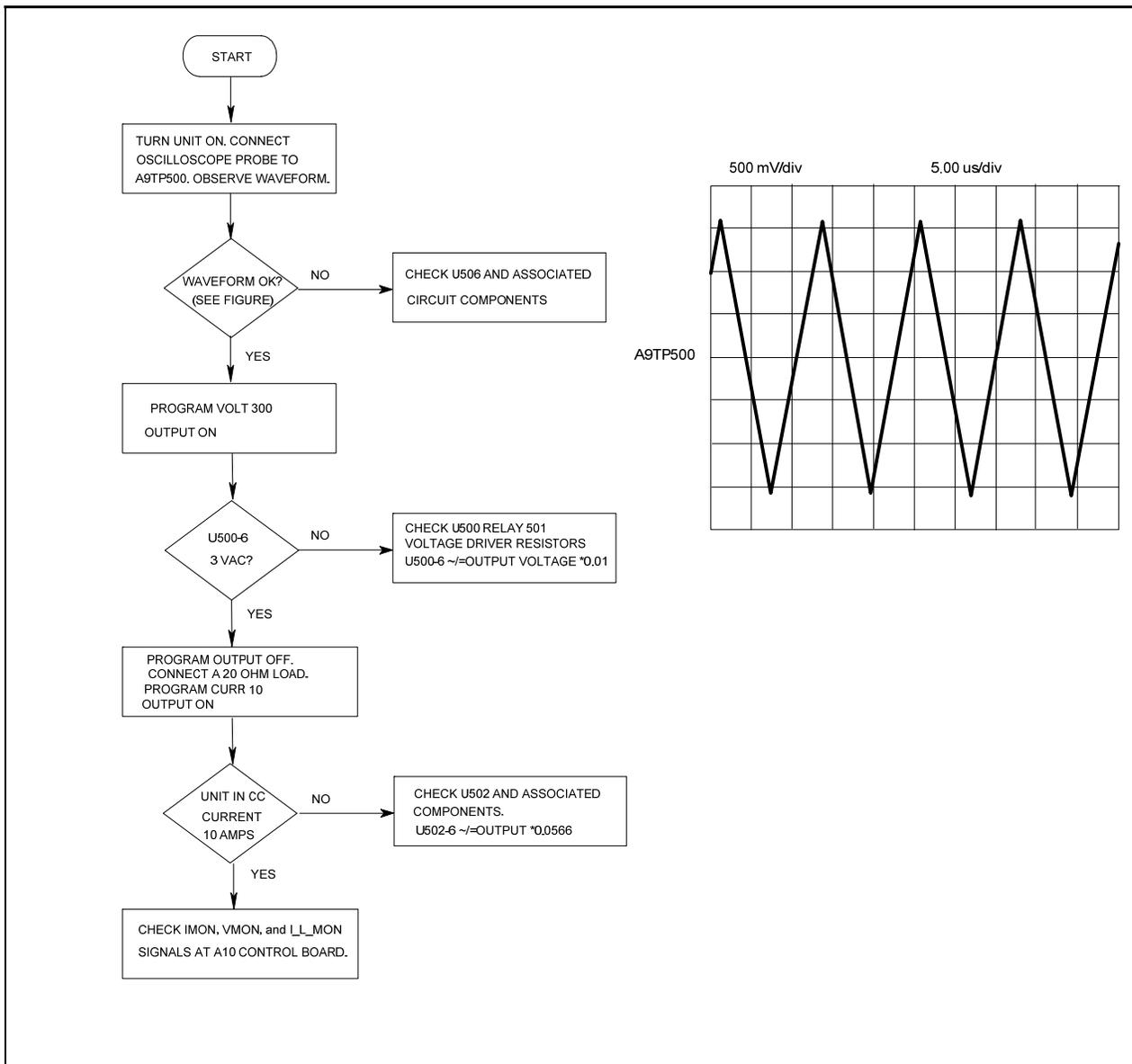
Figure 4-9. Output/Filter/Relay Troubleshooting
