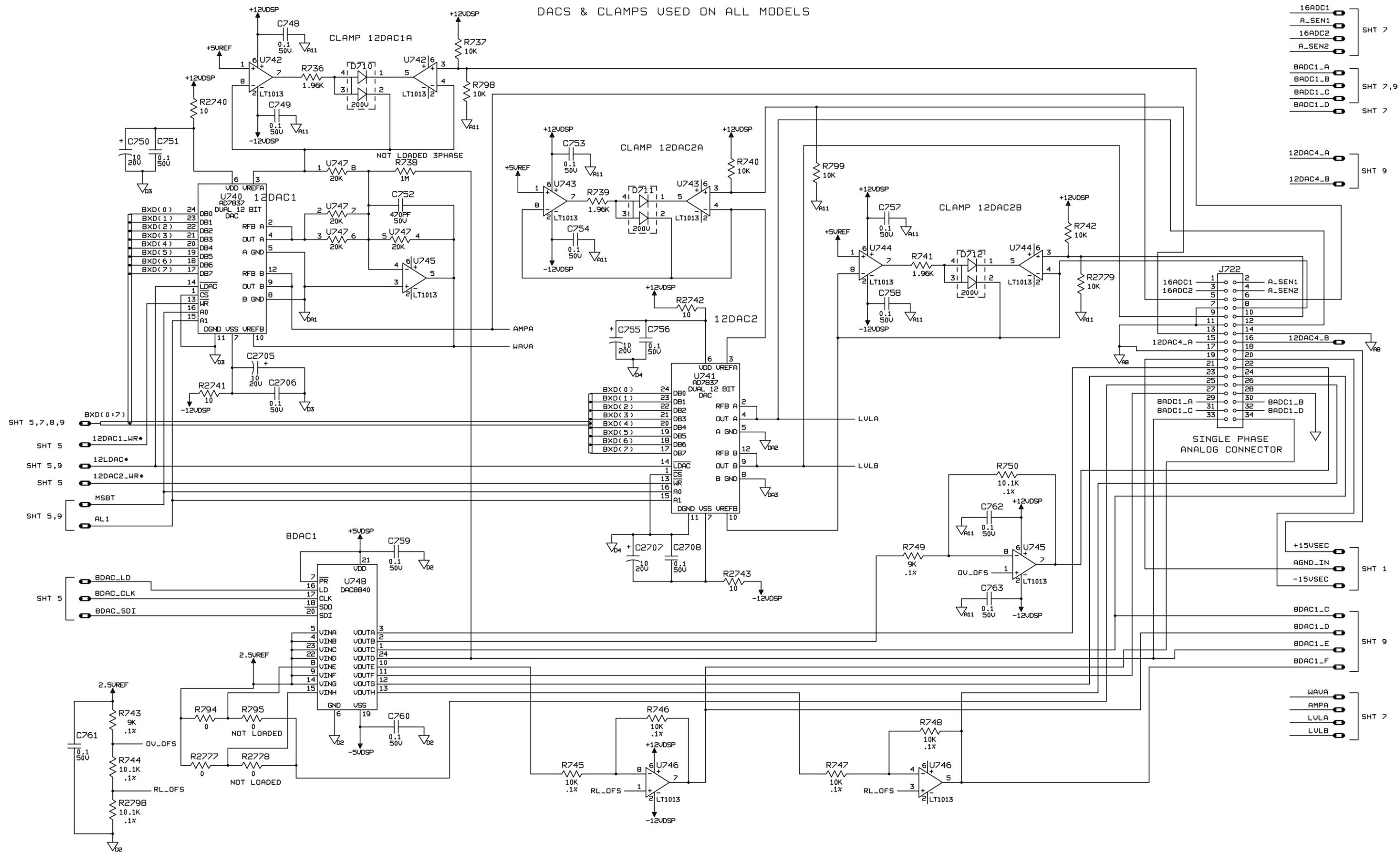
Figure 6-17. DSP Assembly, Schematic Diagram (sheet 6 of 10)
