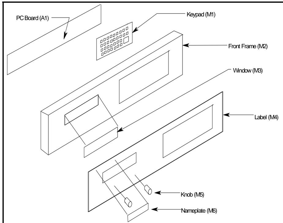
**Figure 5-1. Front Panel Components (see Table 5-1)**
