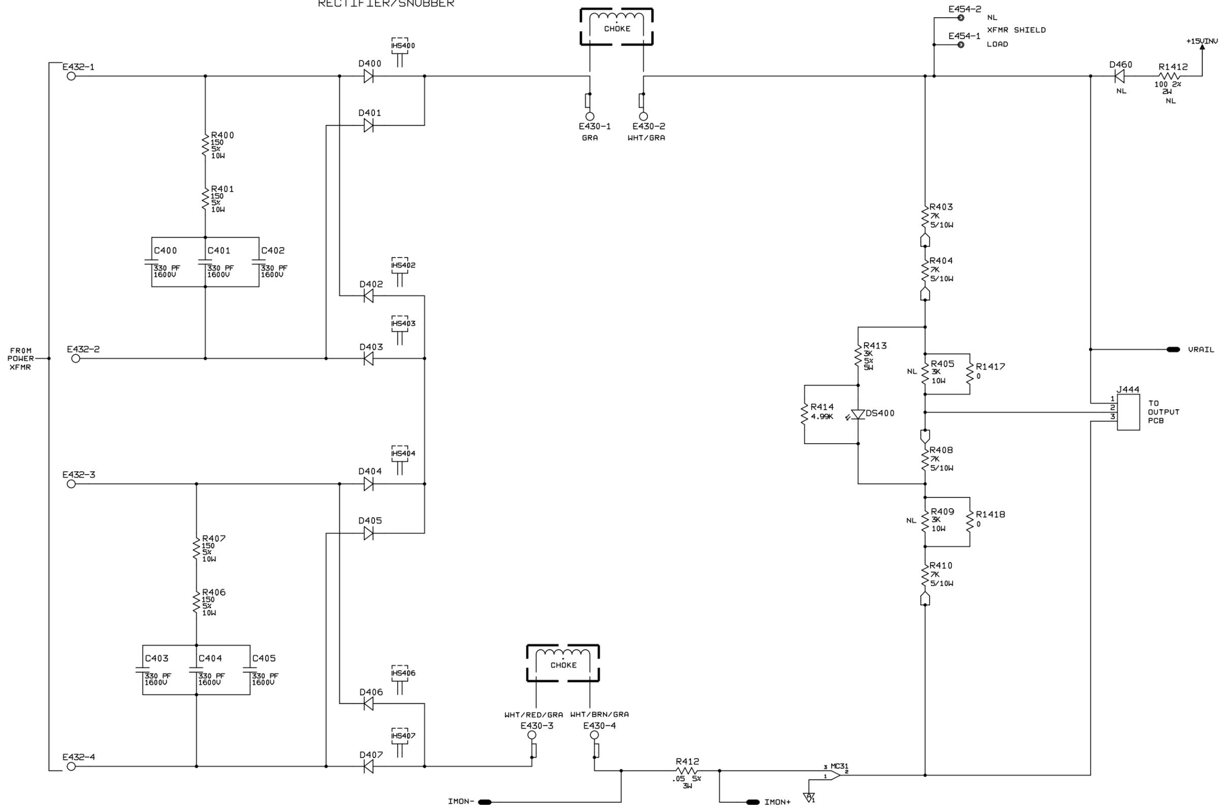
Figure 6-11. DC Rail/Diode Assembly, Schematic Diagram (sheet 1 of 3)
