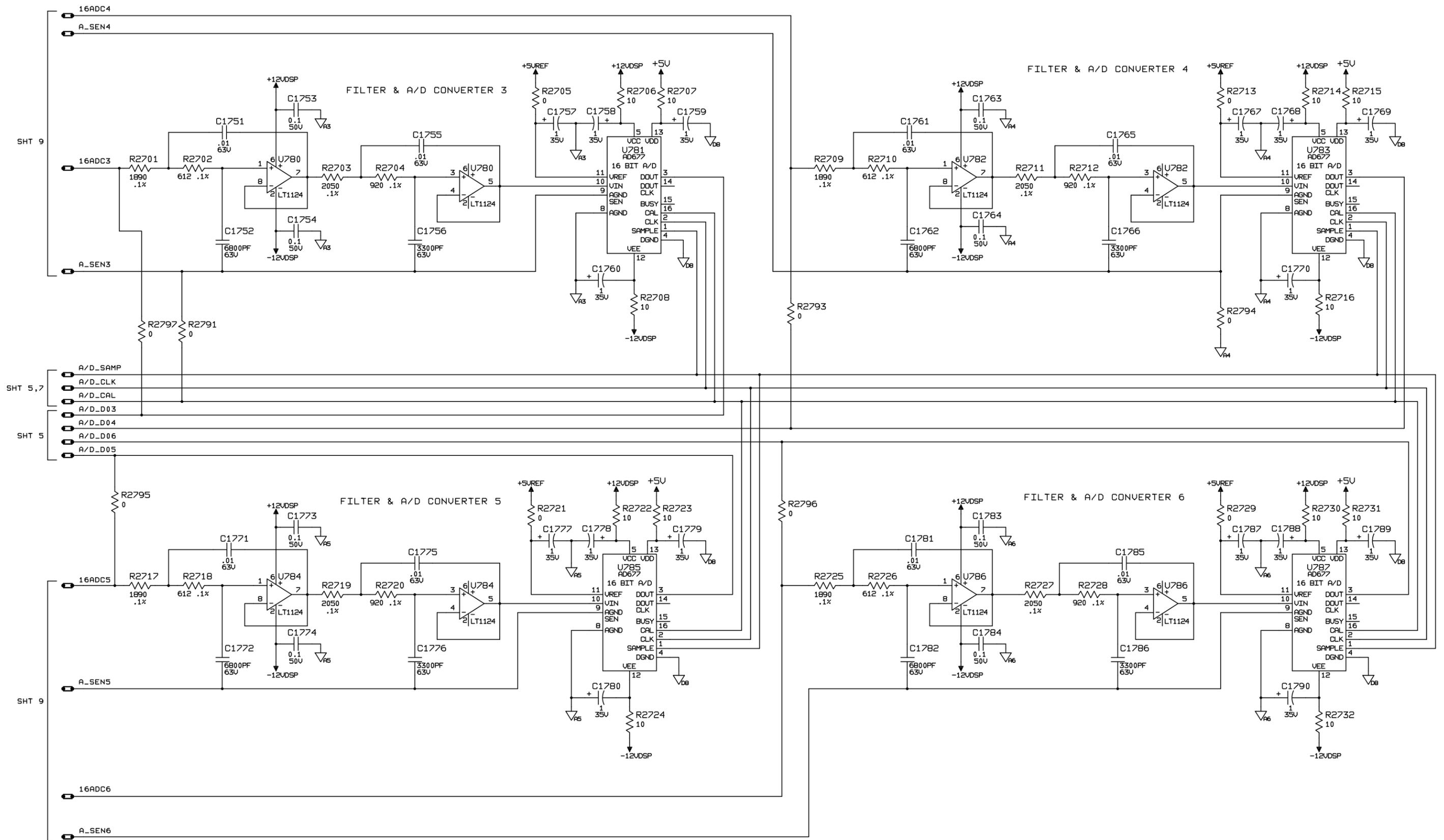
Figure 6-17. DSP Assembly, Schematic Diagram (sheet 10 of 10)
