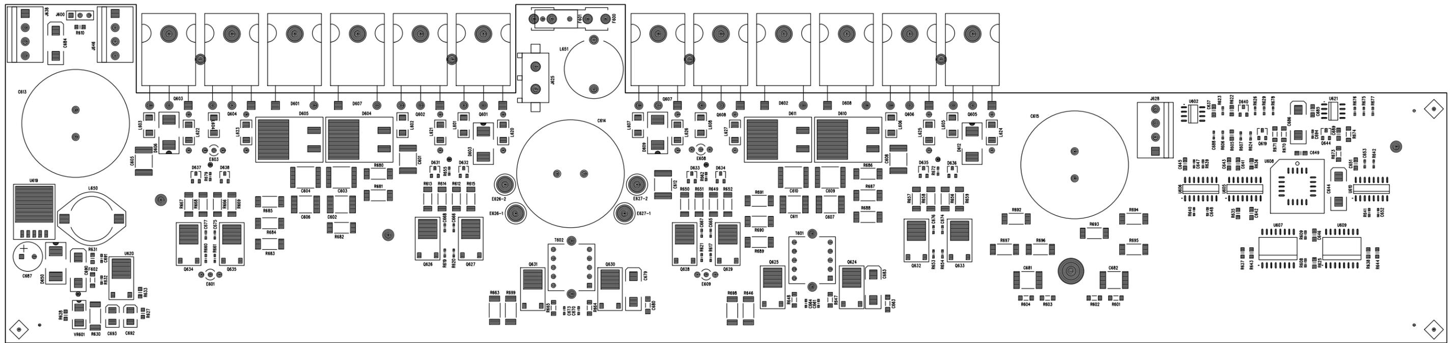
Figure 6-14. Inverter Assembly, Component Locations
