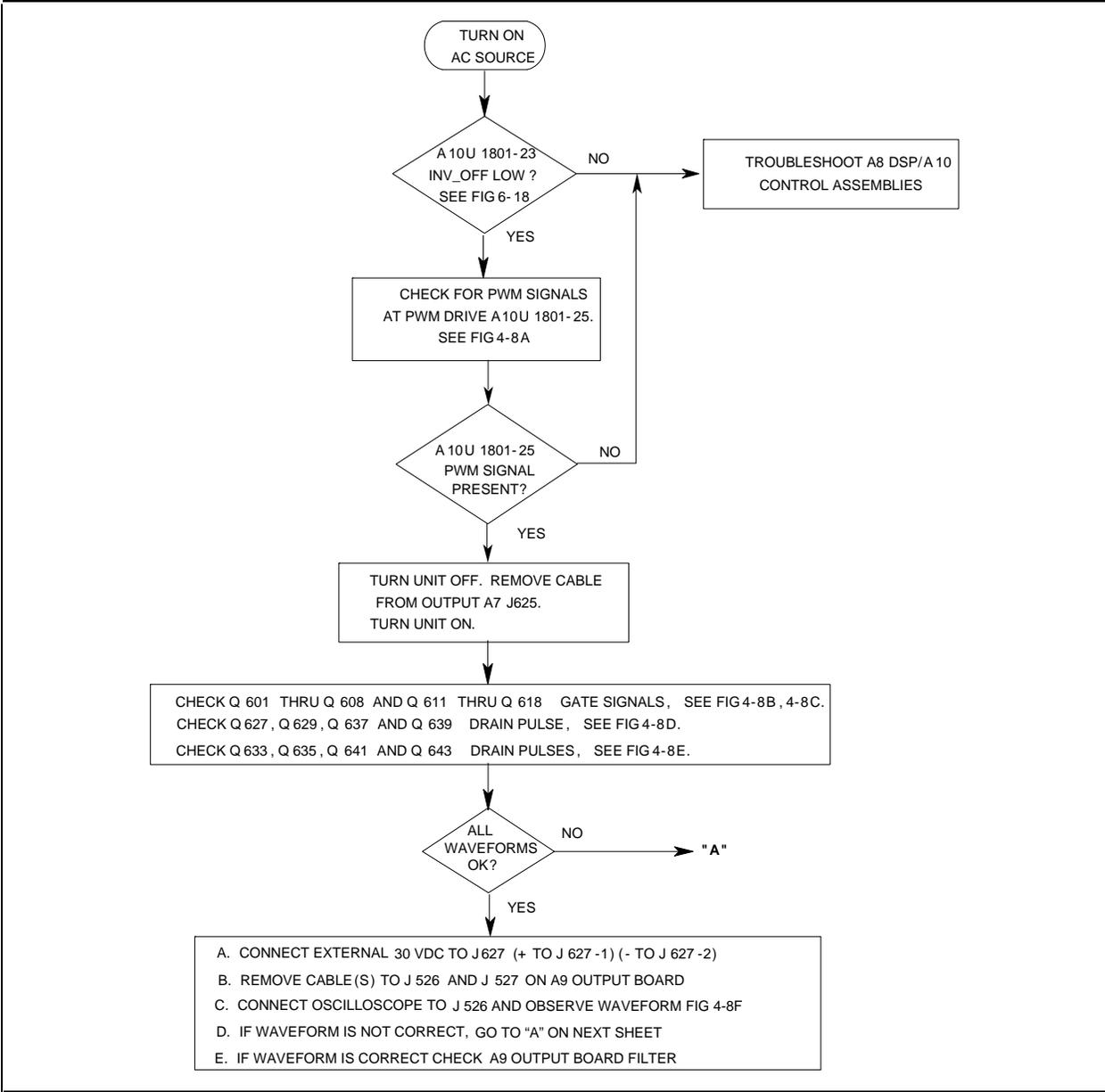
Figure 4-7. Inverter Assembly Troubleshooting (sheet 1 of 2)
