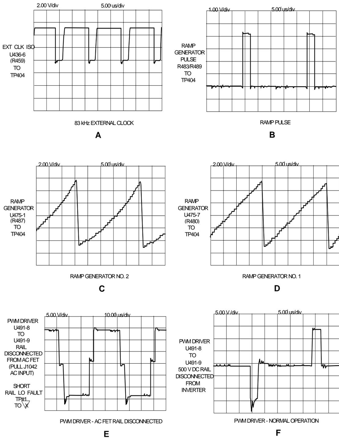
Figure 4-5. DC Rail Assembly - Test Waveforms
