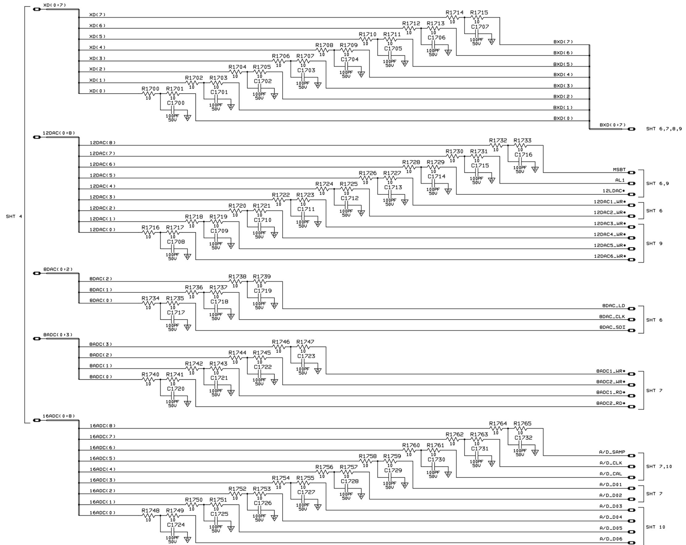
Figure 6-17. DSP Assembly, Schematic Diagram (sheet 5 of 10)
