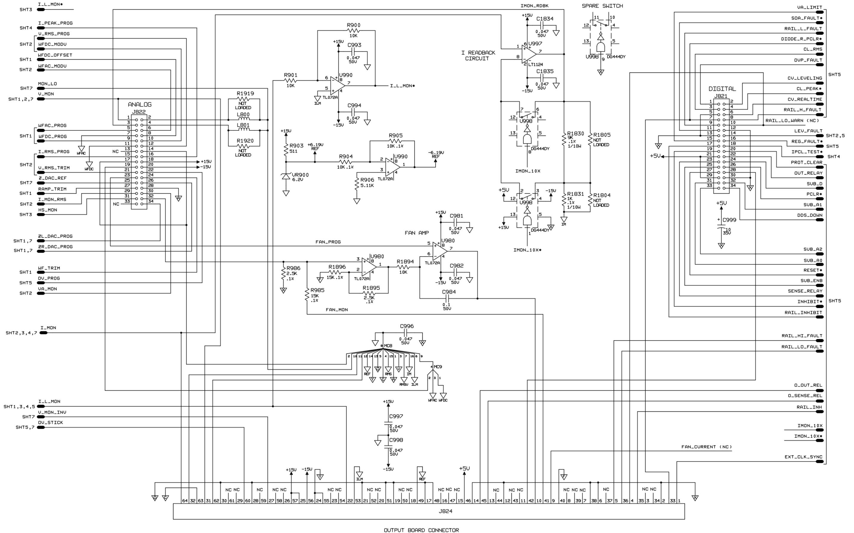
Figure 6-19. Control Assembly, Schematic Diagram (sheet 6 of 7)
