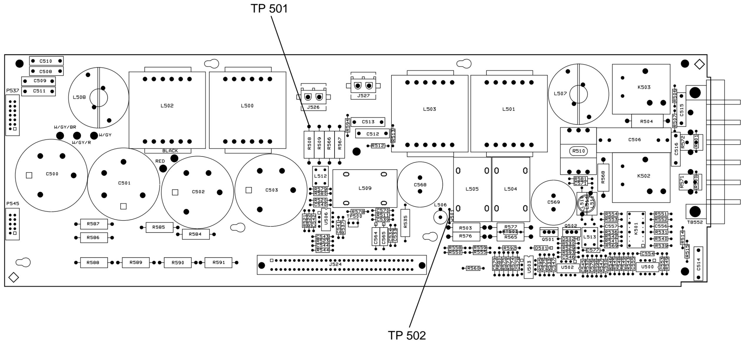
Figure 6-20. Output Board, Component Locations
