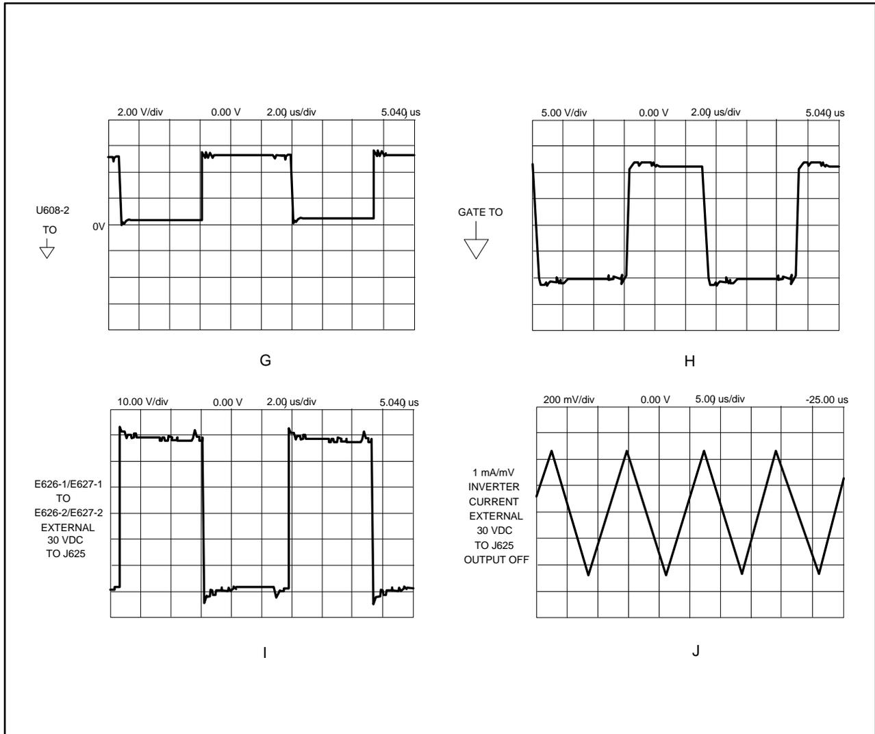
Figure 4-8. Inverter Assembly - Test Waveforms (sheet 2 of 2)
