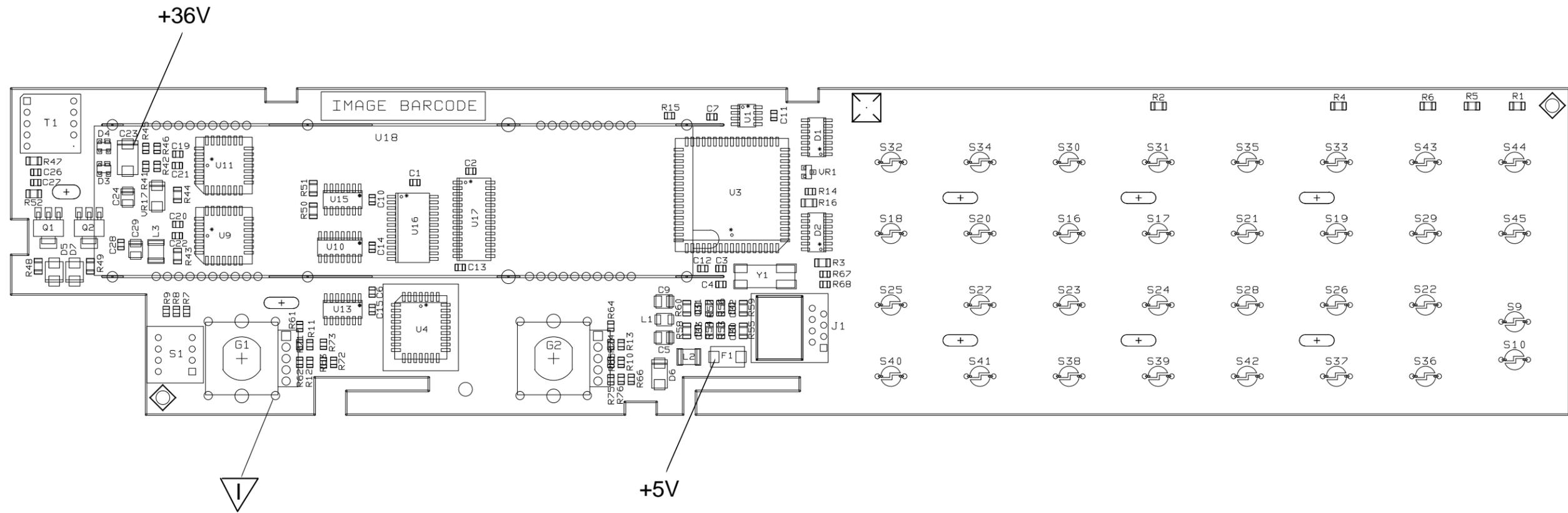
Figure 6-2. Front Panel Assembly, Component Locations
