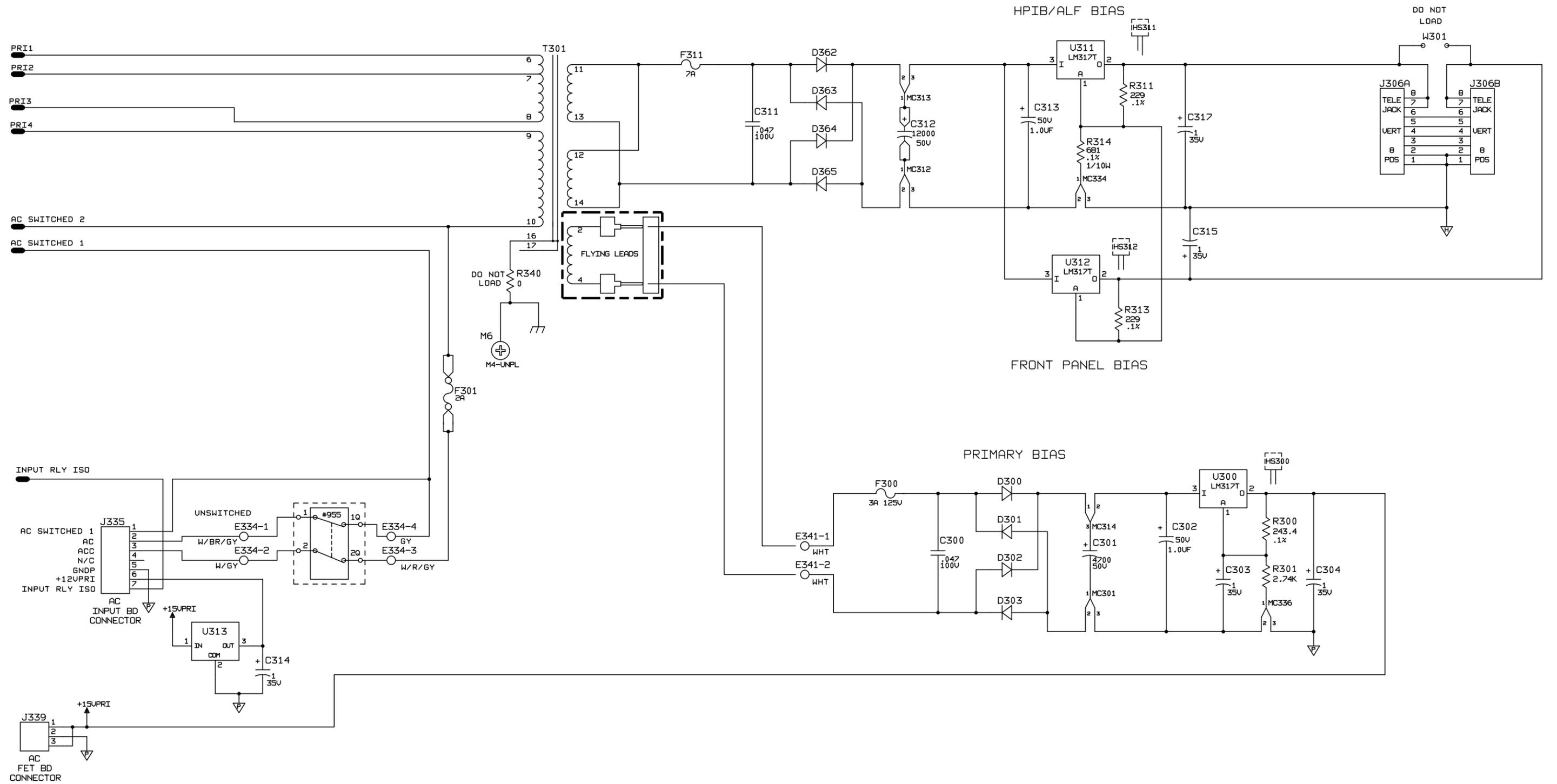
Figure 6-13. Bias Assembly, Schematic Diagram (sheet 1 of 2)
