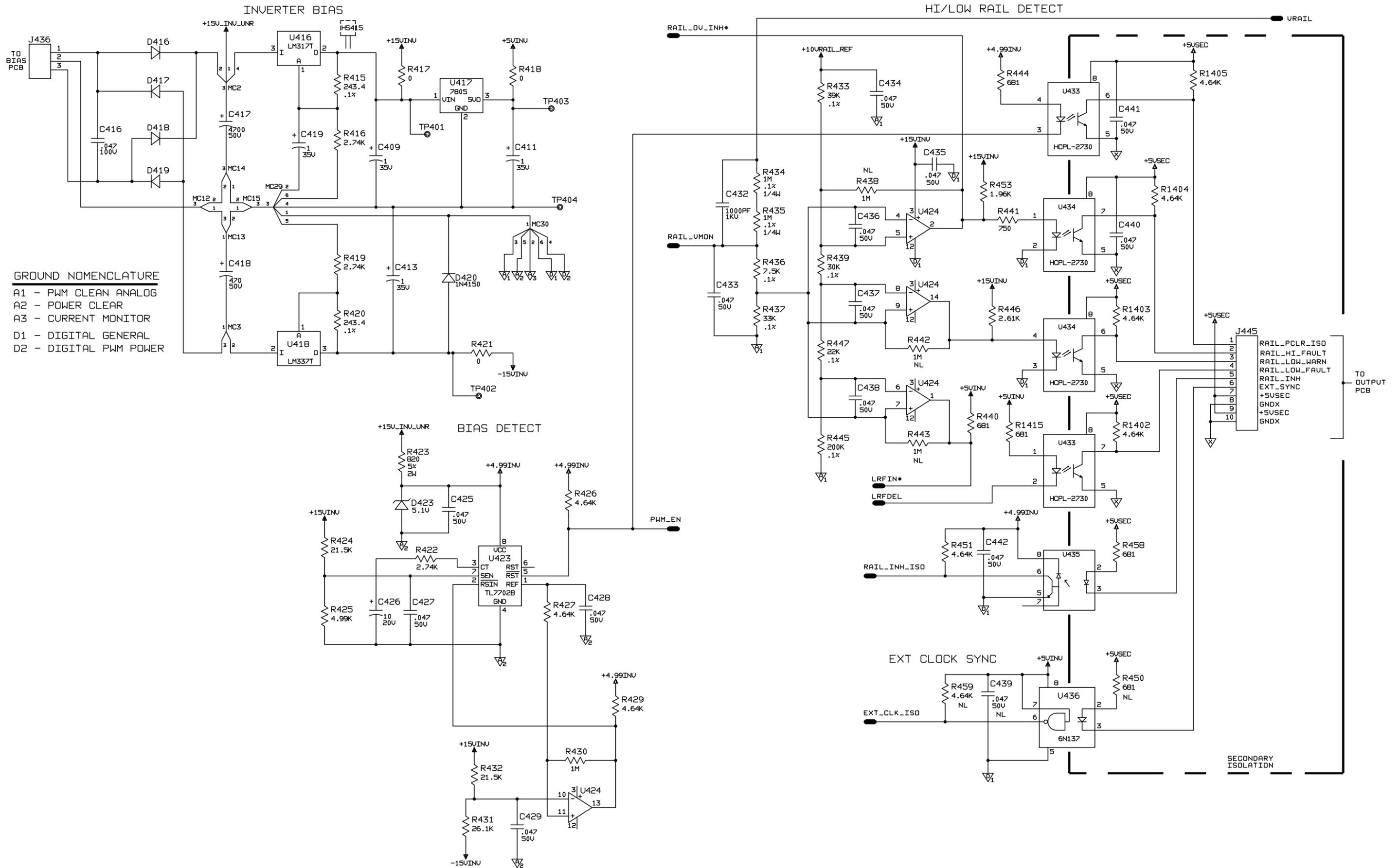
Figure 6-11. DC Rail/Diode Assembly, Schematic Diagram (sheet 2 of 3)
