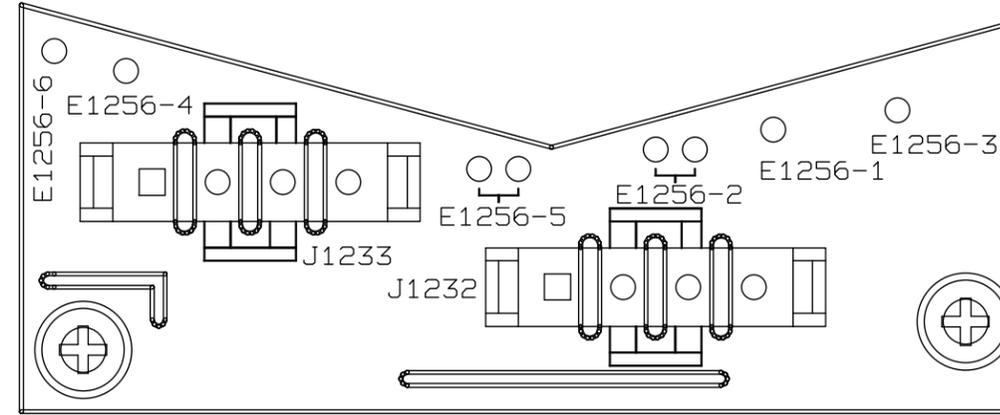
Figure 6-26. Transformer Assembly, Component Locations
