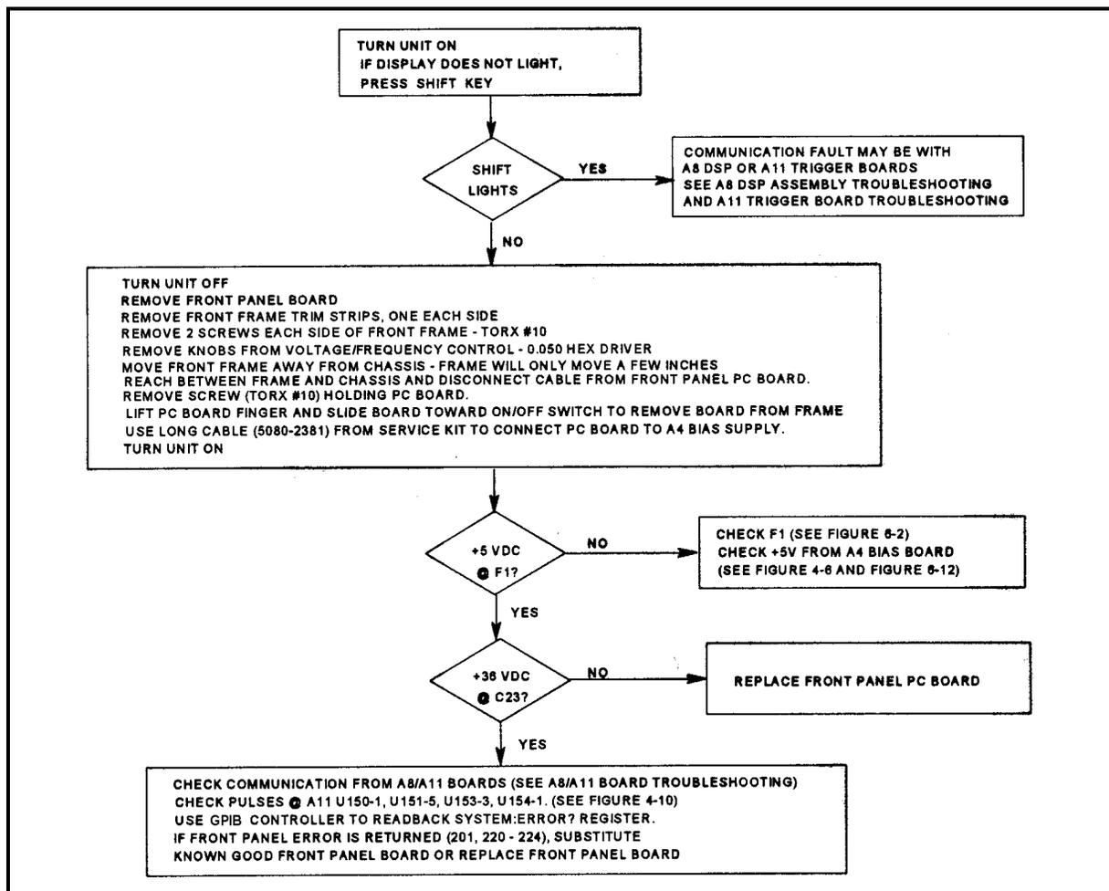
Figure 4-2. Front Panel Assembly Troubleshooting
