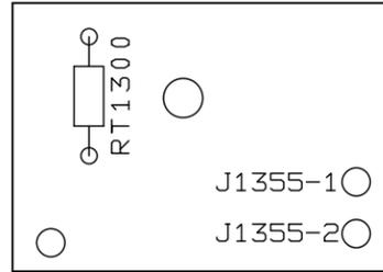
Figure 6-24. Thermistor Assembly, Component Locations
