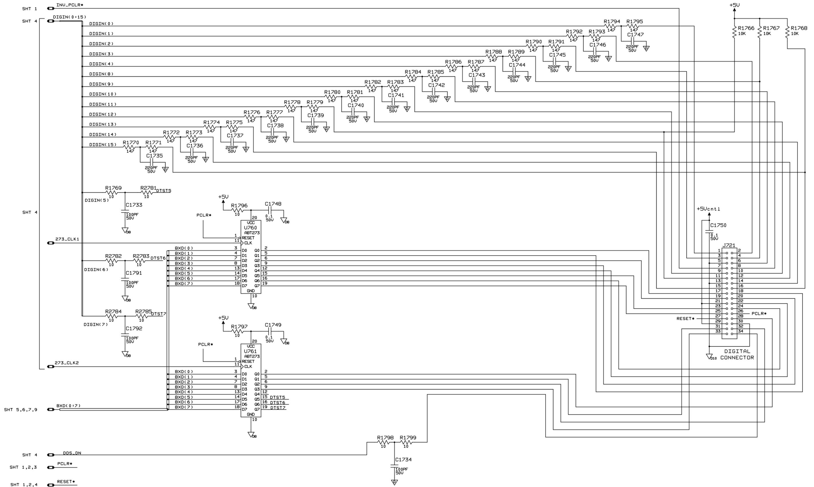
Figure 6-17. DSP Assembly, Schematic Diagram (sheet 8 of 10)
