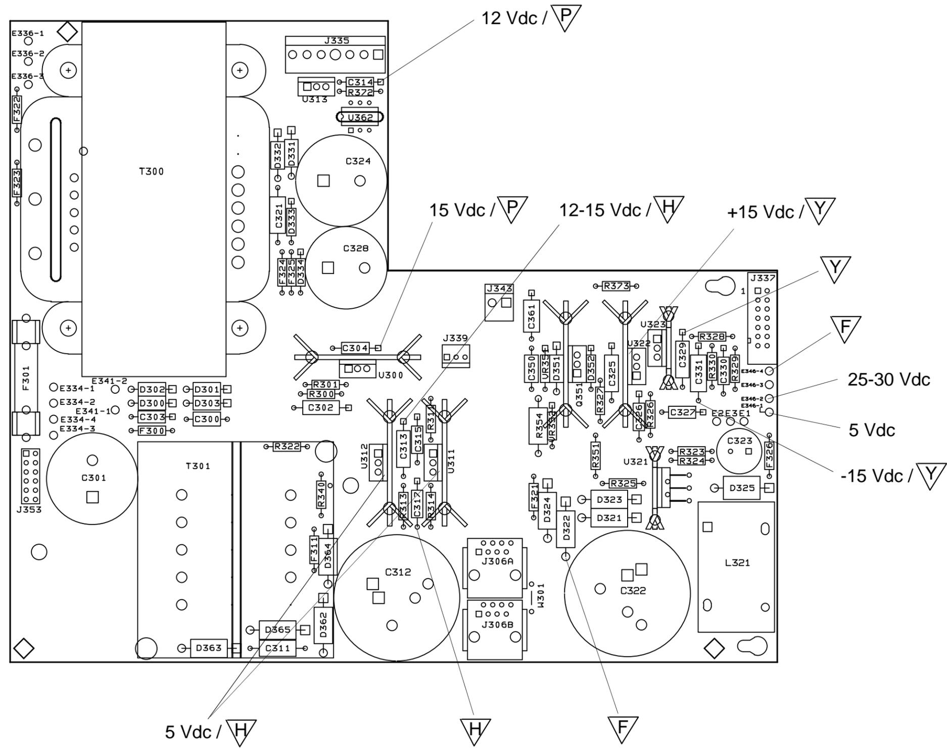
Figure 6-12. Bias Assembly, Component Locations
