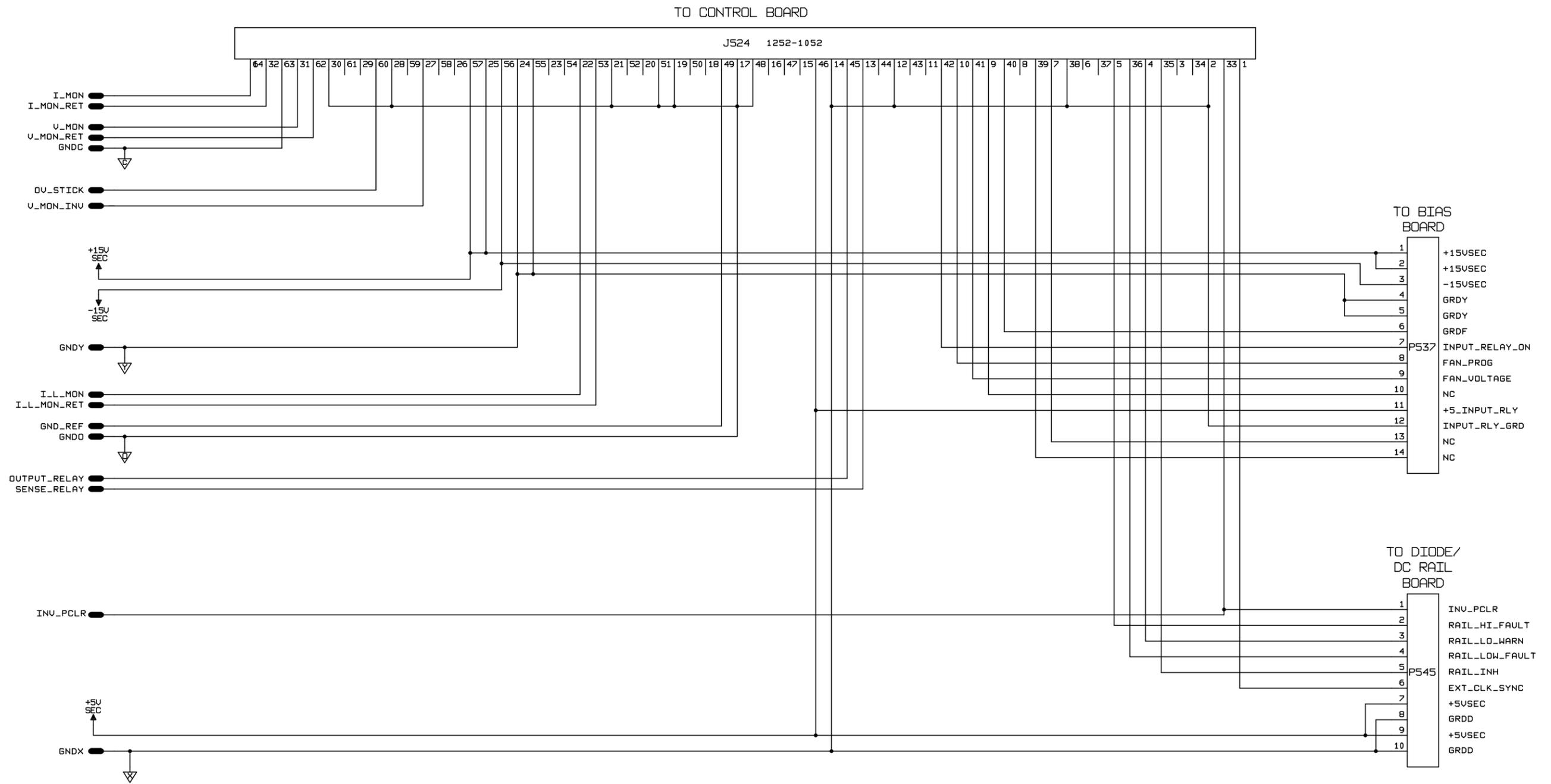
Figure 6-21. Output Assembly, Schematic Diagram (sheet 4 of 4)
