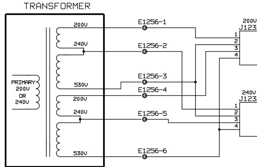
Figure 6-27. Transformer Assembly, Schematic Diagram
