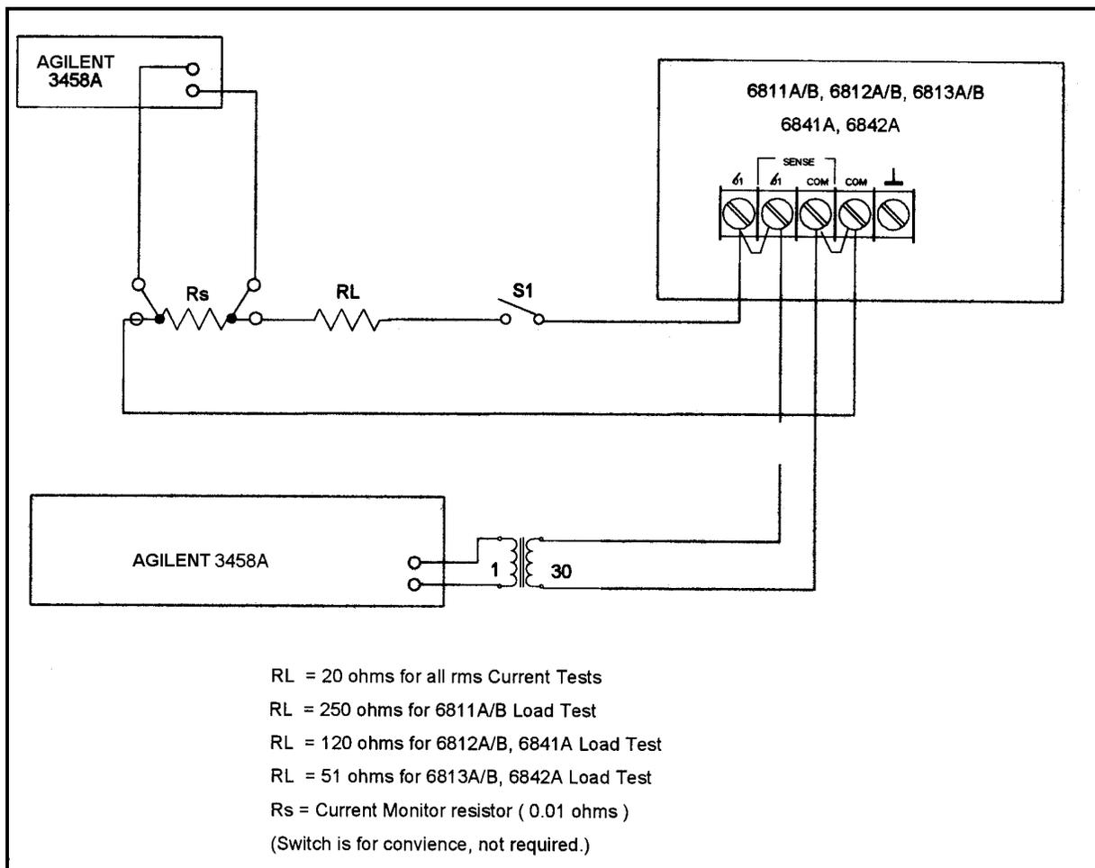
Figure 2-1. Test Setup
