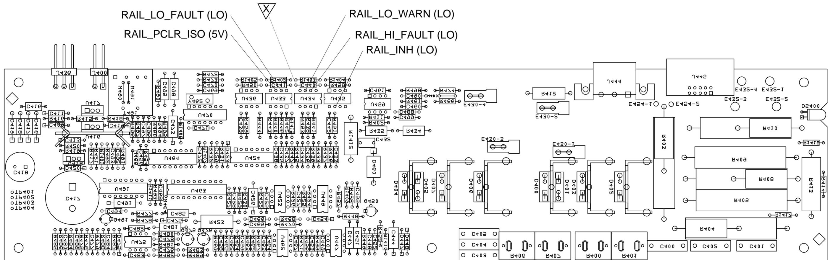
Figure 6-10. DC Rail/Diode Assembly, Component Locations (sheet 1 of 2)
