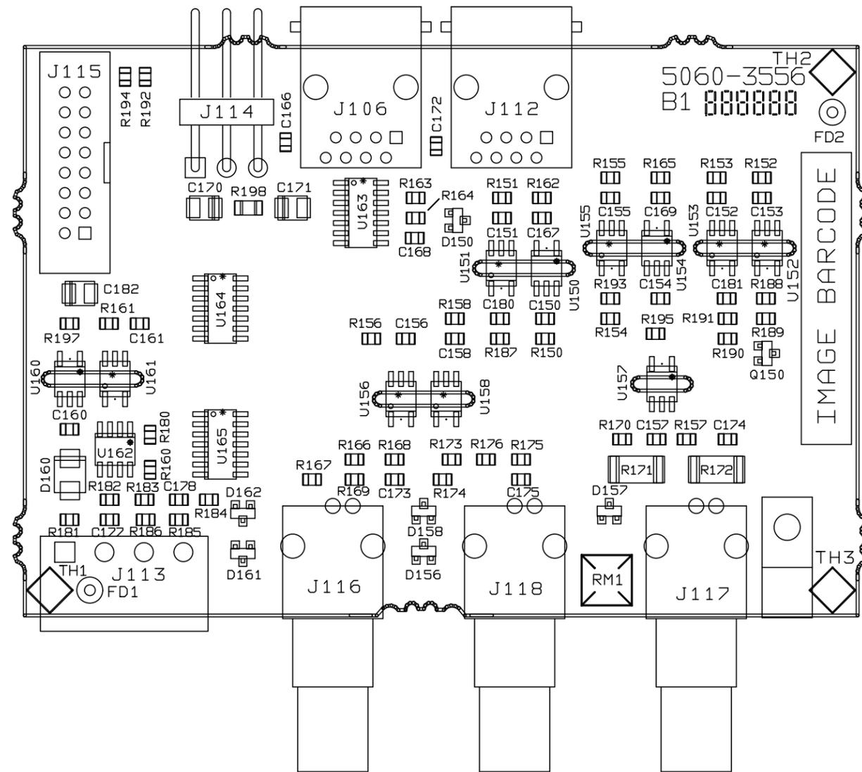
Figure 6-22. Trigger Board, Component Locations
