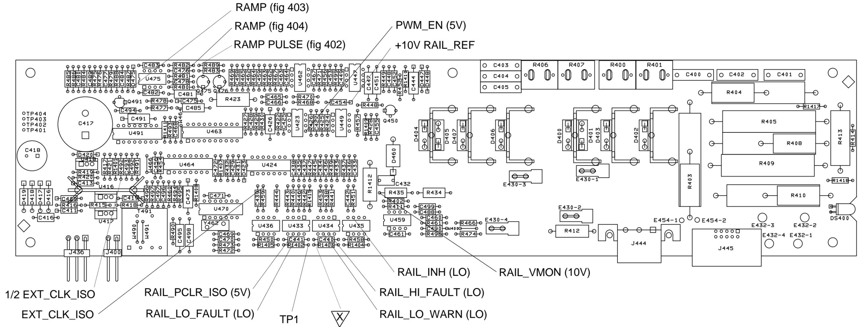
Figure 6-10. DC Rail/Diode Assembly, Component Locations (sheet 2 of 2)
