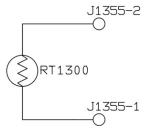
Figure 6-25. Thermistor Assembly, Schematic Diagram
