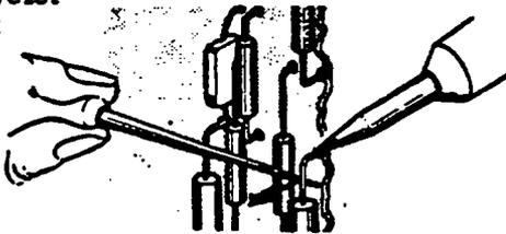
2. Reheat solder in vacant eyelet and quickly insert a small awl to clean inside of hole.
