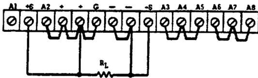
Figure 3-7. Remote Sensing
