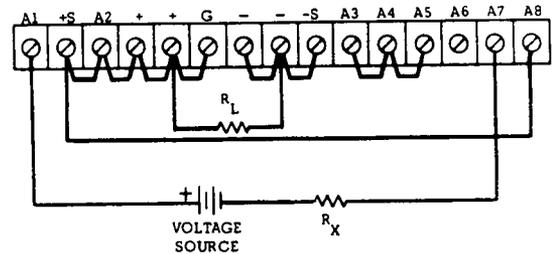
Figure 3-6. Remote Voltage Programming (Constant Current)
