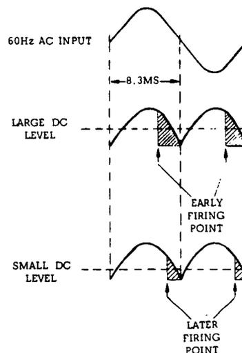
Figure 4-3. SCR Phase Control of DC Input Level
