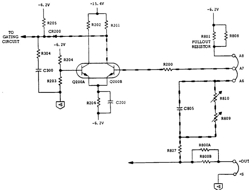
Figure 4-7. Constant Current Input Circuit, Simplified Schematic
