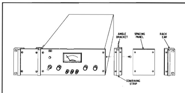
Figure 2-2. Rack Mounting, One Unit
