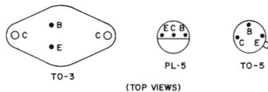
**12. PIN LOCATIONS FOR INTEGRATED CIRCUITS AND THE RESISTOR NETWORK ARE SHOWN BELOW:**
