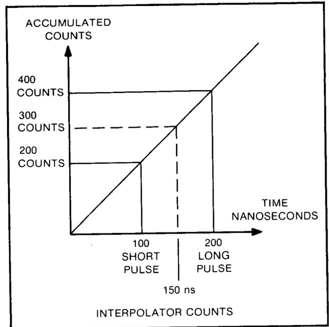
Figure 8-39. Short and Long Calibration Pulses Example
