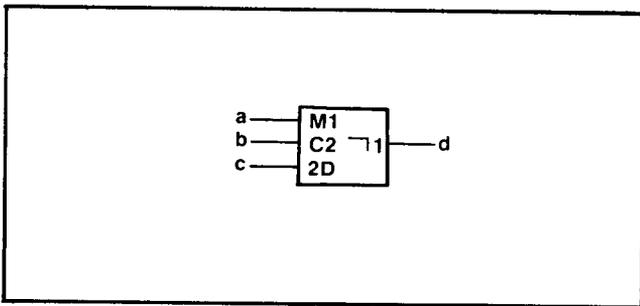
Figure 8-18. Type of Flip-Flop Determined by Mode
