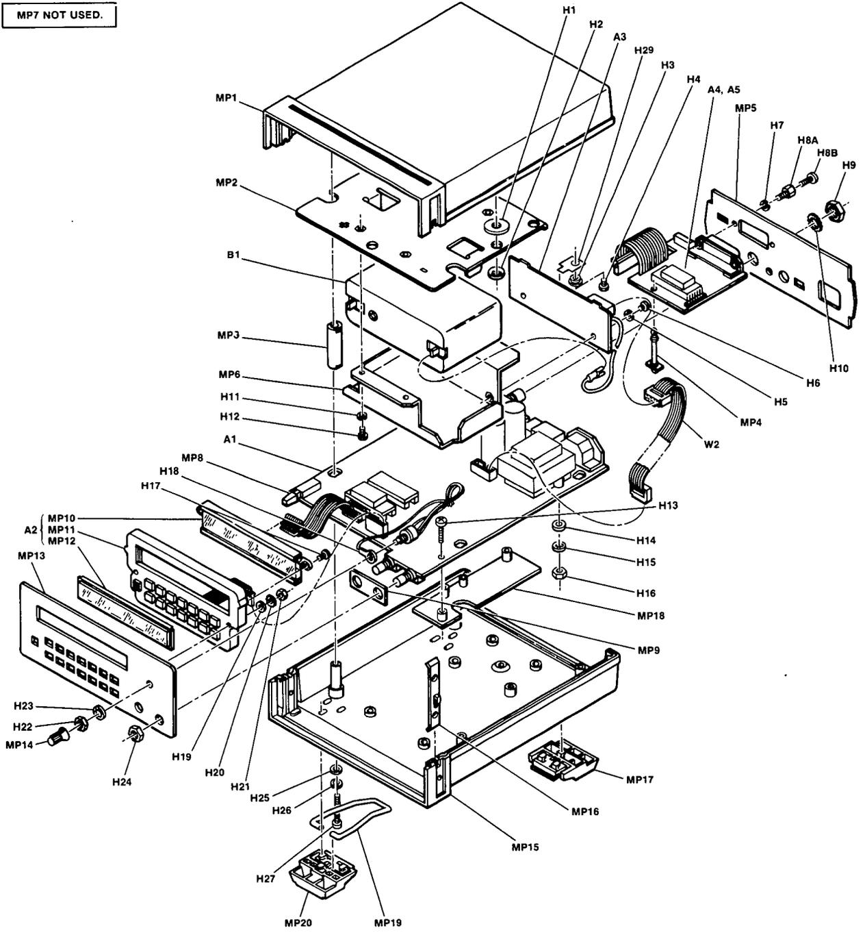
Figure 6-2. HP 5385A Exploded View
