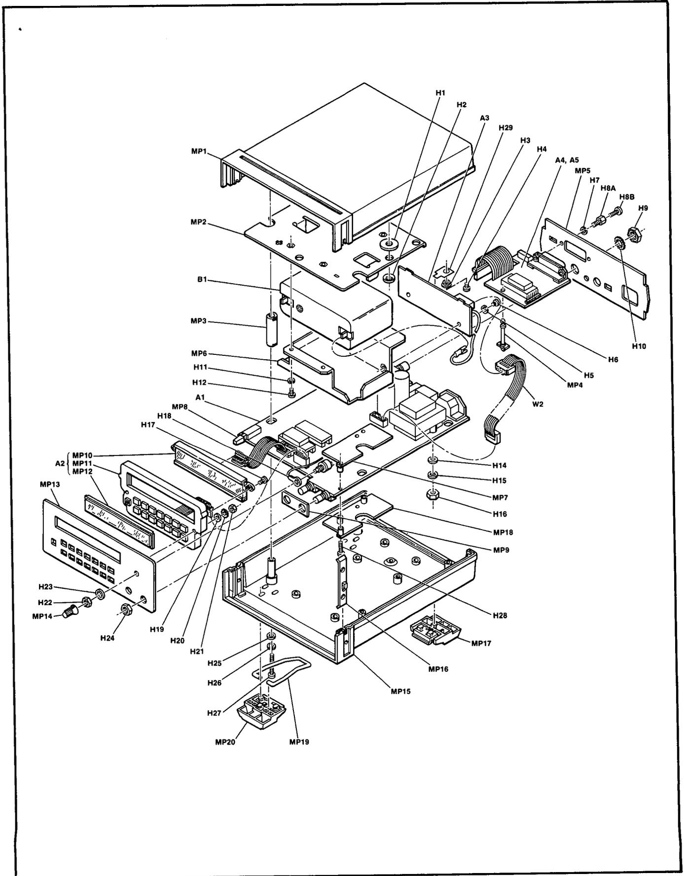
Figure 6-1. HP 5384A Exploded View
