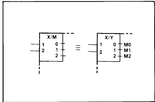
Figure 8-29. Coder Producing One Type of Dependency
