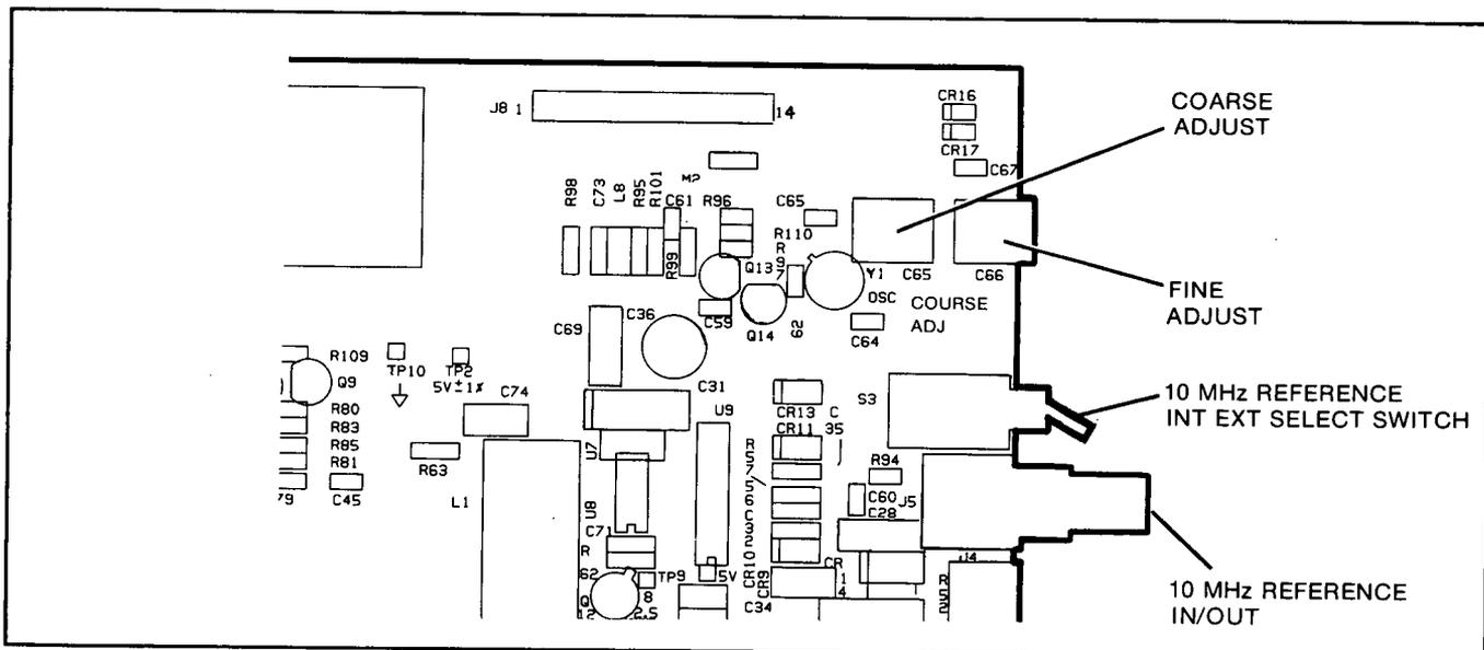
Figure 5-8. Standard Oscillator Coarse and Fine Adjustment Location
