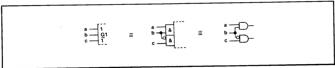
Figure 8-5. G Dependency Between Inputs
