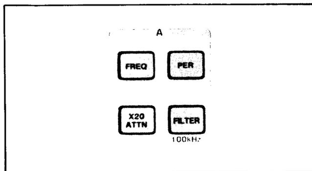
Figure 3-2. Front Panel A Channel Function Keys
