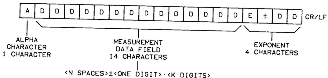
The decimal point is omitted if it is the last character preceding the exponent "E" in the output string. The first digit will be zero only if the data output is zero. At times, the display may contain a number which is equivalent to zero (such as 0E-9). If this is the case, the HP-IB output will be:
