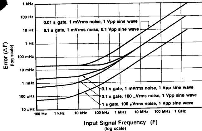
Graph 1. Frequency Resolution Error: Noise on the input signal and internal uncertainties affect Frequency and Period measurements. For Period, invert the period (P) of
