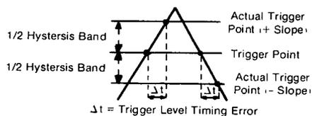
Auto trigger disabled: trigger point = trigger level reading.
