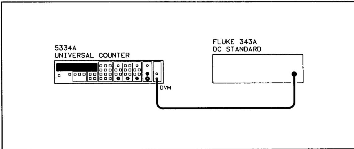
Figure 4-14. DVM Accuracy Test Setup
