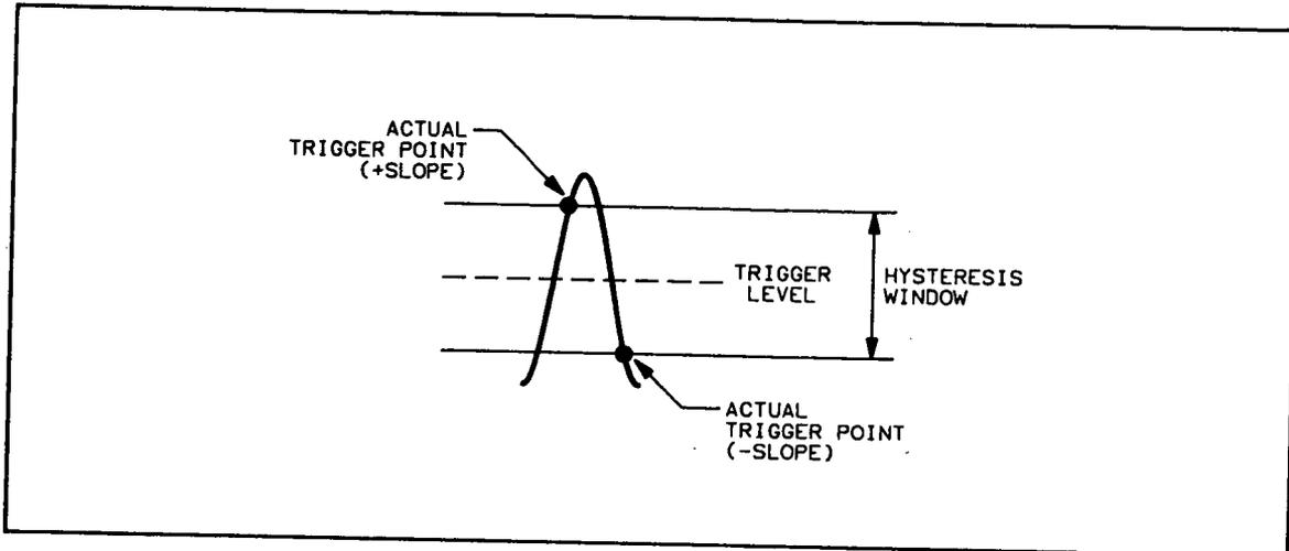
Figure 3-9. Trigger Level and Actual Trigger Point
