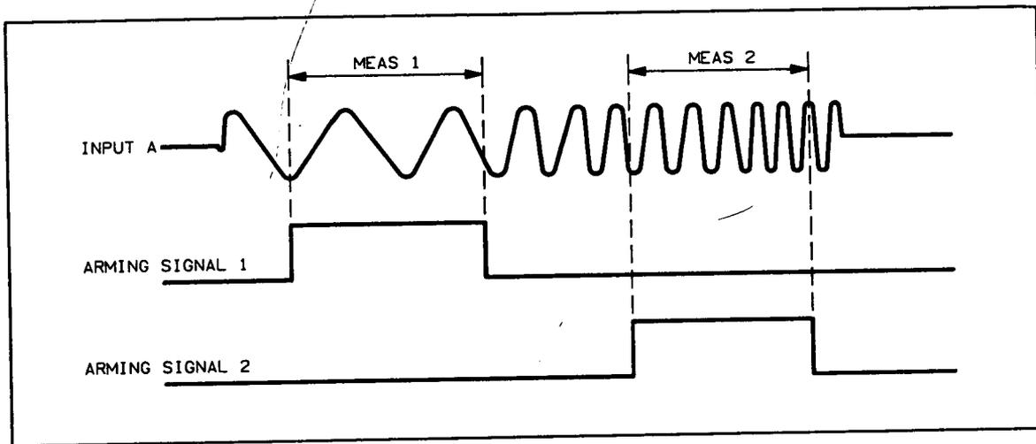
Figure 3-12. Use of External Arming to Measure Frequency
