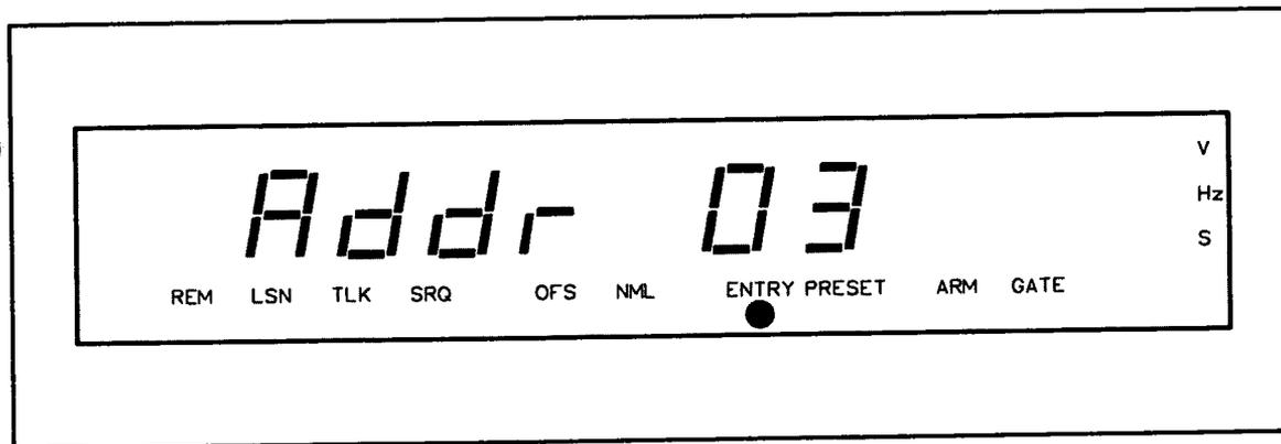
*Figure 3-61. HP 5334A/B Address Entry Display*
