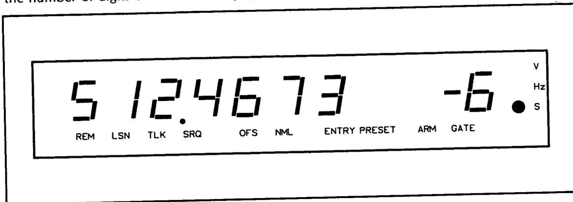
*Figure 3-28. Pulse Width Measurement Display*
