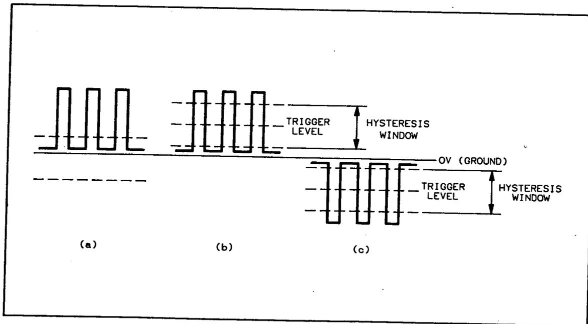
Figure 3-10. Trigger Level Control Shifts Hysteresis Window
