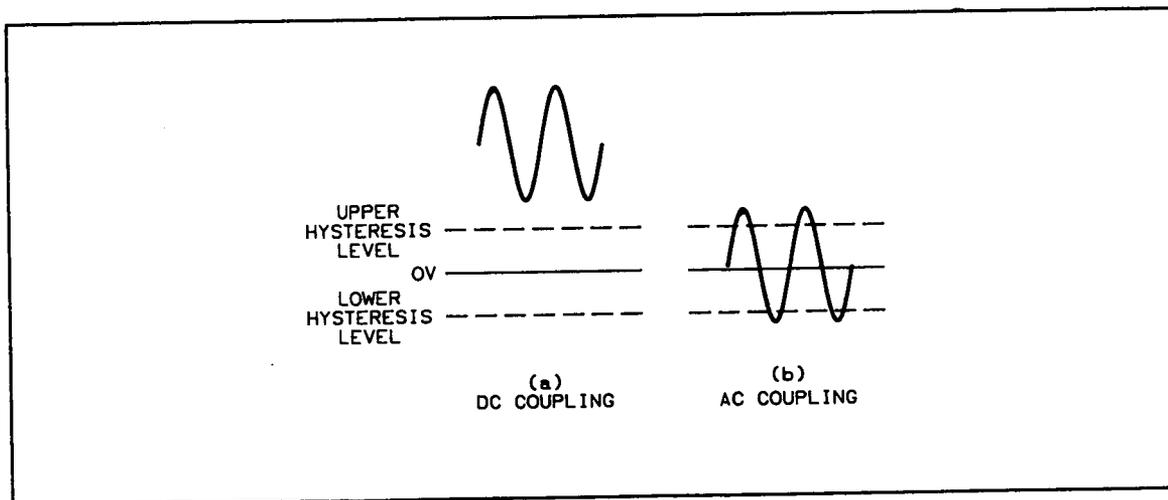
Figure 3-8. AC-DC Coupling
