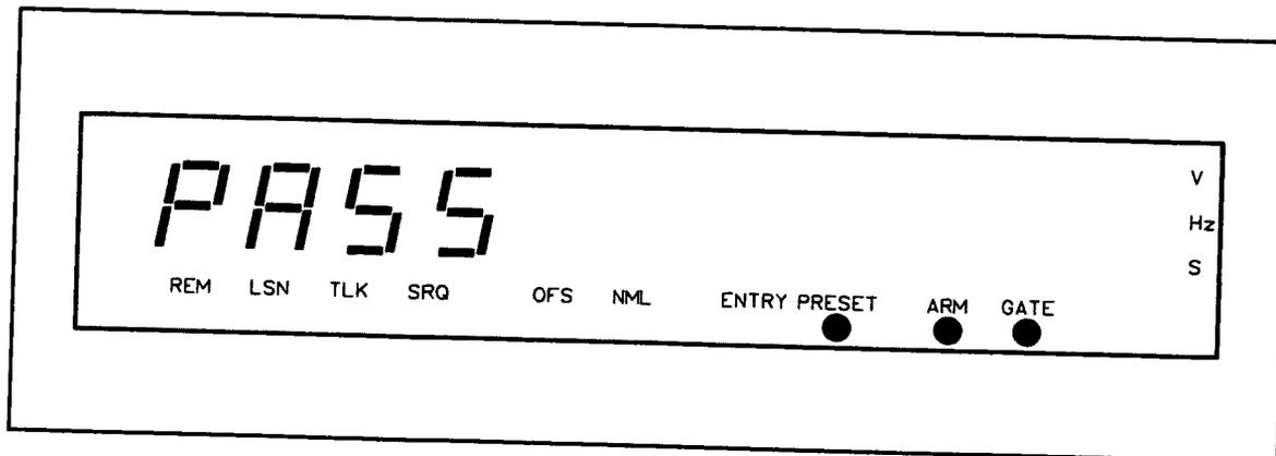
Figure 3-42. Self-Check PASS Display
