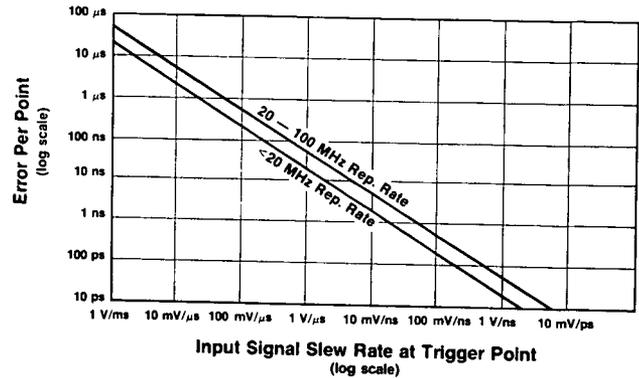
Graph 4. Trigger Level Timing Error: Affects the Start and Stop points of all time interval measurements. Total error is the larger of the two trigger point errors.
