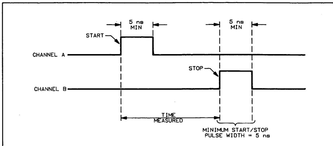
Figure 3-13. Time Interval Measurement
