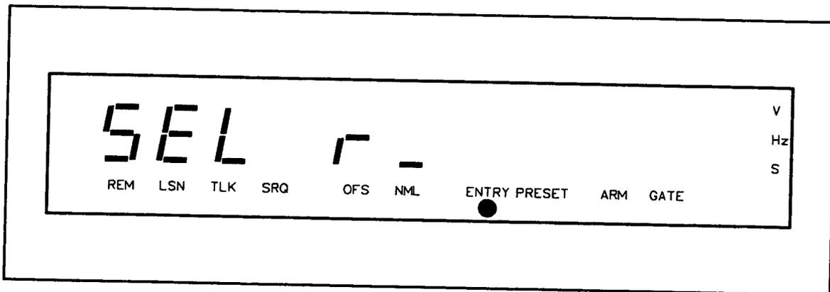
*Figure 3-24. HP 5334A RECALL ENTRY Mode Display*
