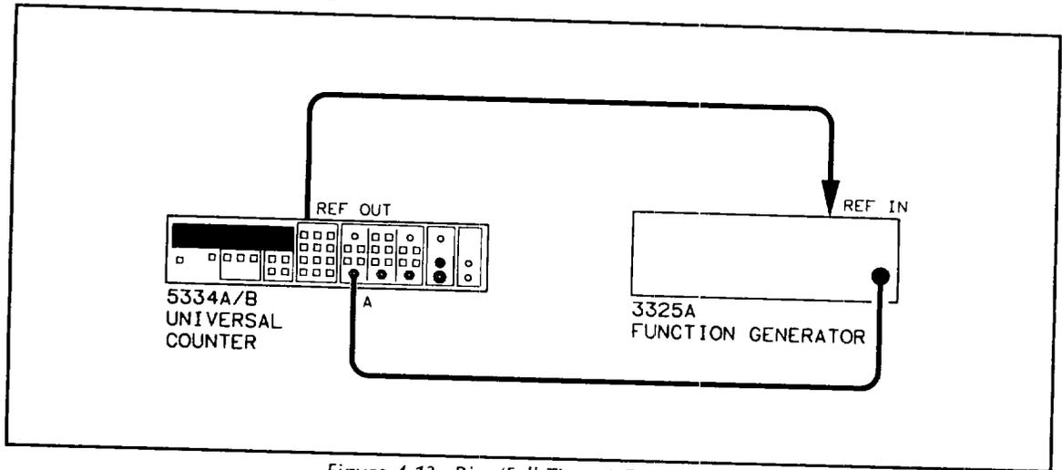
Figure 4-13. Rise/Fall Time A Test Setup
