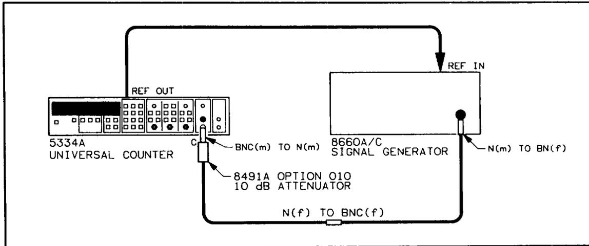
Figure 4-15. HP 5334A Channel C Frequency and Sensitivity Setup
