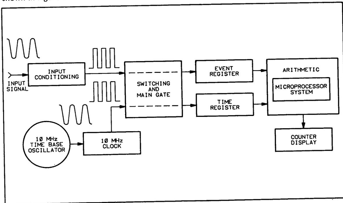
Figure 3-1. Simplified Block Diagram of the Reciprocal Counter
