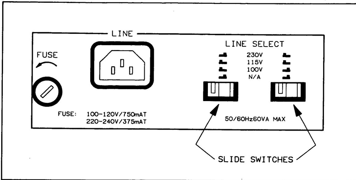
Figure 2-2. HP 5334B Voltage Selection with Slide Switches
