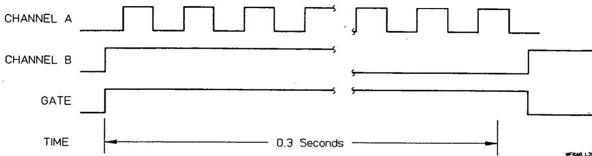
Notice that the measurement is completed by the first channel B event after the gate time interval.
