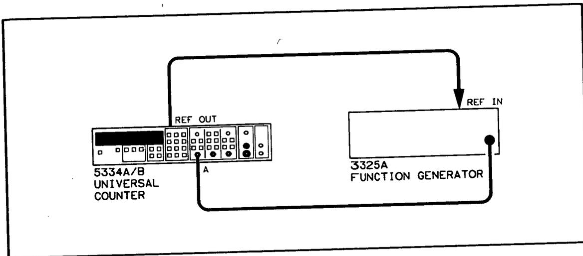
Figure 4-10. Time Interval A to B Test Setup
