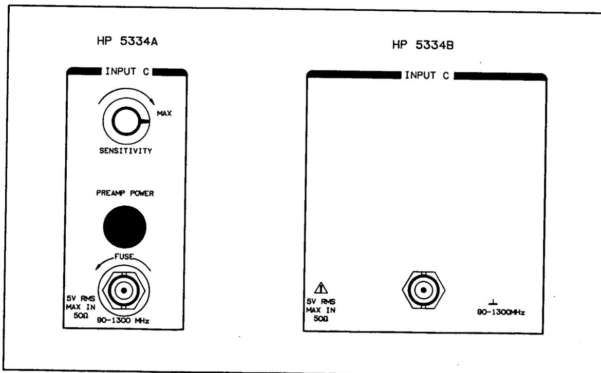
Figure 3-37. HP 5334A and HP 5334B C-Channels
