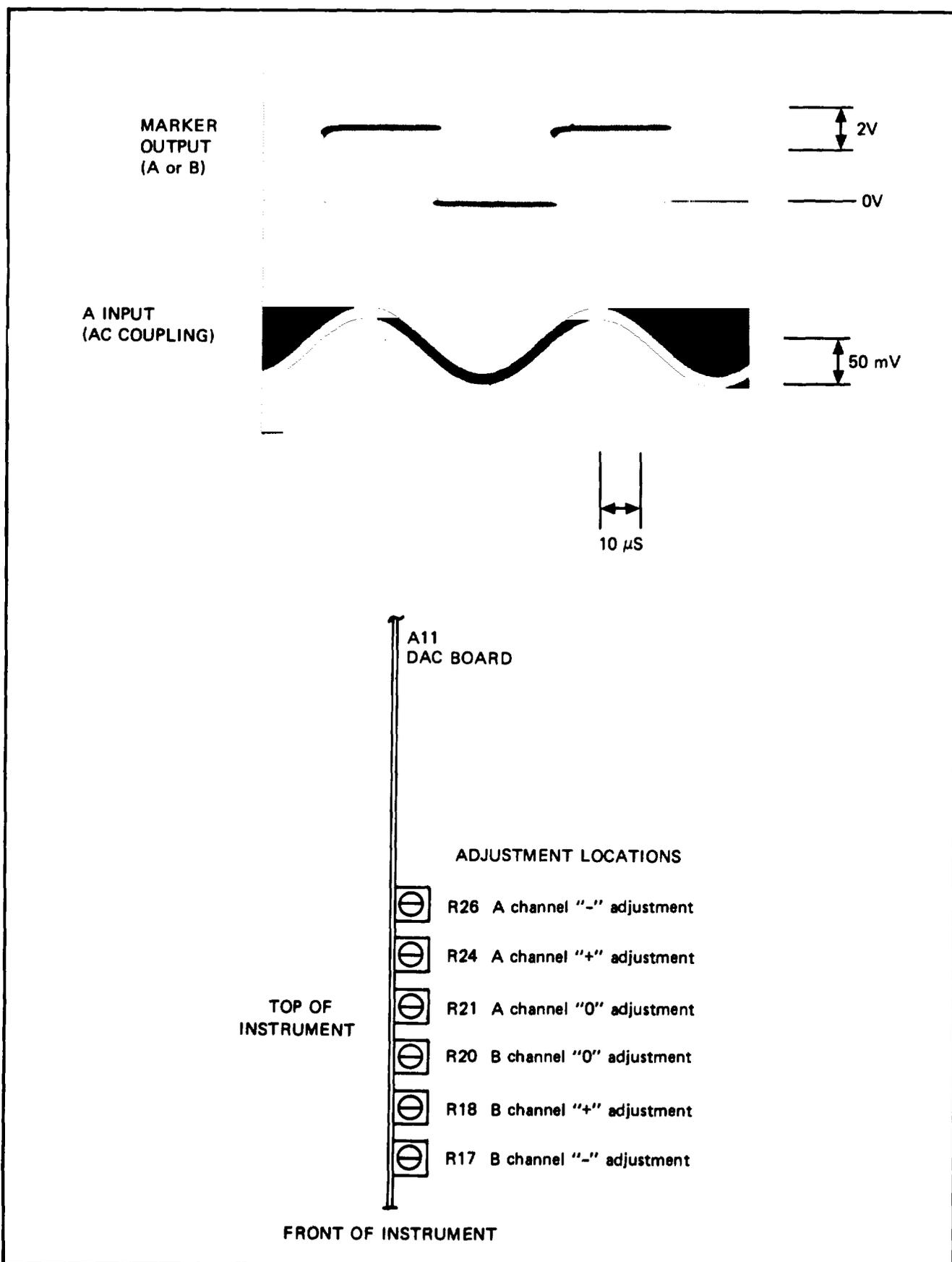
Figure 5-3. DAC Adjustment oscilloscope readout and adjustment locations
