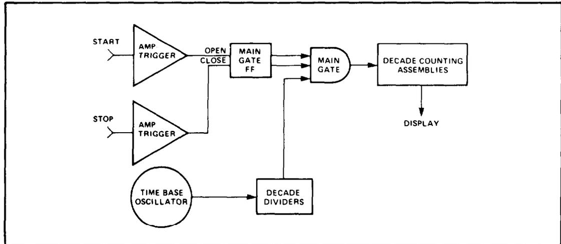
*Figure 4-3. Basic Elements of a Time Interval Counter*
