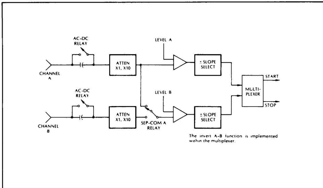
Figure 3-8. Programmable Input Switch Configuration for COM A
