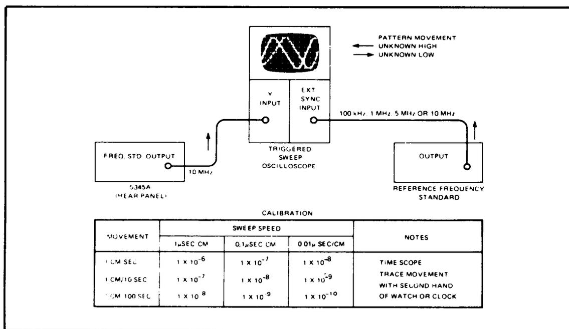
Figure 5-1. 10 MHz Oscillator Frequency Check
