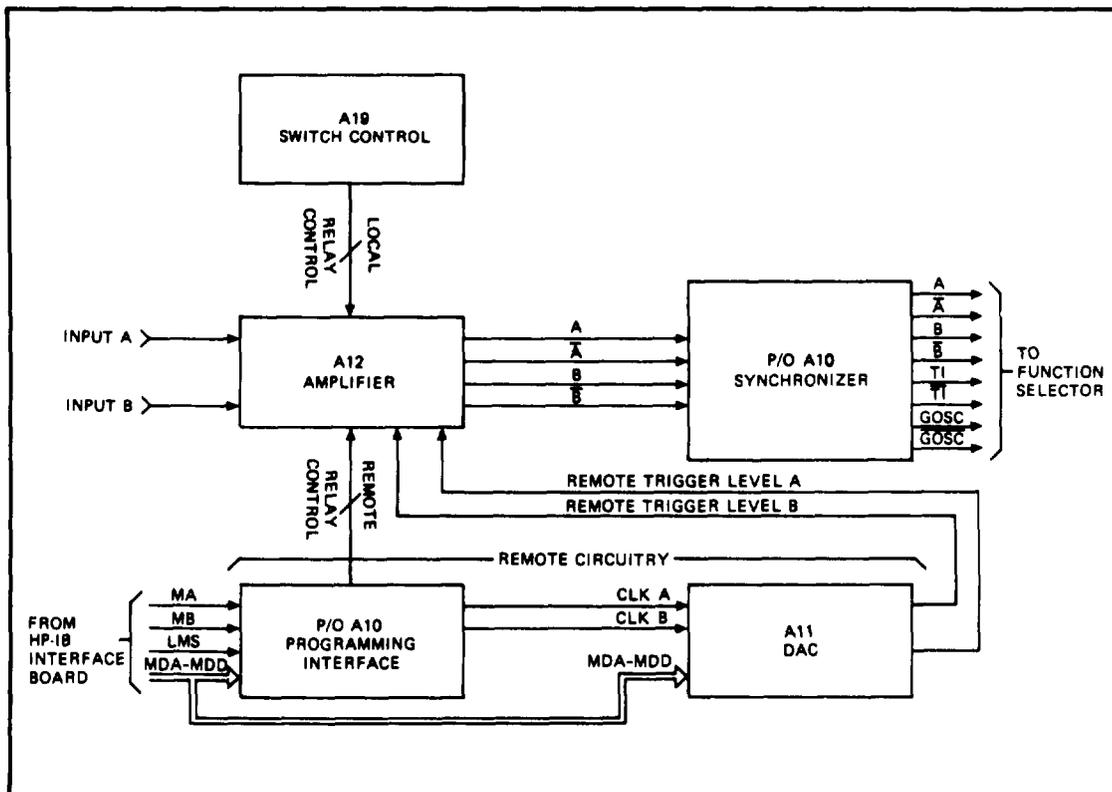
Figure 4-9. Remote Controllable (Programmable) Input Block Diagram
