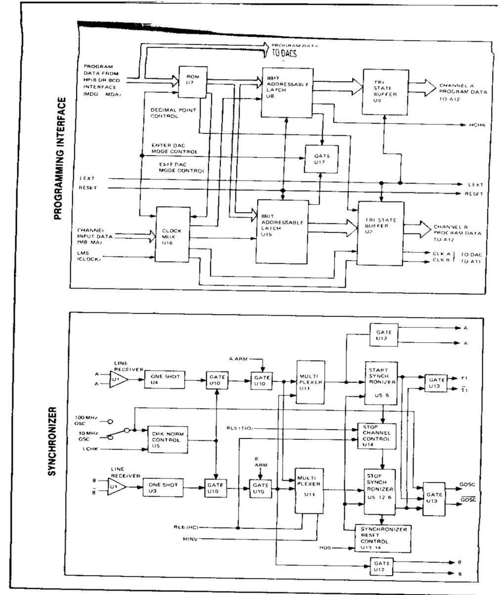
Figure 8-15. A10 Synchronizer Block Diagram
