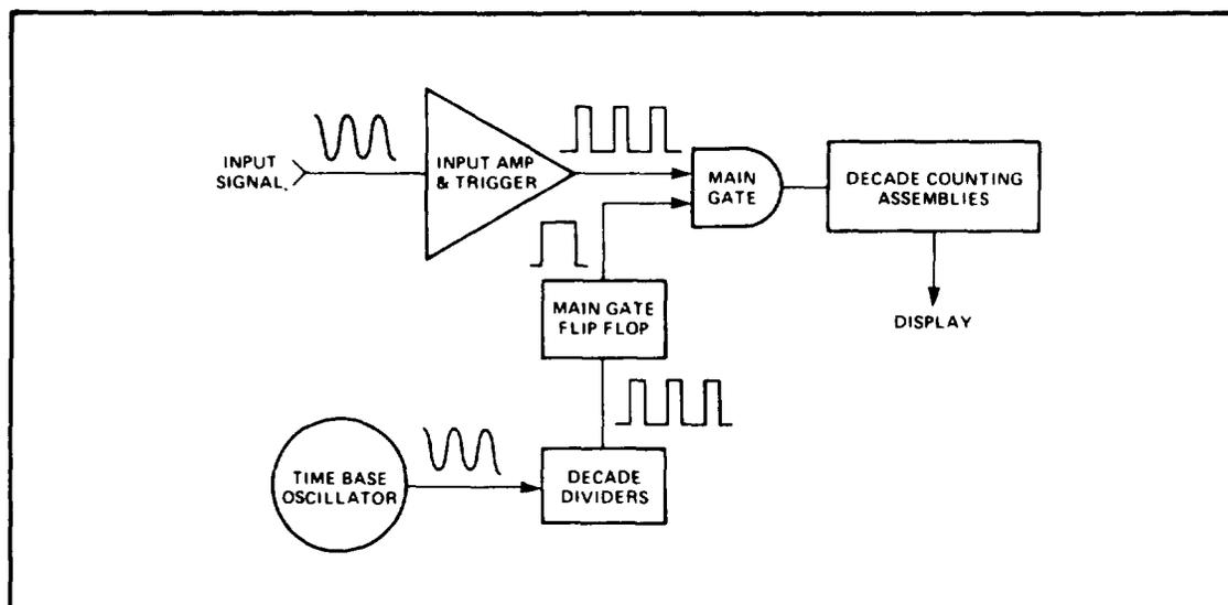
*Figure 4-1. Basic Elements of the Frequency Counter*
