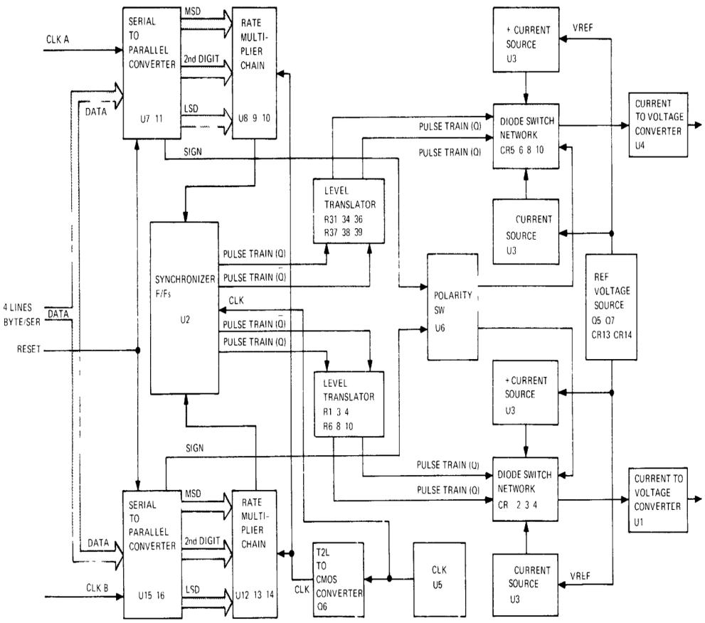
Figure 8-17. All Digital-to-Analog Converter Block Diagram
