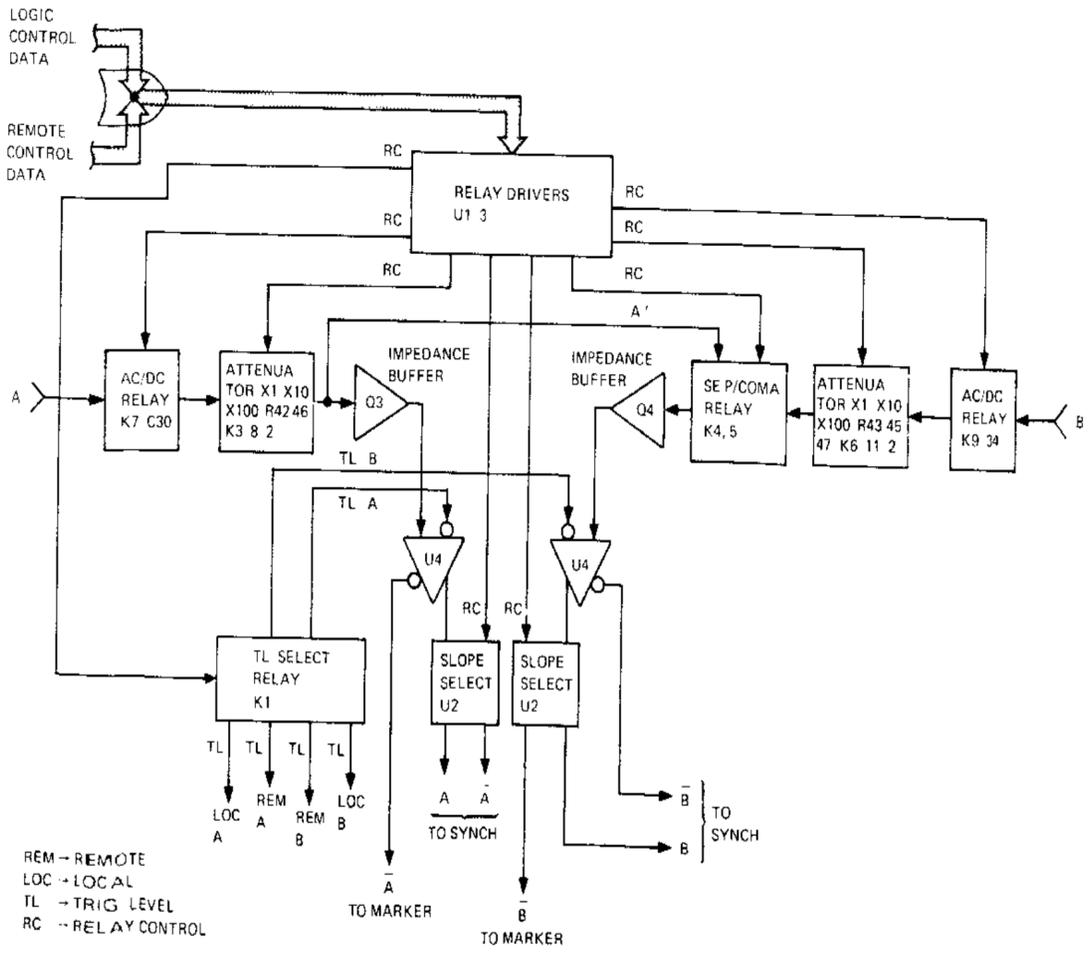
Figure 8-19. A12 "A-B" Channel Block Diagram
