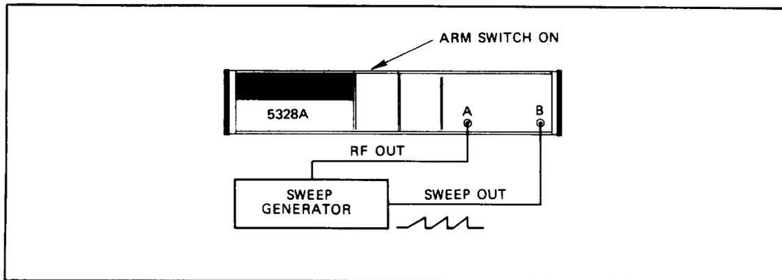
Figure 3-1. Measuring Linearity
