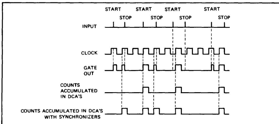
Figure 4-5, Synchronizer Operation with Time Interval Averaging
