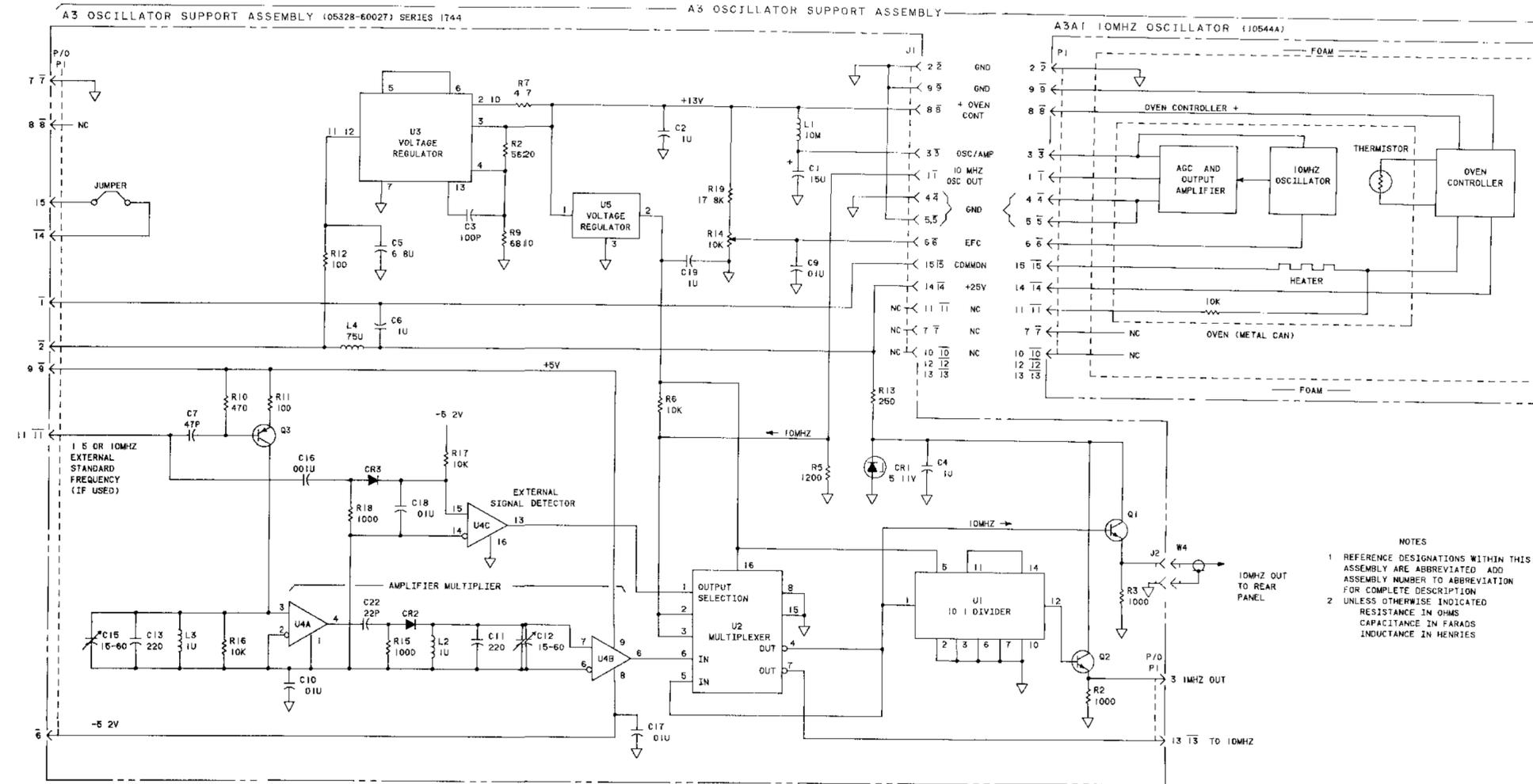
Figure 8-10. A3/A3A1 Oscillator Support Schematic and Components
