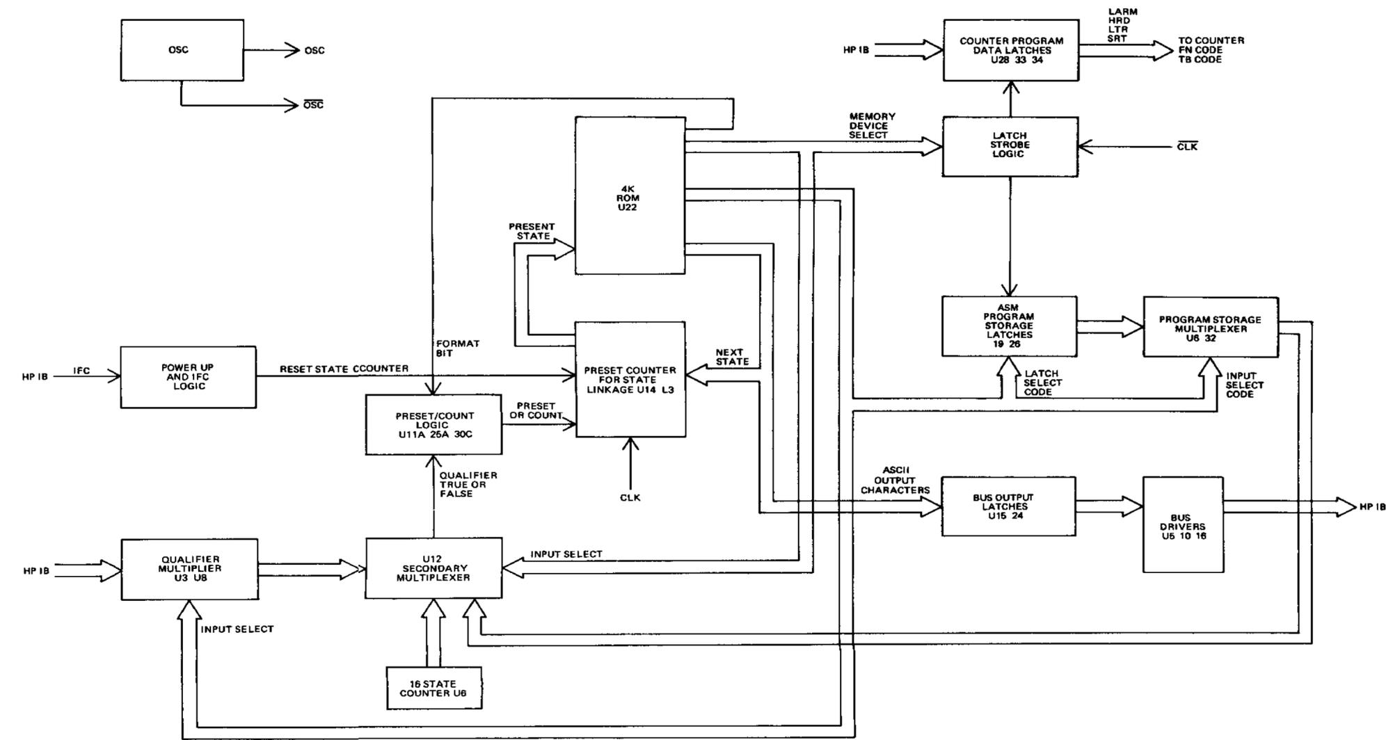
Figure 8-21. A15 HP-IB Interface Block Diagram
