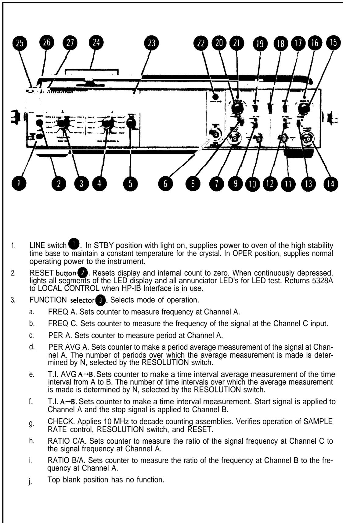
1. LINE switch **1**. In STBY position with light on, supplies power to oven of the high stability time base to maintain a constant temperature for the crystal. In OPER position, supplies normal operating power to the instrument.
