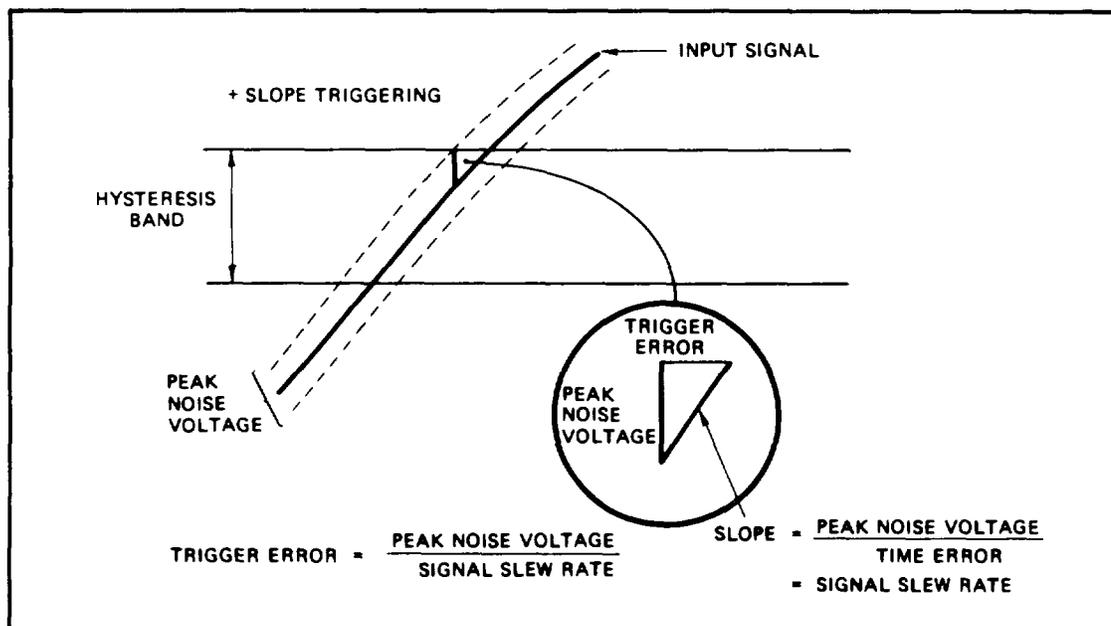
Figure 4-7. Trigger Error
