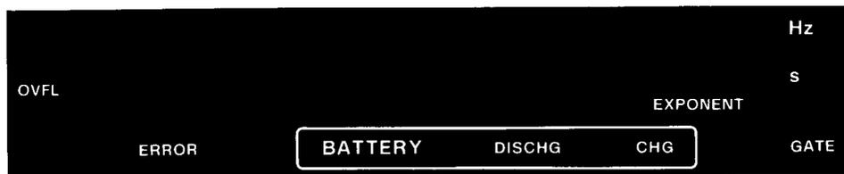
3-54. During this cycle, the microcomputer performs a check sum of the internal program in ROM and a bit pattern written into RAM. Additionally, a partial check of the MRC and I/O ports is performed. Any failure during the cycle will produce a numbered error message, momentarily displayed, and will latch the ERROR annunciator ON. Refer to Error Messages, paragraph 3-55.
