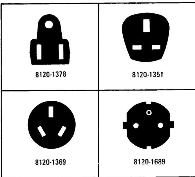
Figure 2-2. Power Cable and Mains Plug Part Numbers
