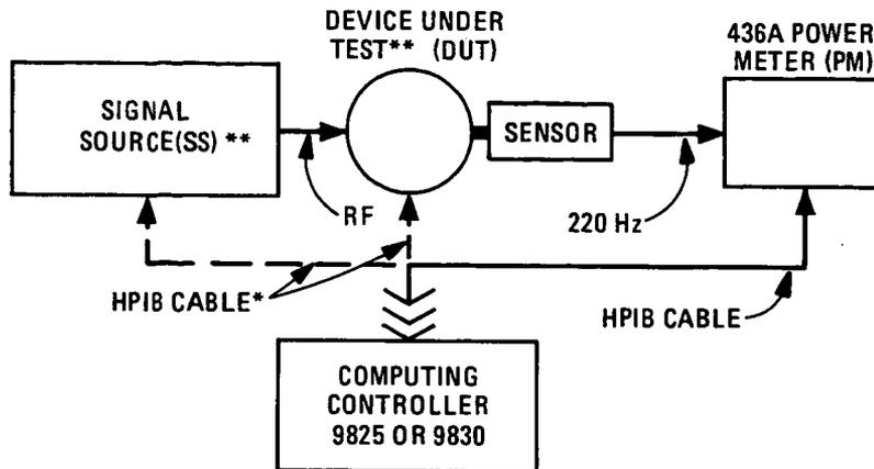
\* HP-IB cables shown with dotted lines are used only if the Source and Device under test are programmable.
