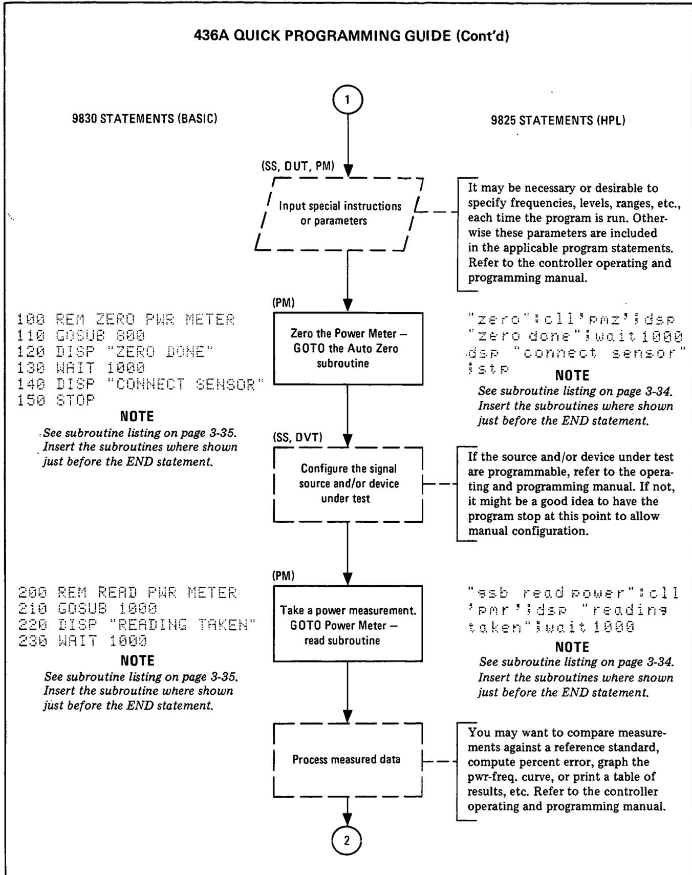
Figure 3-8. 436A Quick Programming Guide (2 of 5)
