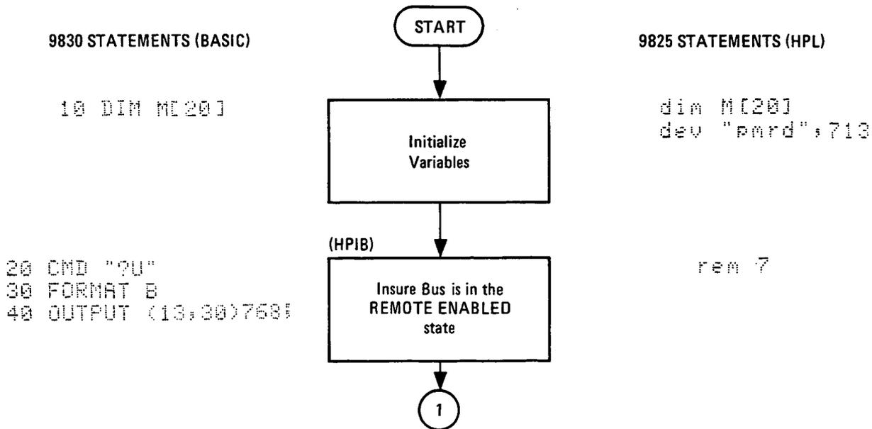
Figure 3-8. 436A Quick Programming Guide (1 of 5)
