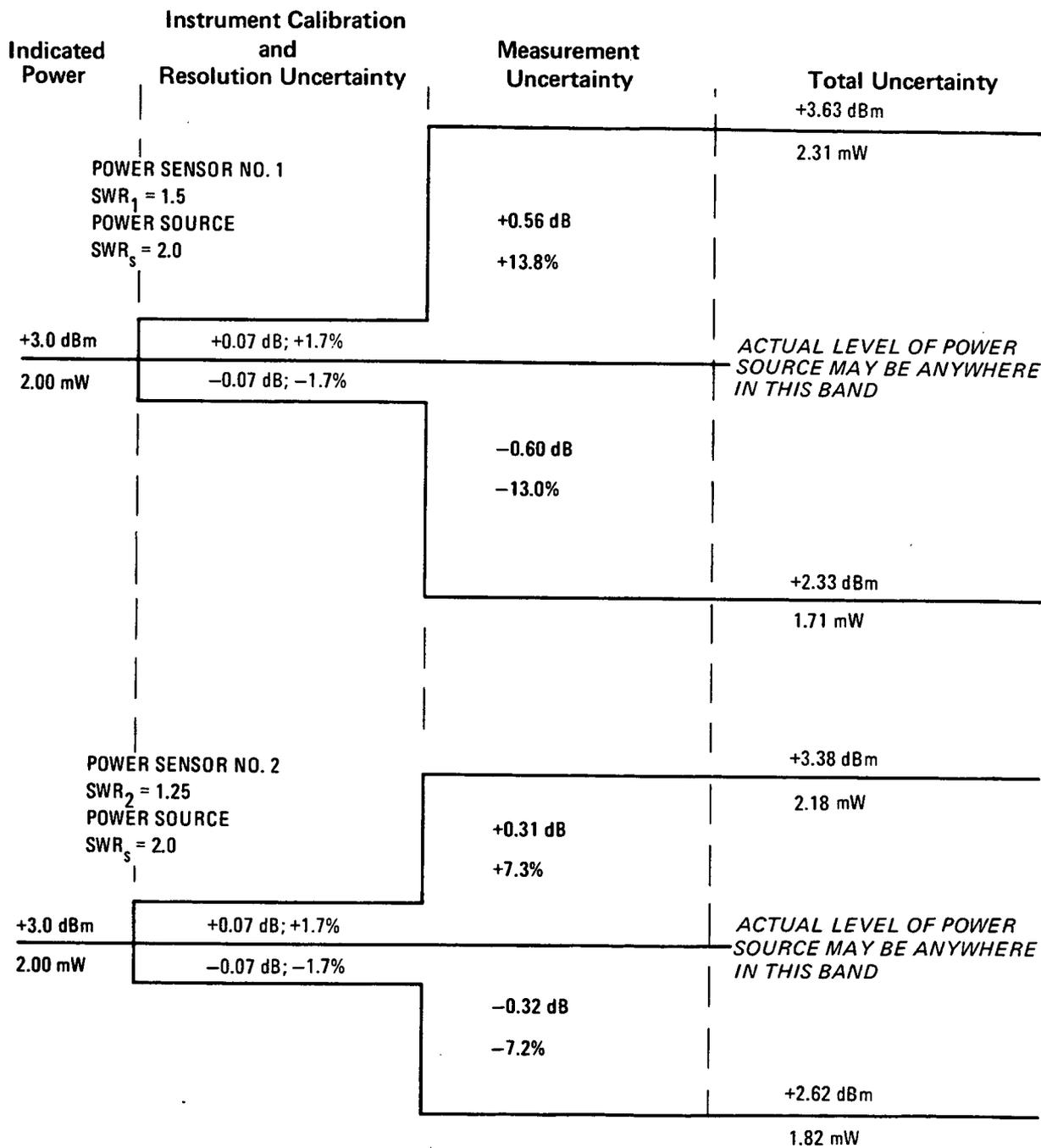
Figure 3-10. The Effect of Power Sensor Mismatch on Measurement Accuracy
