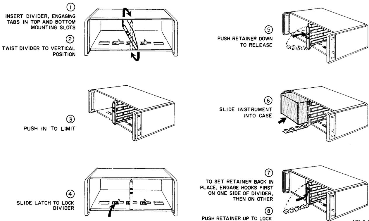
Figure 2-2. HP Model 1051A Combining Case Instrument Installation
