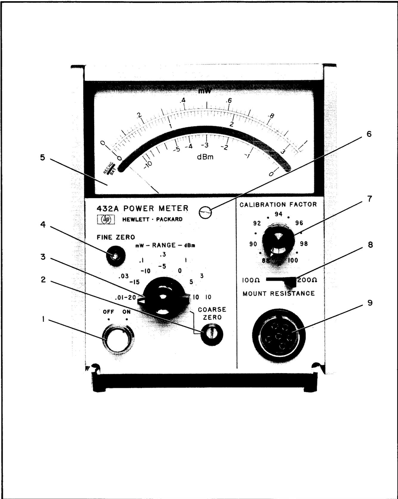
Figure 3-2. Front Panel Controls, Connectors and Indicators (Sheet 1 of 2)
