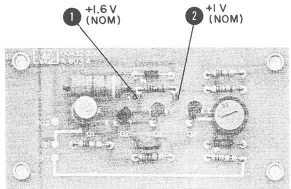
Figure 7-4. Model 432A Test Point Locations
