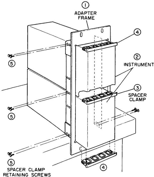
Figure 2-1. Sub-module Installation in Rack Adapter Frame
