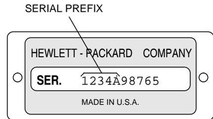
Figure 1-2. Instrument Identification
