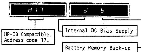
6. Automatic initial control settings. Instrument controls are automatically set as follows:
