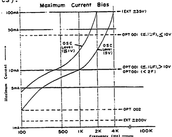
6. When a low capacitance (below  $0.1\mu\text{F}$ ) is to be measured using a dc bias, set rear panel DC BIAS switch to INT 35V/100V ( $\leq .1\mu\text{F}$ ) position (to obtain shorter bias voltage settling time). To apply an internal dc bias to a high capacitance sample ( $0.1\mu\text{F}$  to  $2\text{F}$ ), set the switch to INT 35V/100V ( $\leq 2\text{F}$ ) position.
