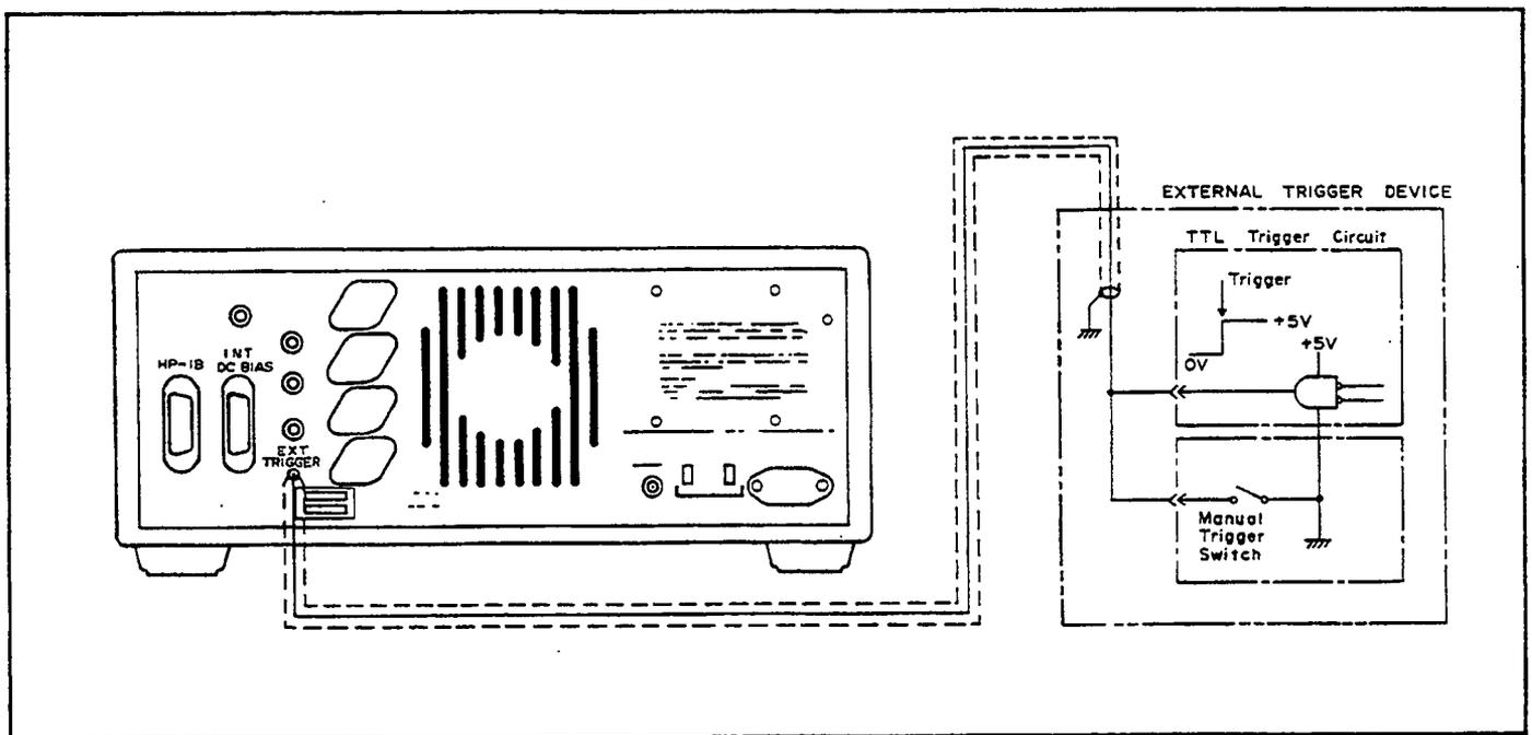
Figure 3-15. External Trigger Circuit.
