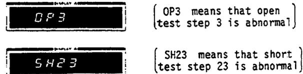
If an abnormal display is obtained, first check for test setup. If such display occurs even under proper test conditions, notify the nearest Hewlett-Packard office.
