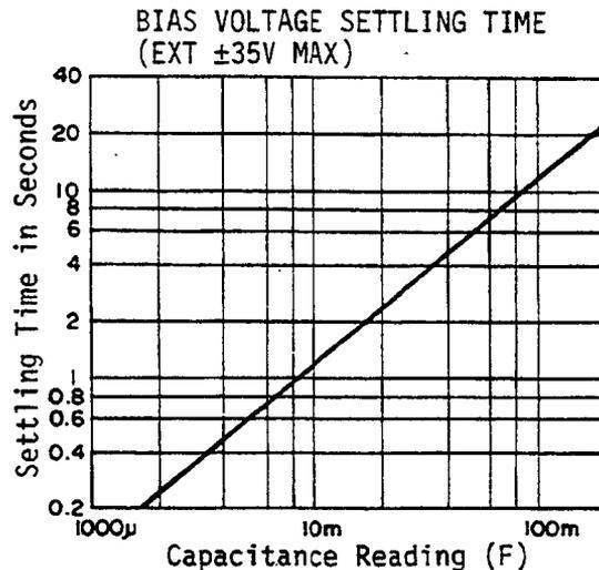
Note: EXT  $\pm$ 35V MAX and EXT  $\pm$ 200V MAX inputs feed external dc bias to sample through resistors of approximately 50 $\Omega$  and 150k $\Omega$ , respectively.
