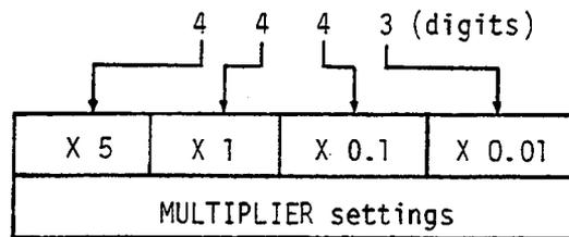
On 3 digit full scale ranges (at MULTIPLIER X 5 settings), when the measured sample value is small compared to full scale range value, the number of digits displayed is automatically increased as illustrated below:
