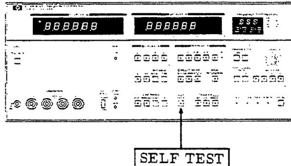
**Display Test (first step of SELF TEST):** When SELF TEST button is pushed, all front panel indicator lamps except that for the BIAS ON indicator illuminate for approximately 1 second. All segments of the numeric and character displays are also lit. This test is the initial step of the cyclic SELF TEST operation.
