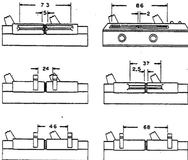
Dimensions of Test Fixture Contacts.
