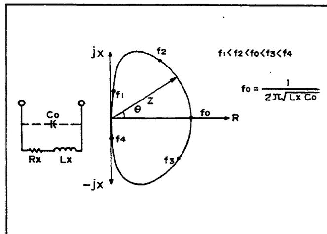
Figure 3-13. Typical Impedance Locus of an Inductor.
