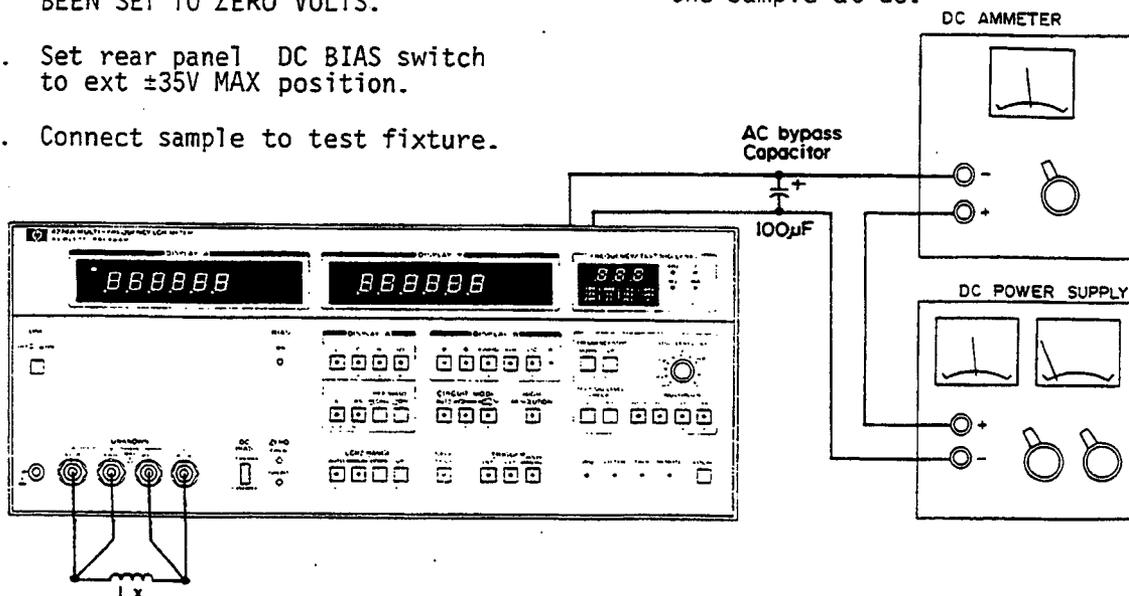
Figure 3-19. External DC Bias Circuits (sheet 4 of 4).
