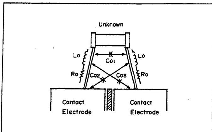
Figure 3-10. Parasitic Impedances Incident to DUT Connections.
