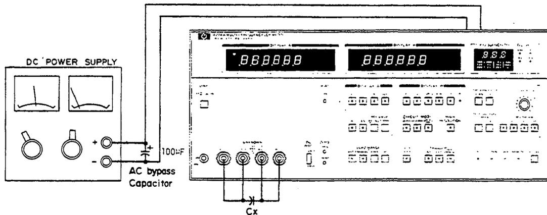
To make capacitance measurements using external dc bias voltages up to  $\pm 200V$ , connect dc bias source and test fixture as shown in diagram. If maximum applied dc bias voltage exceeds  $\pm 35V$ , use operating PROCEDURE A. If not, use PROCEDURE B to obtain a shorter bias voltage settling time.
