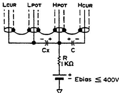
Capacitance value of the dc blocking capacitor C should satisfy the following condition:
