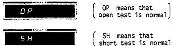
The sequential diagnostic test is repeated, and another Display Test initiated until the SELF TEST button is again pushed. If an abnormal result occurs during the open or short test, the number of the abnormal step is displayed in DISPLAY A as, for example, illustrated below:
