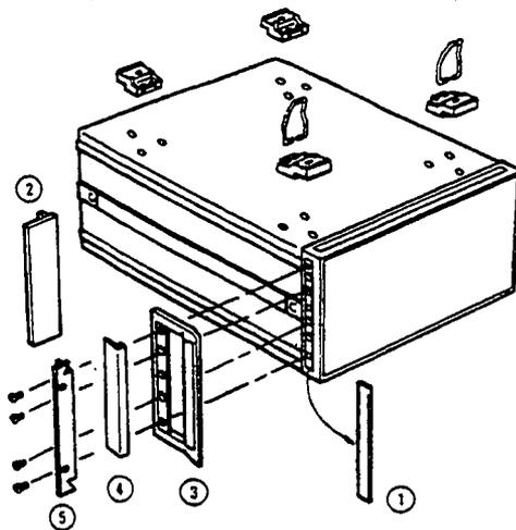
1. Remove adhesive-backed trim strips ① from side at right and left front of instrument.
