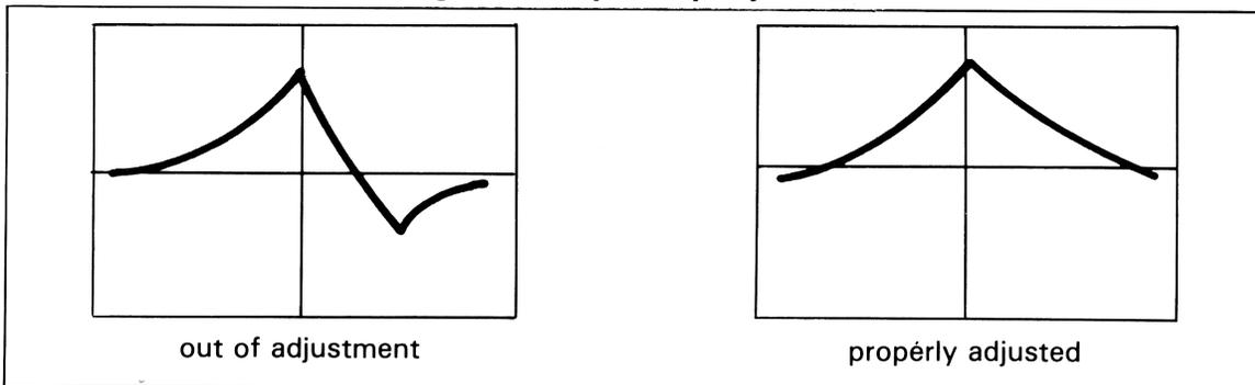
**Figure 7-4. Symmetry Adjustment**
