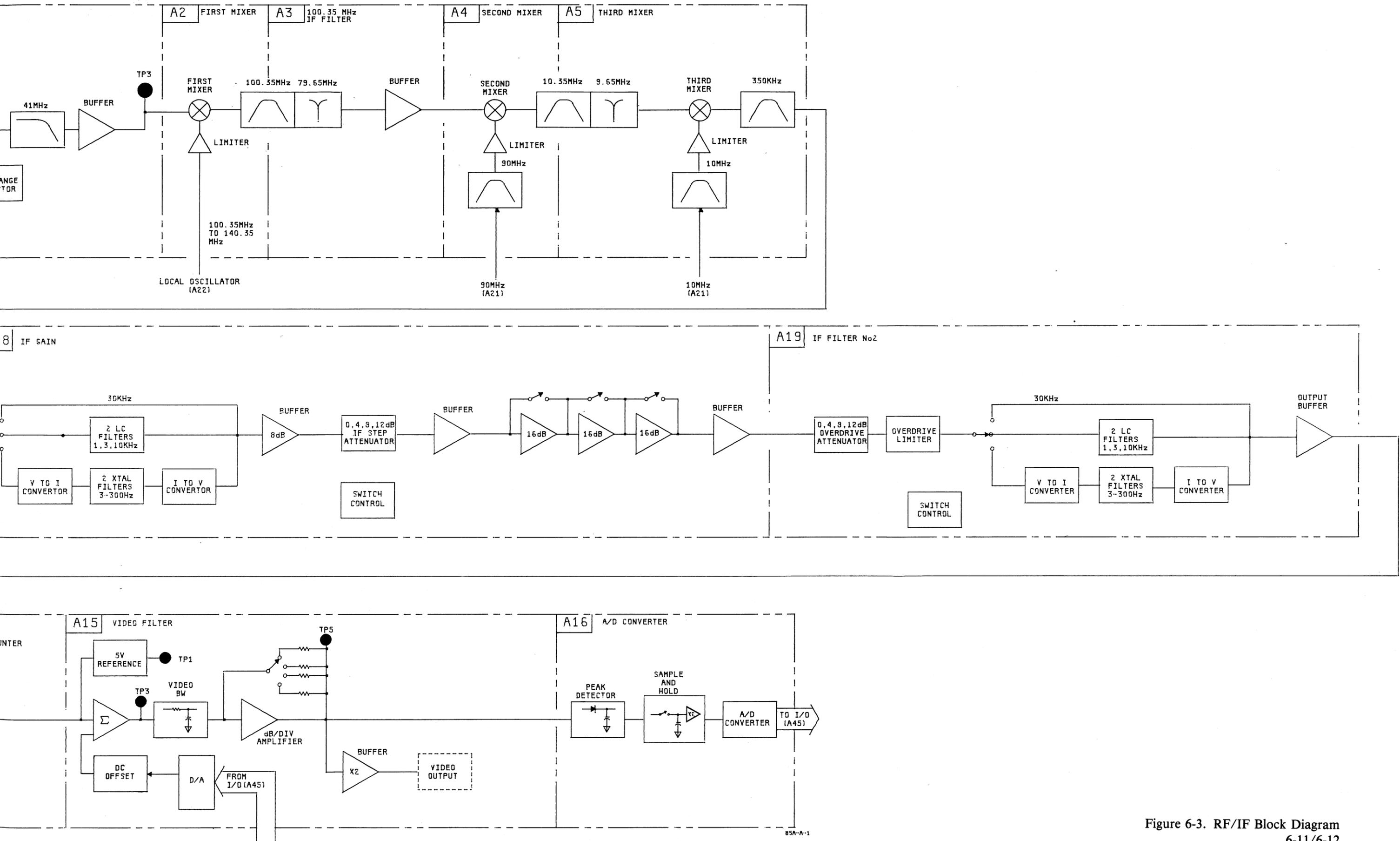
Figure 6-3. RF/IF Block Diagram
