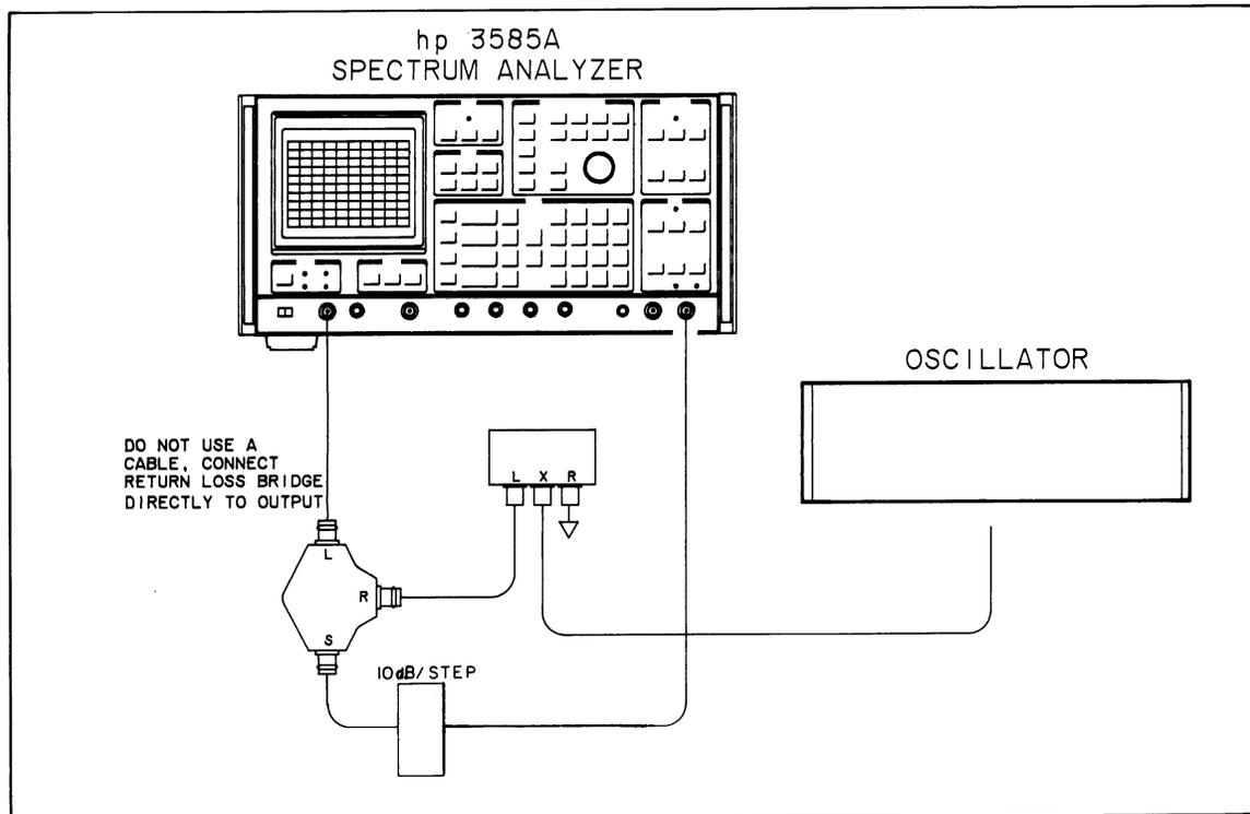
**Figure 4-15. Tracking Generator Return Loss Test (Automatic Tests)**
