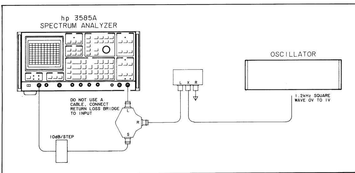
Figure 4-13. 50 ohm Return Loss Test (Automatic Tests)
