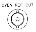
The OVEN REF OUT supplies a  $10 \text{ MHz} \pm 1 \times 10^{-7}$  per month sinusoidal frequency reference from an internal crystal oscillator, located in a temperature-controlled oven. The output is ac coupled and the output impedance is 50 ohms. The nominal output level is +10 dBm/50 ohms. The output is disabled during the oven's warm-up cycle. To use the internal Oven Reference, this output must be connected to the EXT REF IN jack.
