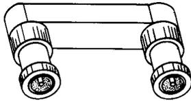
To use the internal Oven Reference, connect this BNC-to-BNC jumper between the OVEN REF OUT connector and the EXTERNAL REF IN connector.
