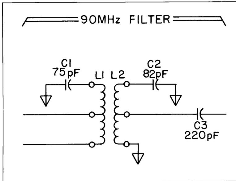
Drawing 7-1. Δ1 90MHz Filter, p/o Schematic A-2
