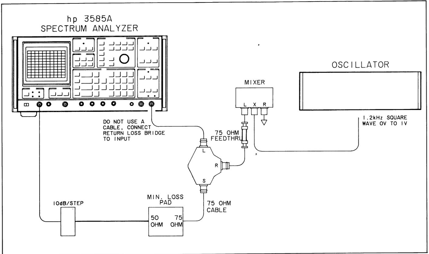
**Figure 4-14. 75 ohm Return Loss Test (Automatic Tests)**
