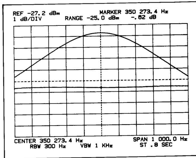
Figure 5-29. Correctly Adjusted IF Stage, A-B Mode
