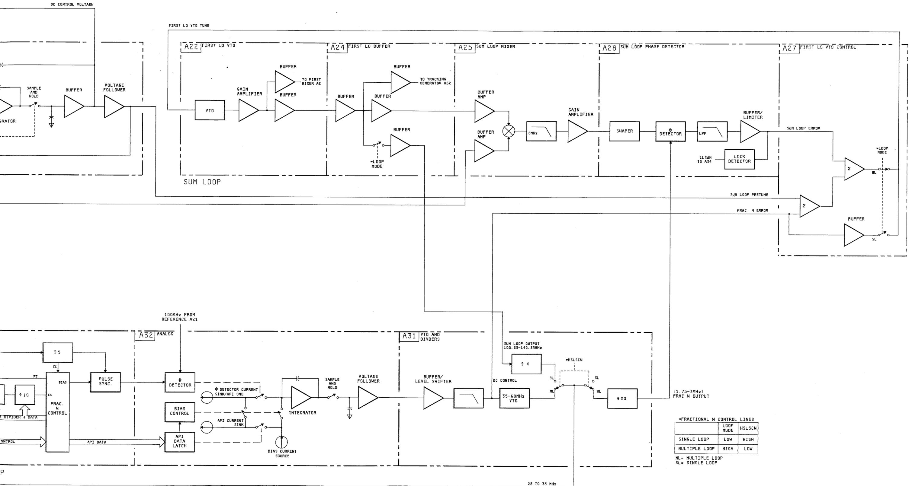
Figure 6-12. Local Oscillator Block Diagram
