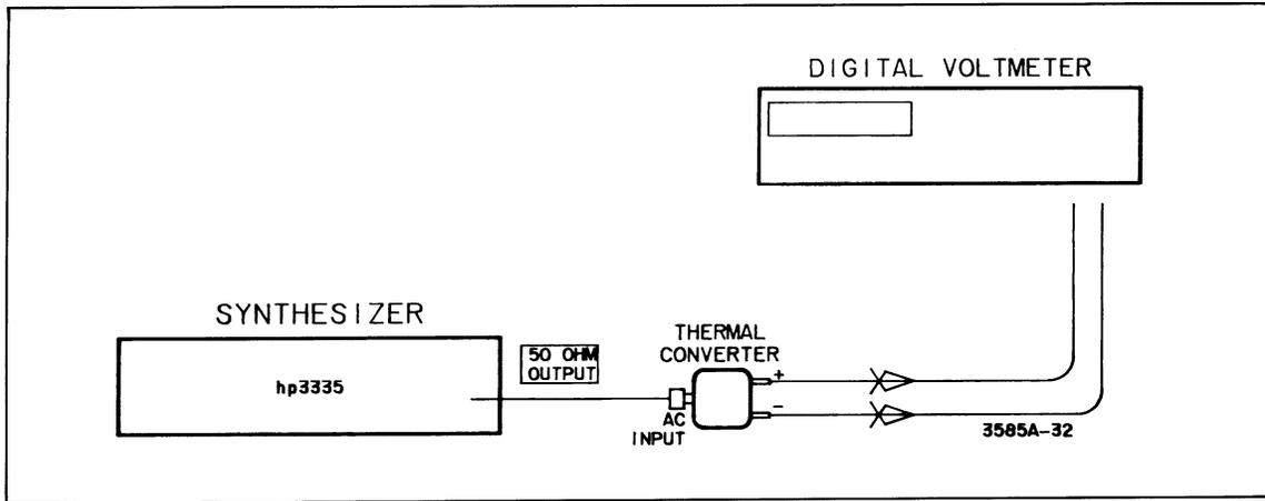
Figure 4-12. Measurement of Frequency Synthesizer For Calibration Data
