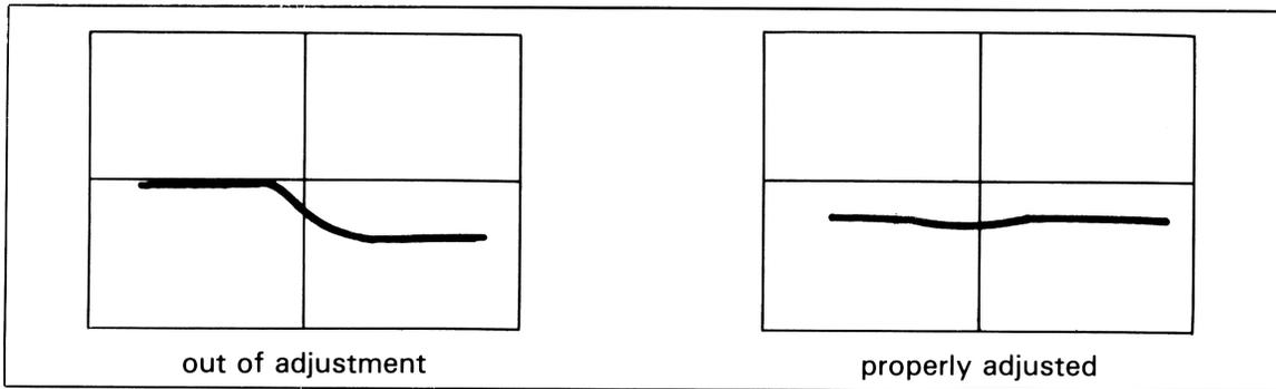
**Figure 7-3. Symmetry Adjustment**
