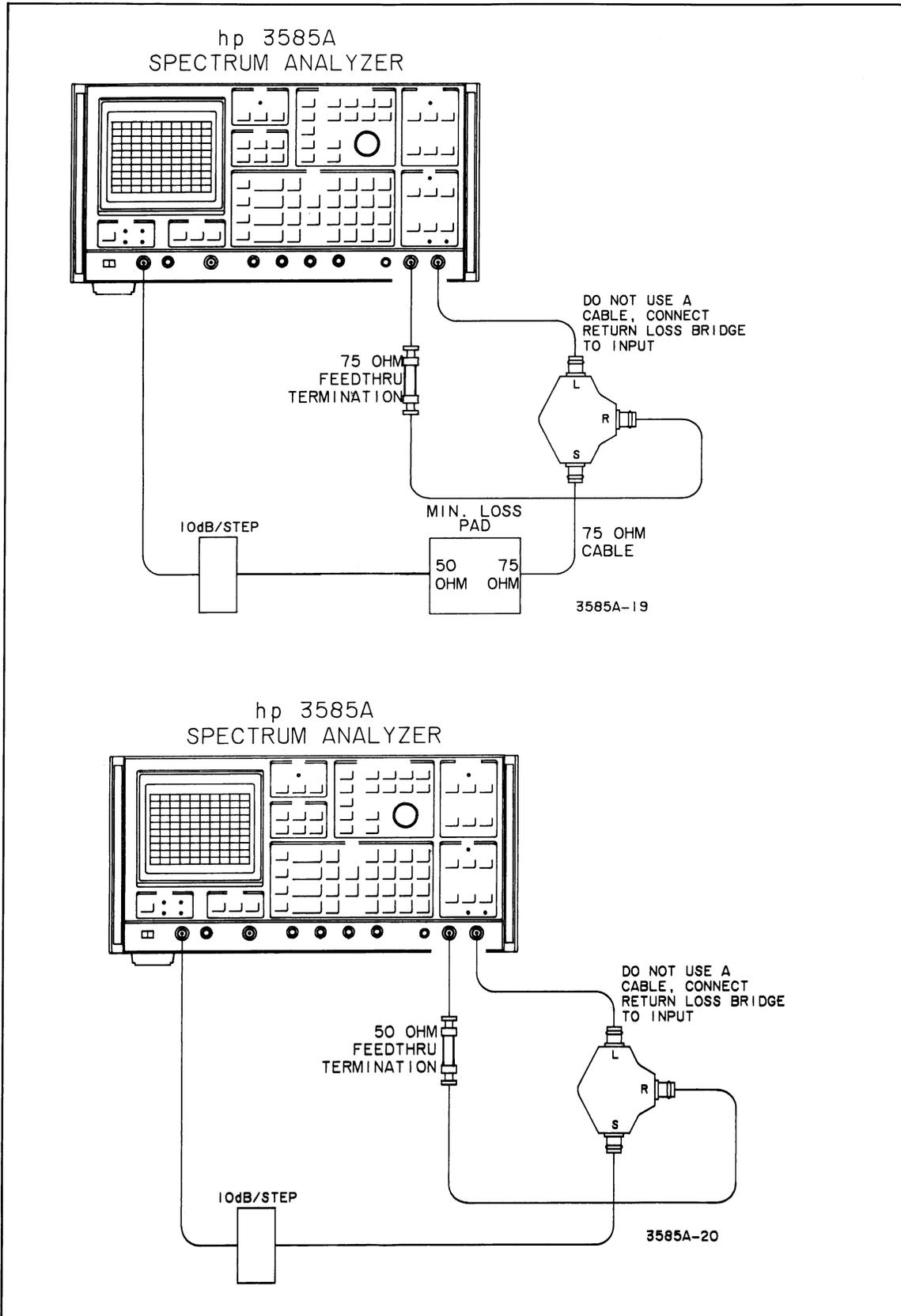
Figure 4-16. Terminated Input Return Loss Test (Automatic Tests)
