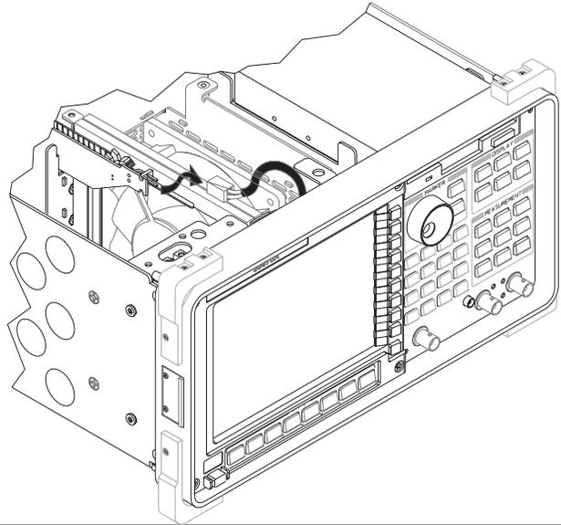
**3** Remove assembly retainer bracket.
