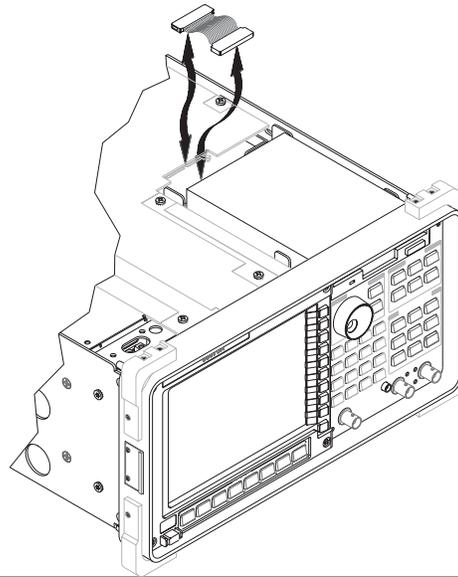
**3** Using a T-10 torx driver, loosen the three screws at the back of the disk drive bracket.
