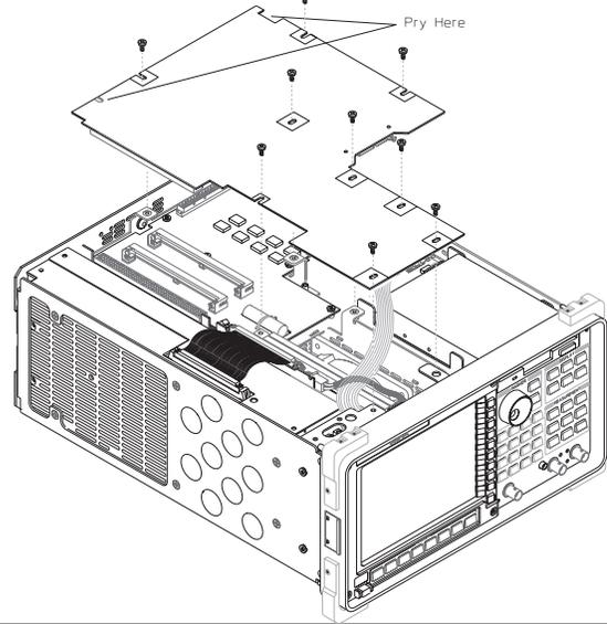
**3** Disconnect the ribbon cables from the A7 CPU assembly.
