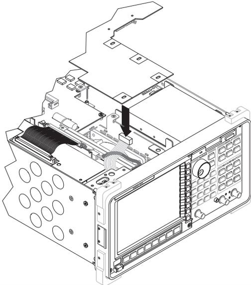
**4** The analyzer's serial number and firmware options are stored in EEPROM (U27) on the A7 CPU assembly. Before replacing the CPU assembly, remove A7 U27 from the faulty assembly and insert into the new assembly. See "What to do before replacing the CPU assembly" on page 6-3.
