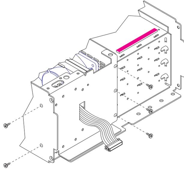
**3** Using a T-10 torx driver, remove the four screws from the shield. Unplug ribbon cables.
