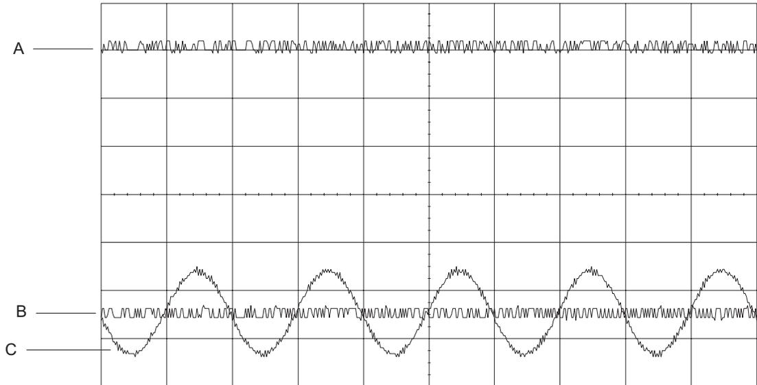
R431 and R405 Correctly Adjusted
