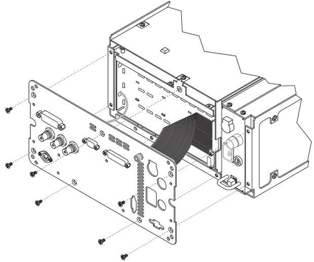
**3** Disconnect the ribbon cable and the coaxial cable from the A10 Rear Panel assembly.
