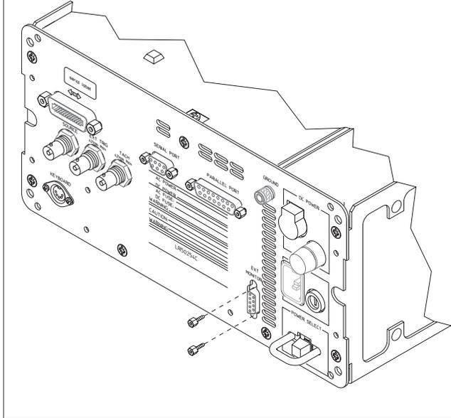
**6** Using T-10 torx driver, remove the twelve screws in A99 Motherboard.
