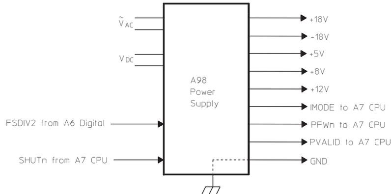
A98 Power Supply Block Diagram
