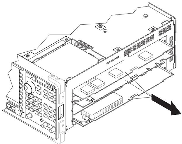
**5** Using a 5 mm open-ended wrench, remove the two screws from the EXT MONITOR connector.
