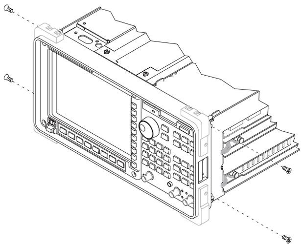
**5** Pull the top of the front panel out of the frame.
