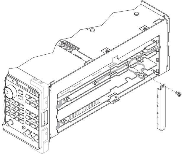
**3** Slide A5 Analog assembly part way out and disconnect gray mic cable.
