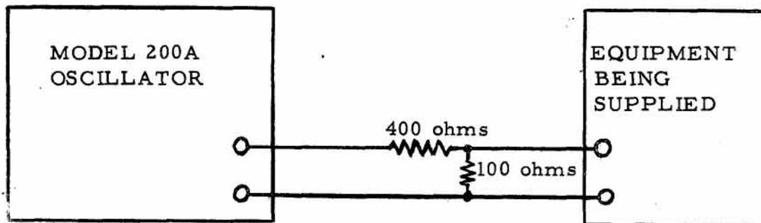
Other values of resistance may be used to obtain different voltage divisions. In all cases, the sum of the divider resistors must equal the rated load of 500 ohms.
