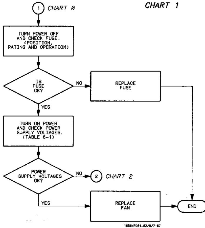
Figure 6-4. Trouble Isolation Chart for HP 1650A/51A Fan/Fuse
