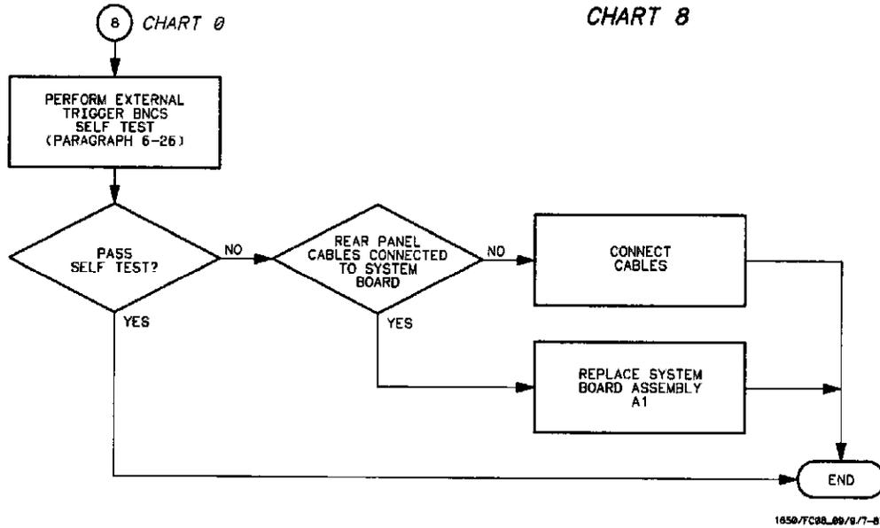
Figure 6-11. Trouble Isolation Flowchart for HP 1650A/51A Trigger BNCs
