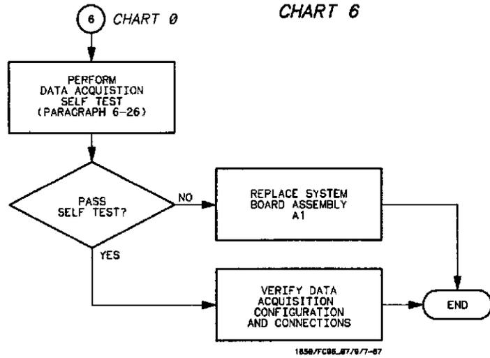
Figure 6-9. Trouble Isolation Flowchart for HP 1650A/51A Data Acquisition
