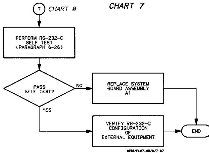
Figure 6-10. Trouble Isolation Flowchart for HP 1650A/51A RS-232-C
