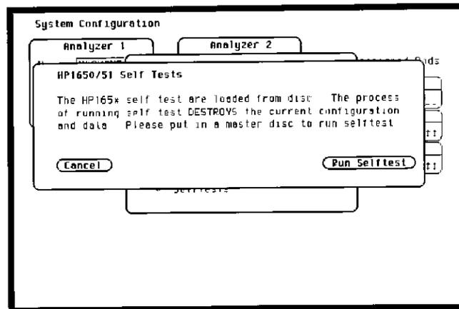
Figure 6-16. HP 1650A/51A Self Tests Pop-up Menu
