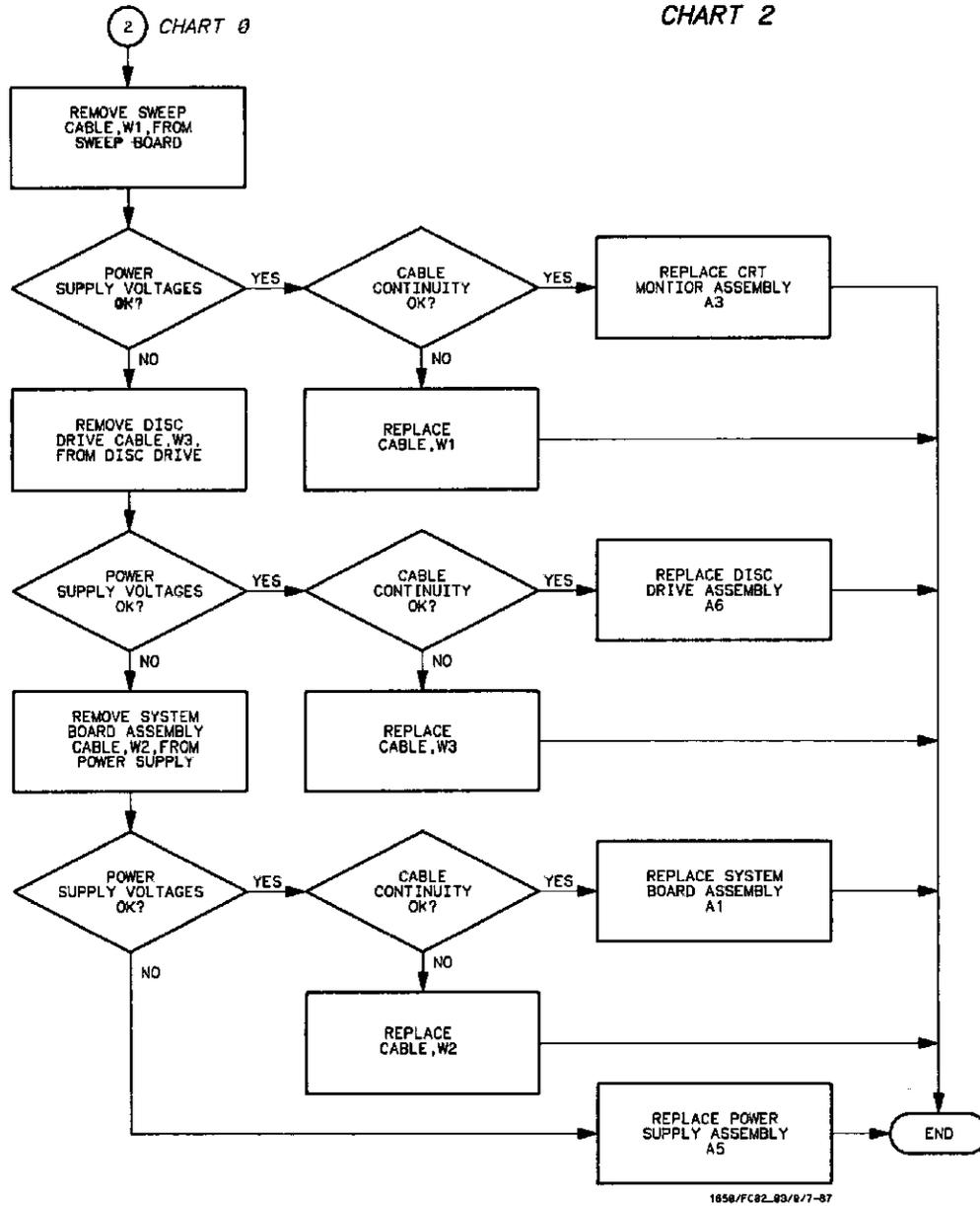
Figure 6-5. Trouble Isolation Flowchart for HP 1650A/51A Power Supply
