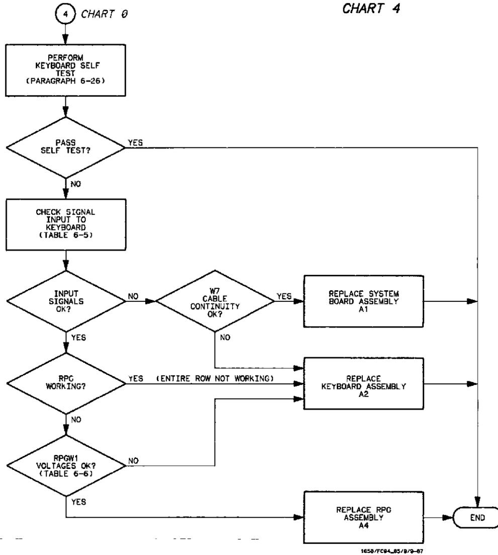
Figure 6-7. Trouble Isolation Flowchart for HP 1650A/51A Keyboard
