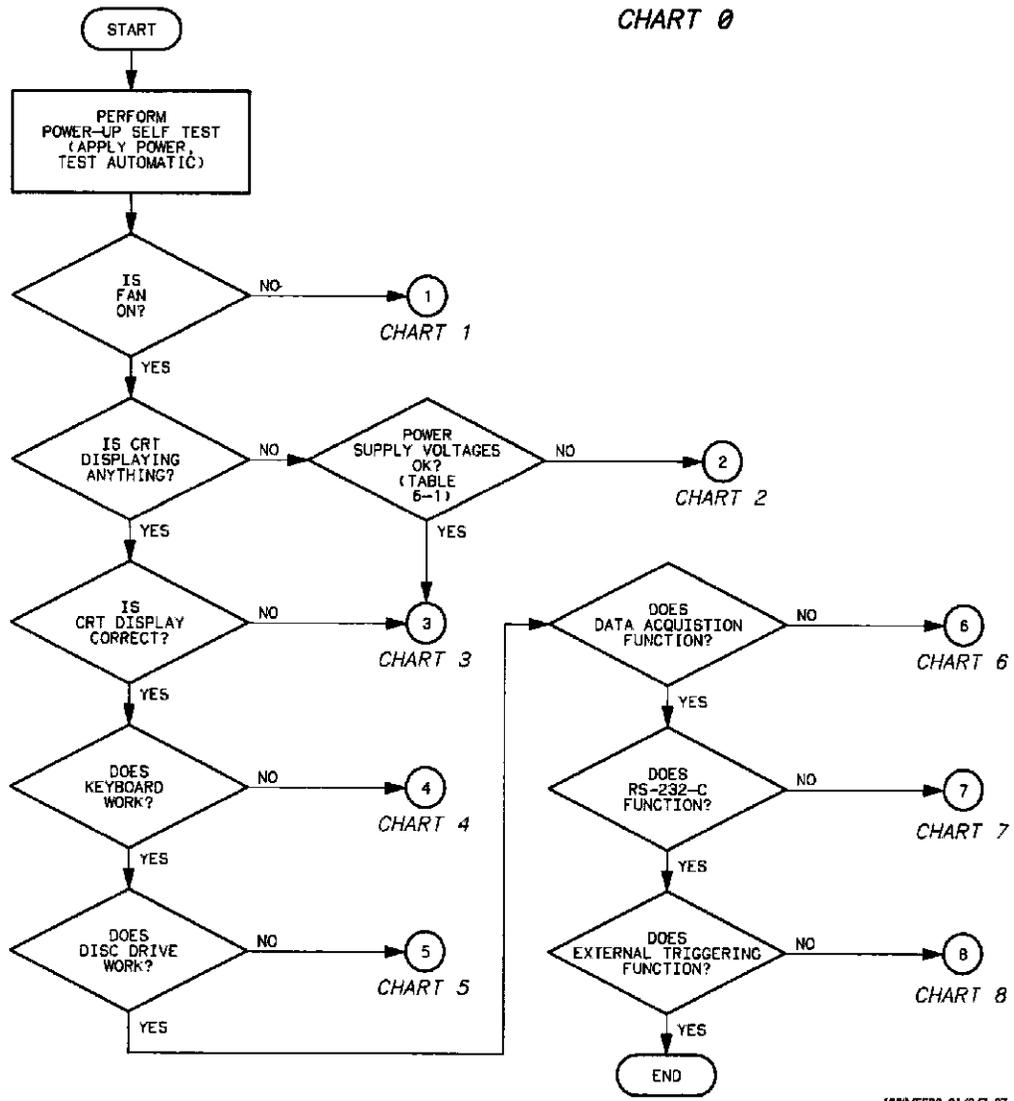
Figure 6-3. General Trouble Isolation Flowchart for HP 1650A/51A
