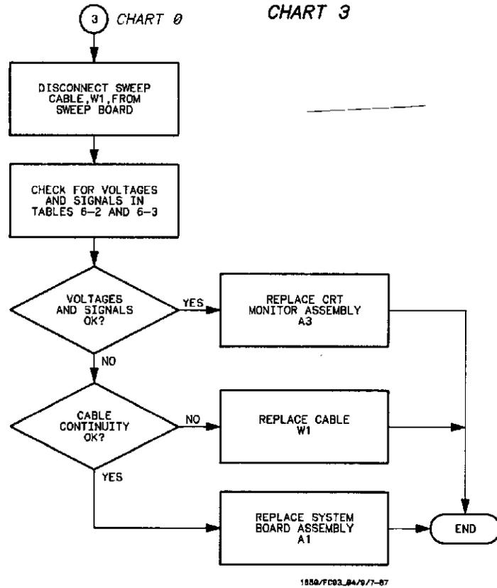
e 6-6. Trouble Isolation Flowchart for HP 1650A/51A CRT Monitor
