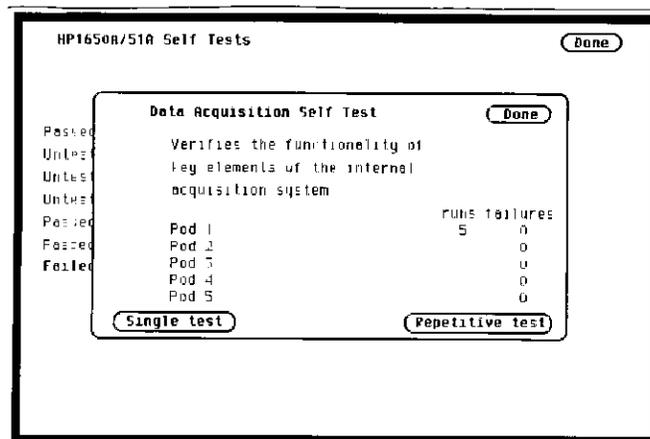
Figure 6-19. Runs and Failures of Repetitive Data Acquisition Self Test
