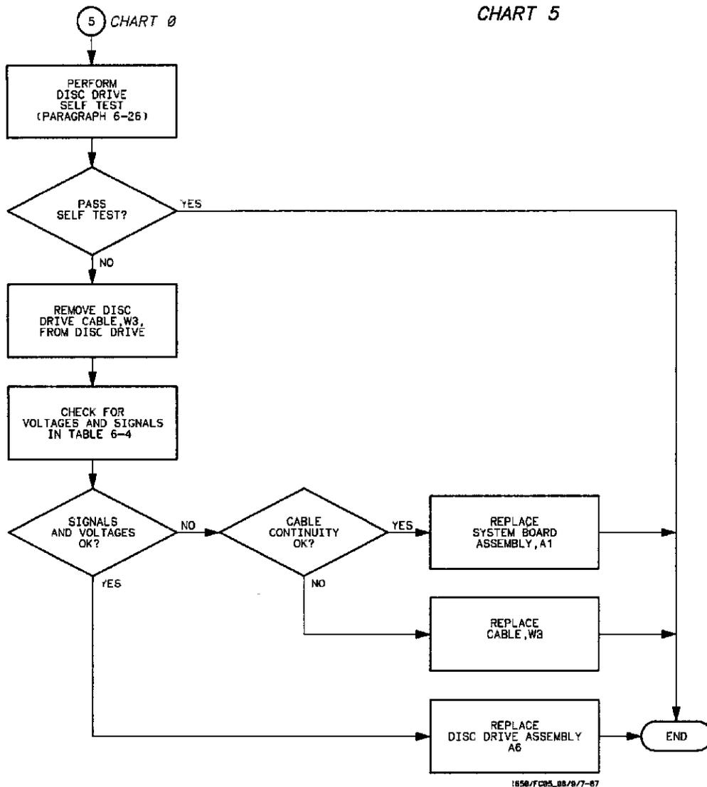
Figure 6-8. Trouble Isolation Flowchart for HP 1650A/51A Disc Drive
