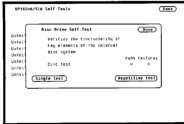
Figure 6-27. Disc Drive Self Test Pop-up Menu
