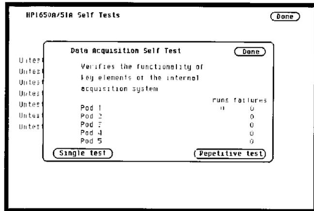
Figure 6-18. Data Acquisition Self Test Pop-up Menu
