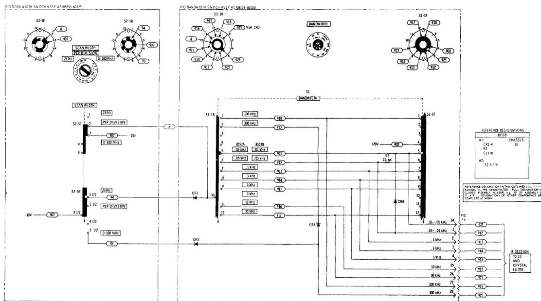
Figure 8-48. Bandwidth Control Circuits for IF Section.
