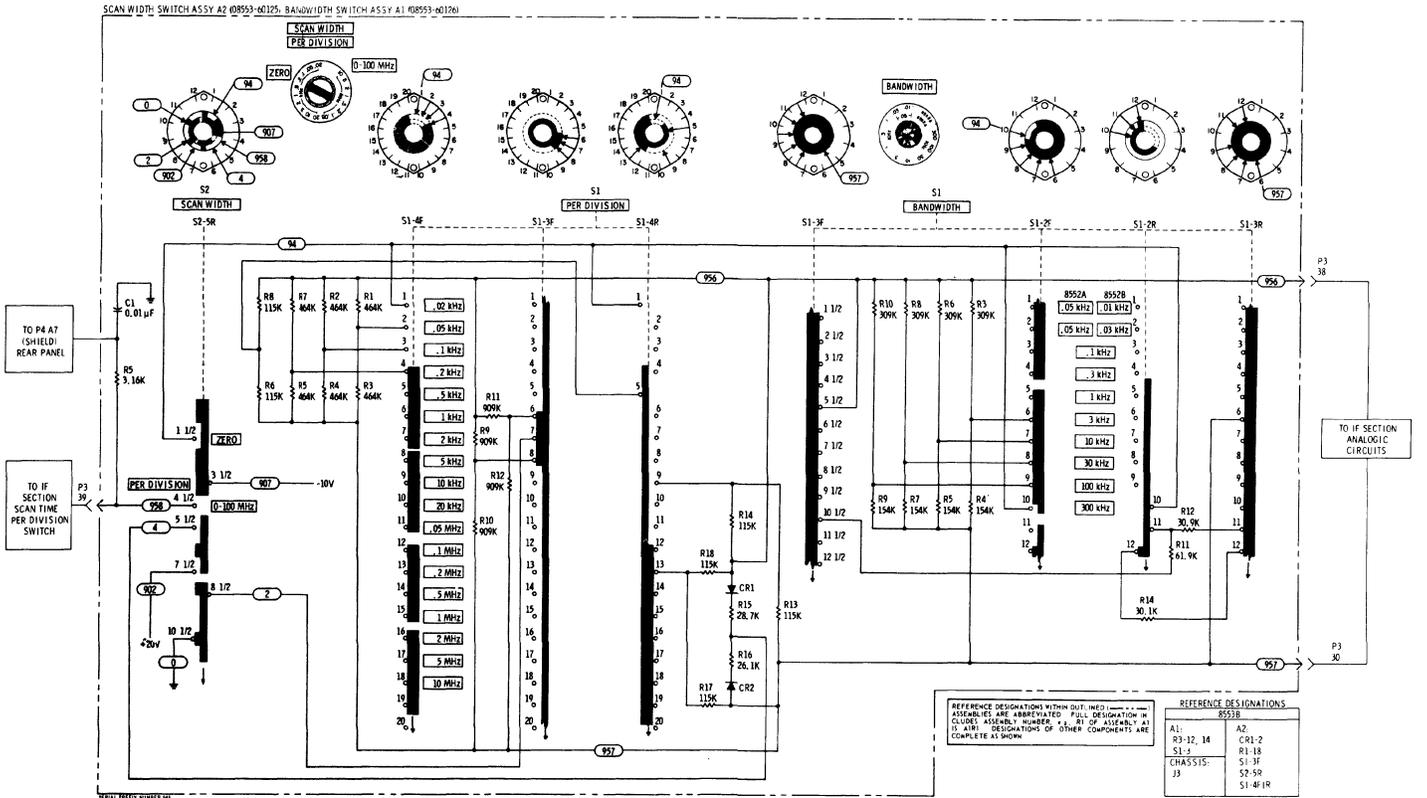
Figure 8-50. Analog Switching Matrix
