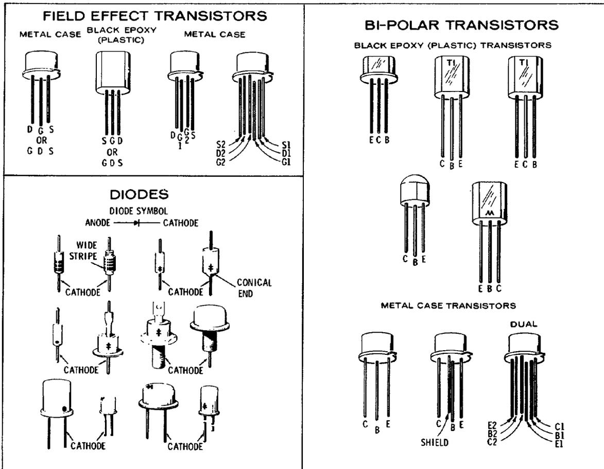
Figure 8-4. Examples of Diode and Transistor Marking Methods.
