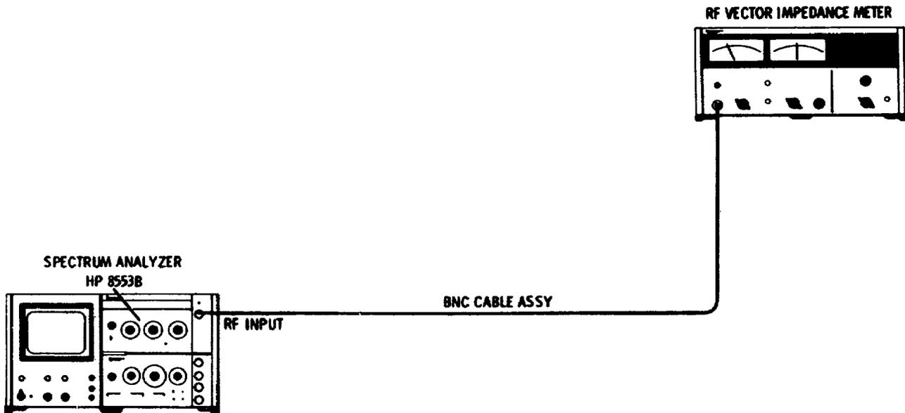
Figure 4-3. Input Impedance Accuracy Test: 500 kHz to 110 MHz
