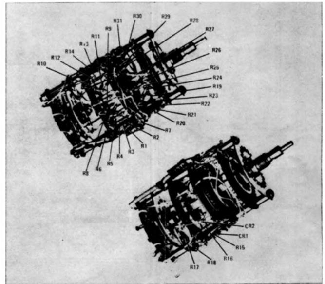
Figure 8-21. Scan Width Attenuator Assembly A2 (08553-60125)
