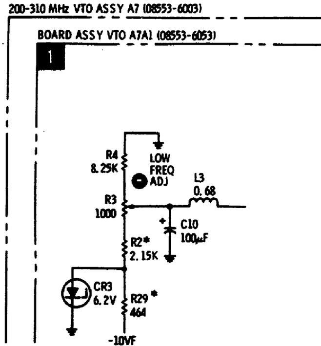
P/O Figure 8-33. 200-310 MHz Voltage-Tuned Oscillator (P/O CHANGE 8).
