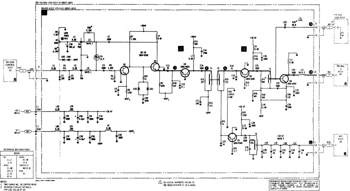
Figure 8-33. 200-301 MHz Voltage Tuned Oscillator (ERRATA)
