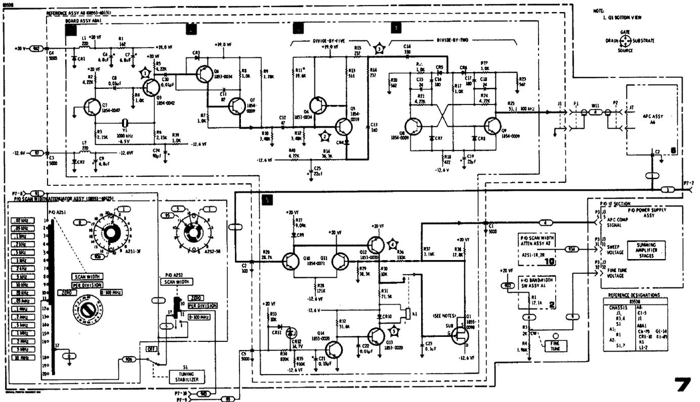
Figure 6. 1 MHz Crystal Oscillator, Frequency Divider and APC Compensation Circuits, Schematic Diagram (replacement for Service Sheet 7 in 8538B Operating and Service Manual)
