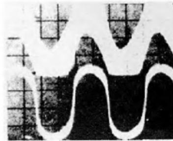
Waveform GOOD and verification procedure below also satisfactory, assembly is functioning properly.
