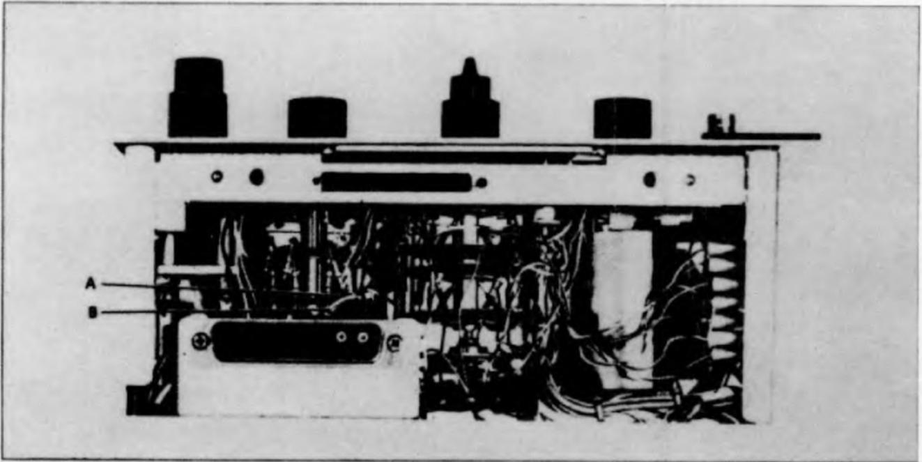
Figure 8-49. Bandwidth Switch A1 (08553-60126) Test Points
