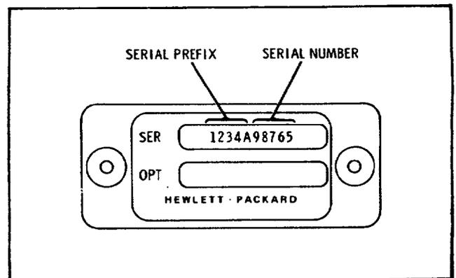
Figure 1-2. Instrument Identification
