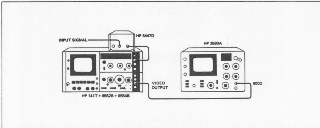
**Figure 16.** Set up for amplitude modulation measurements. HP 8447D Preamplifier, gain 26 dB, frequency range 100 kHz to 1.3 GHz; noise figure of 8.5 dB. HP Spectrum Analyzer 141T, 8552B, 8554B (100 kHz to 1250 MHz) HP Low Frequency Spectrum Analyzer 3580A (5 Hz to 50 kHz, Resolution: 1 Hz).
